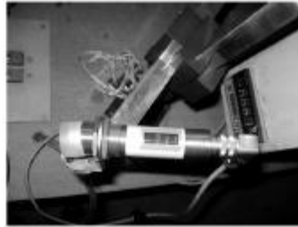
Figure 8: Infrared Pyrometer (A non Contact Temperature Measurement Device in the Range of 0-1000°C)
