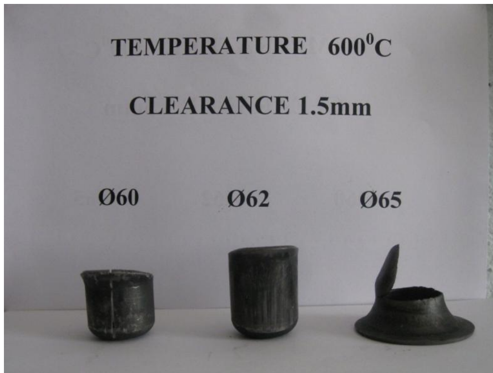
Fig.9.5 Cups with 25% thickness reduction and at 600°C
