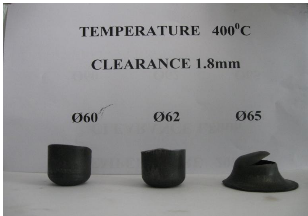
Fig. 9.7 Cups with 10% thickness reduction and at 400°C
