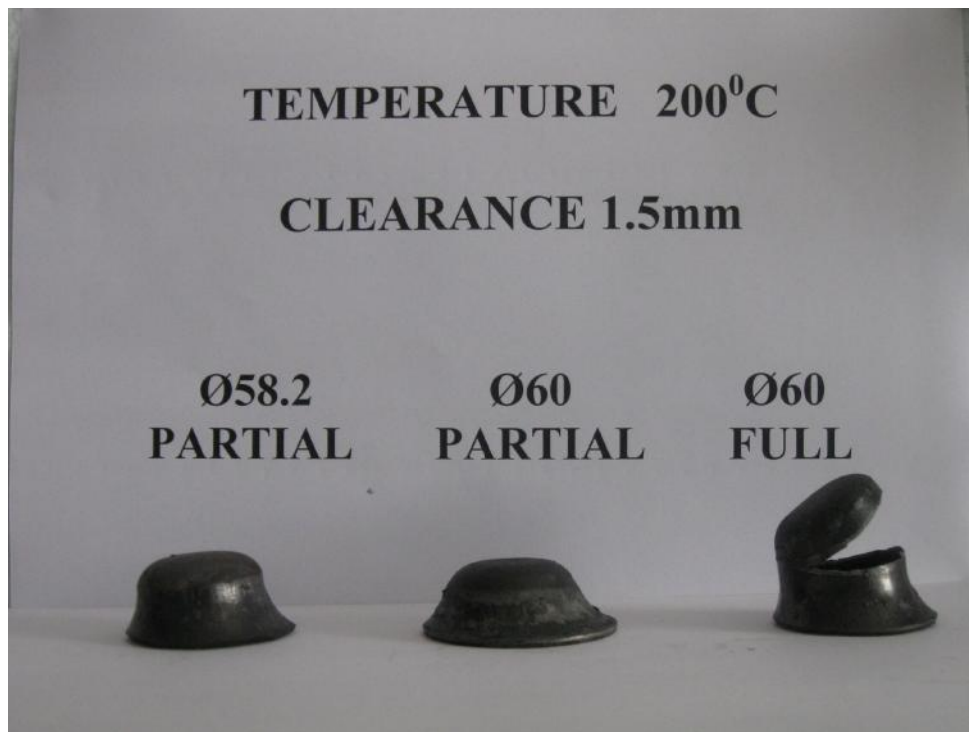
Fig. 9.3 Cups with 25% thickness reduction and at 200°C
