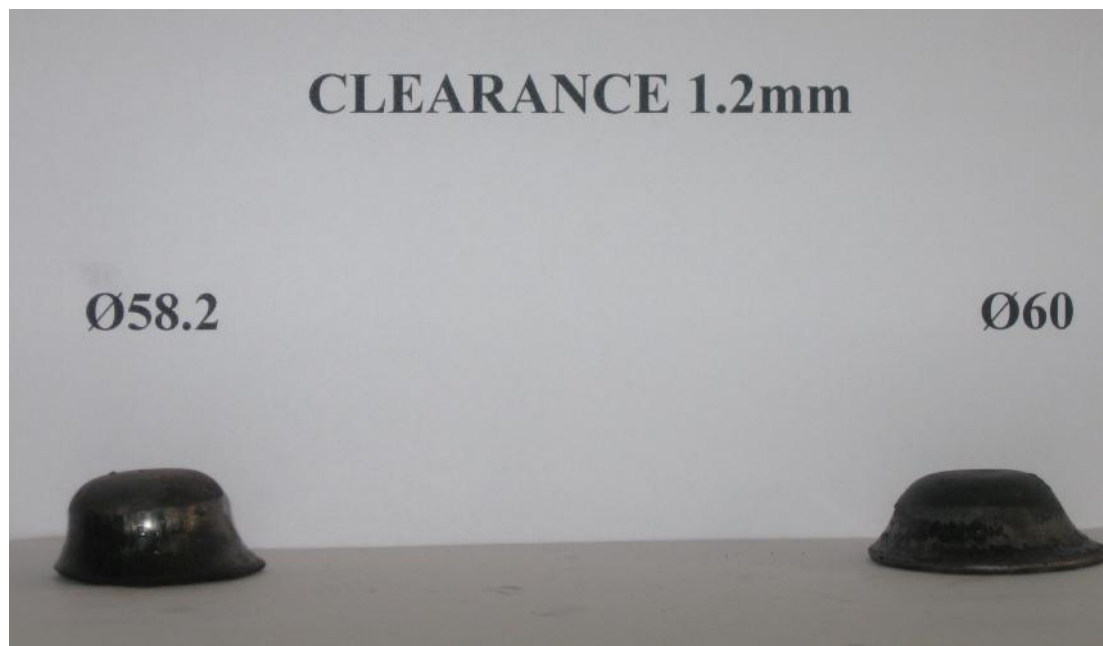
Fig. 9.1 Cups at 40% reduction at 600°C
