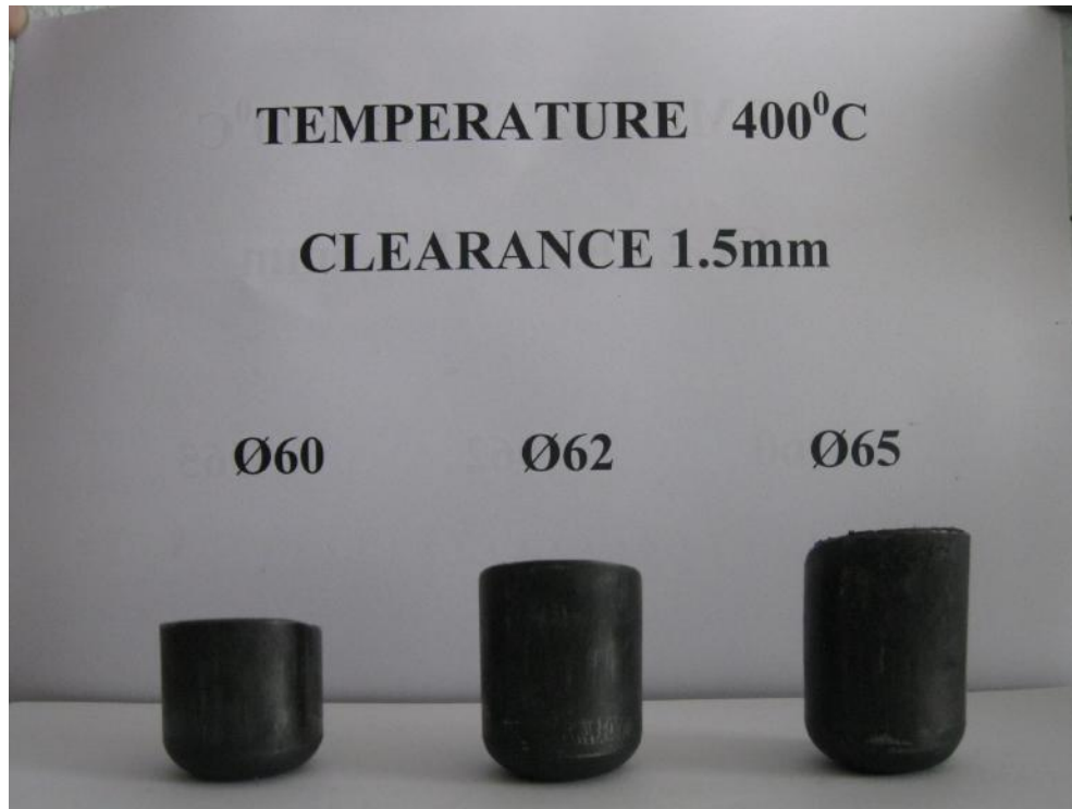
Fig. 9.4 Cups with 25% thickness reduction and at 400°C
