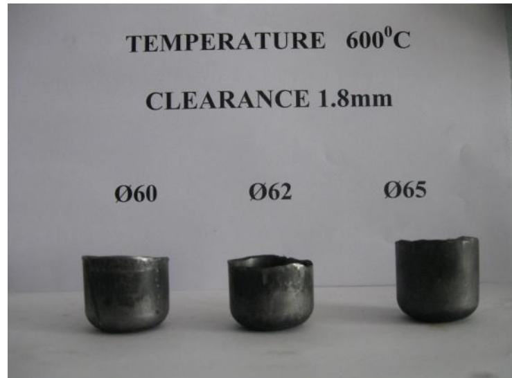
Fig. 9.8 Cups with 10% thickness reduction and at 600°C
