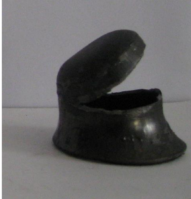
Fig.9.2 Fracture at 40% reduction
