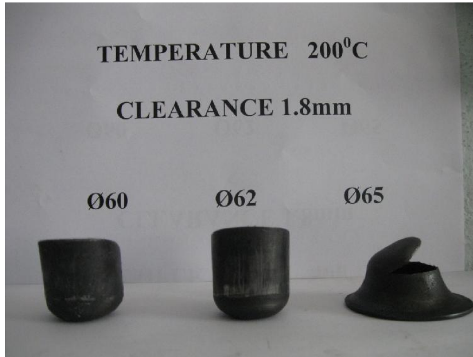
Fig. 9.6 Cups with 10% thickness reduction and at 200°C
