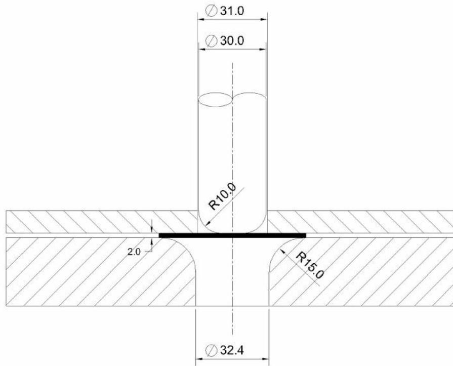
Fig.4.4 Tooling for 40% reduction in the thickness of 2 mm sheet.
