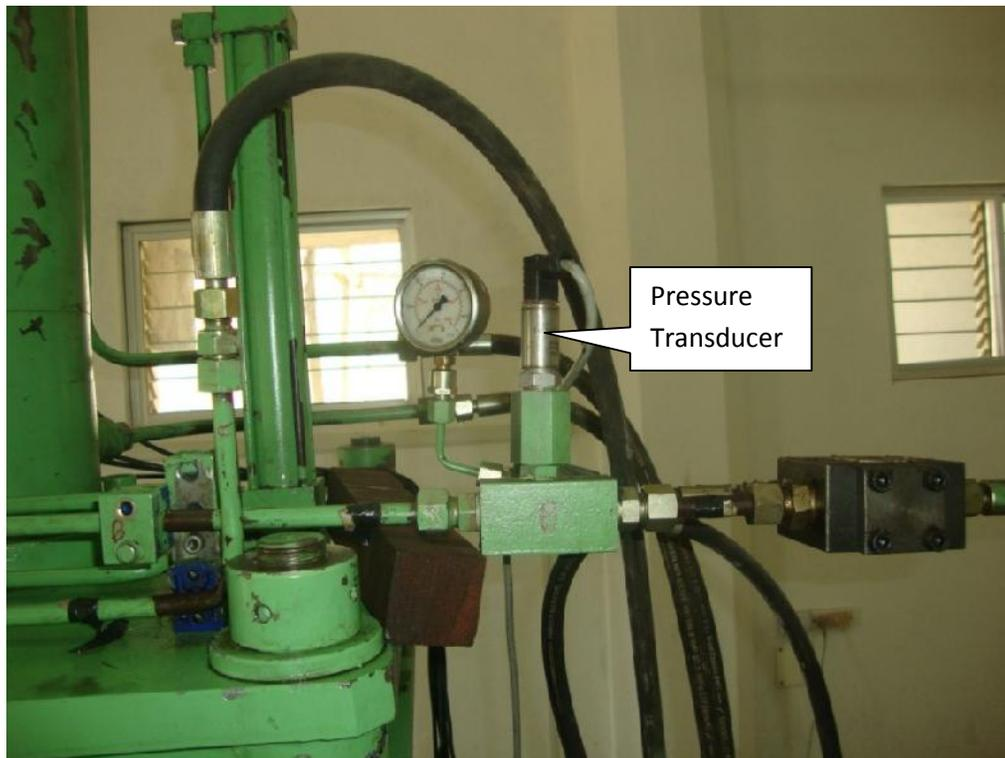
Fig 4.11. Pressure Transducer to measure Blank holding Pressure
