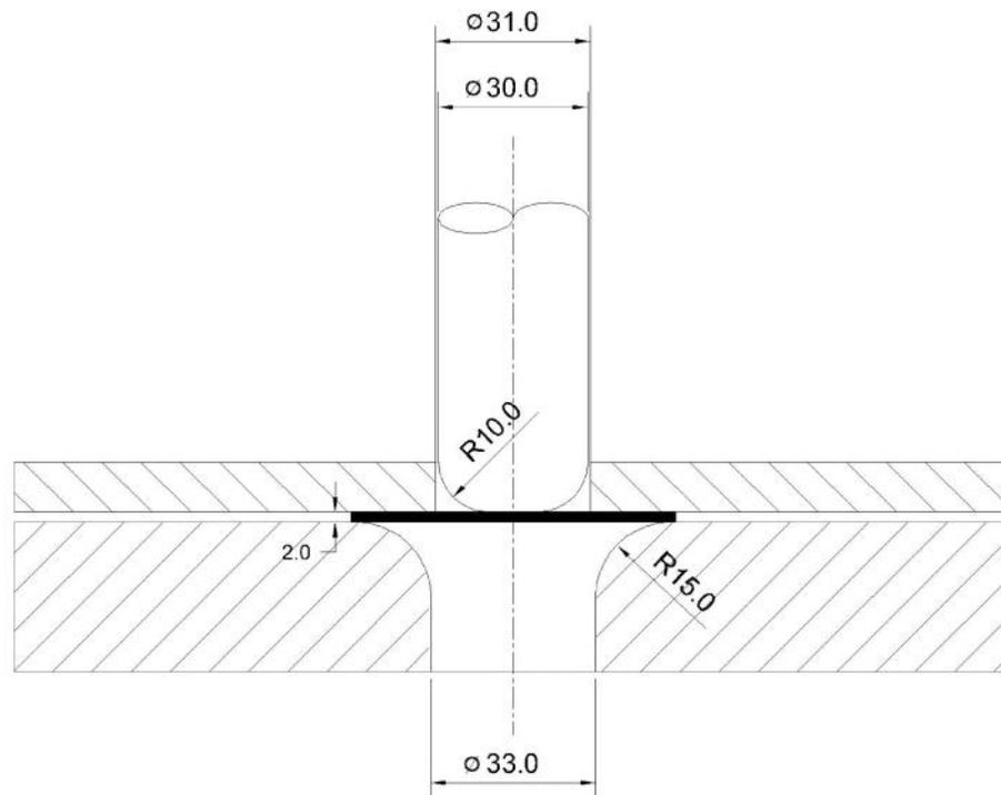
Fig. 4.3 Tooling for 25% reduction in the thickness of 2 mm sheet.
