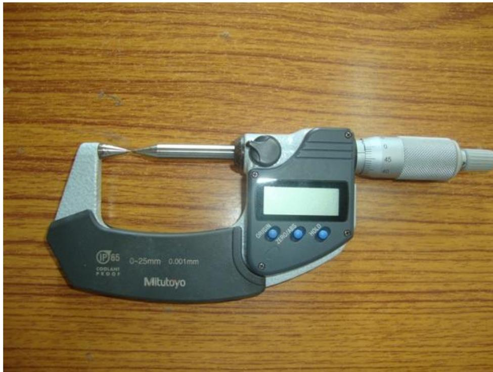
Fig 4.18 Pointed Anvil Micrometer
