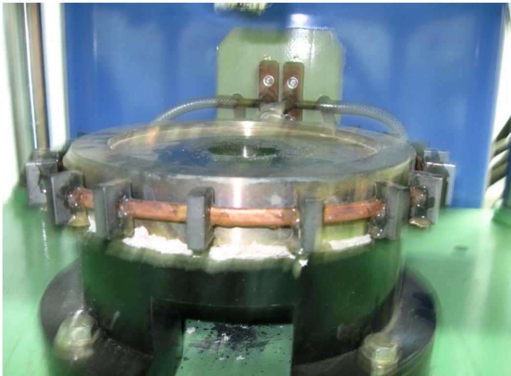
Fig. 4.8 Induction coil connected to the Inconel die for heating it up to 500°C.
