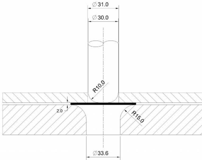
Fig.4.2 Tooling for 10% reduction in the thickness of 2 mm sheet.
