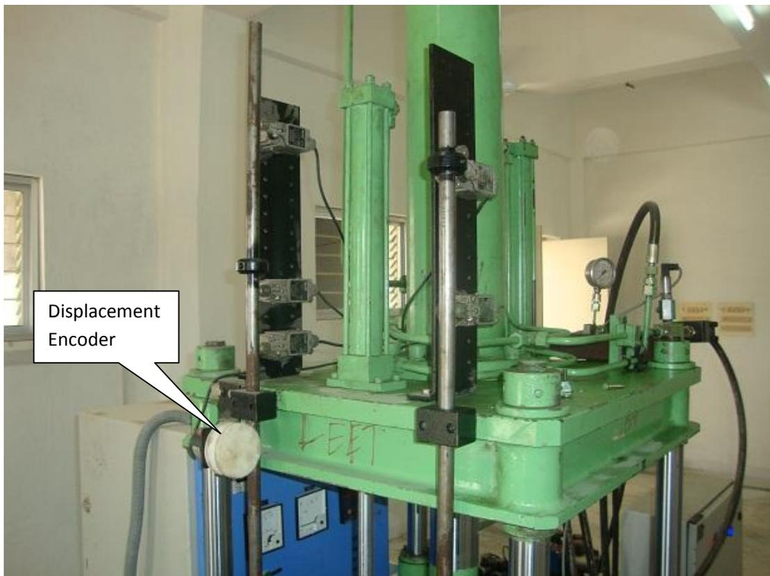
Fig 4.12. Encoder for Punch movement data acquisition
