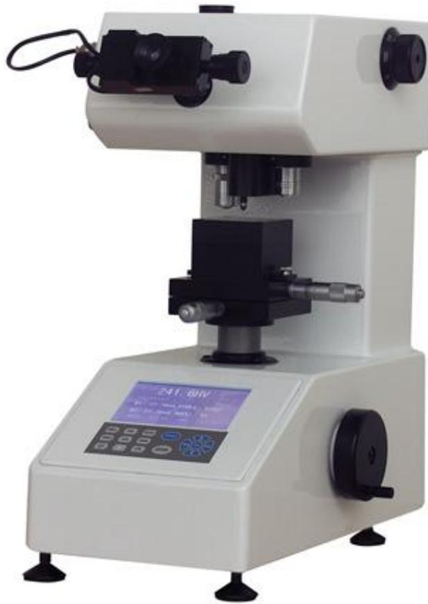
Fig 4.17 Micro Hardness Tester
