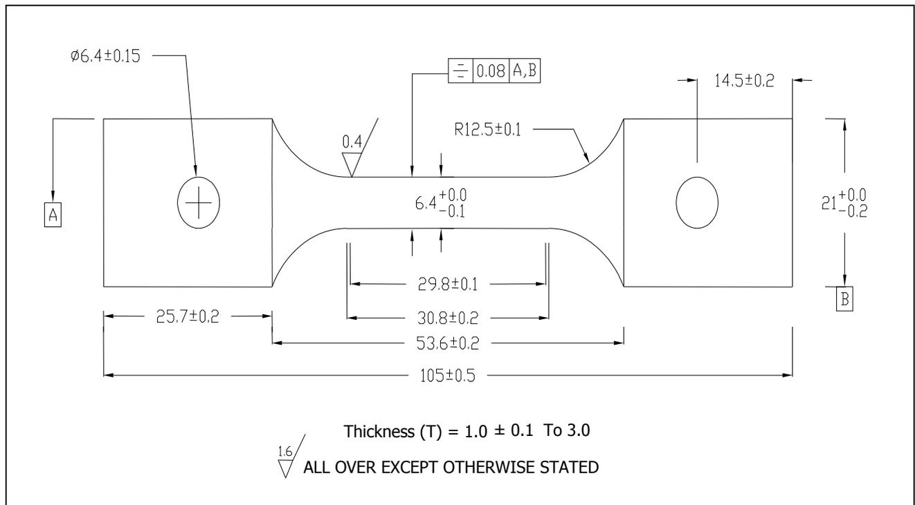
Fig 4.19 Specimen Drawing for Tensile test (DMRL practice)[77]
