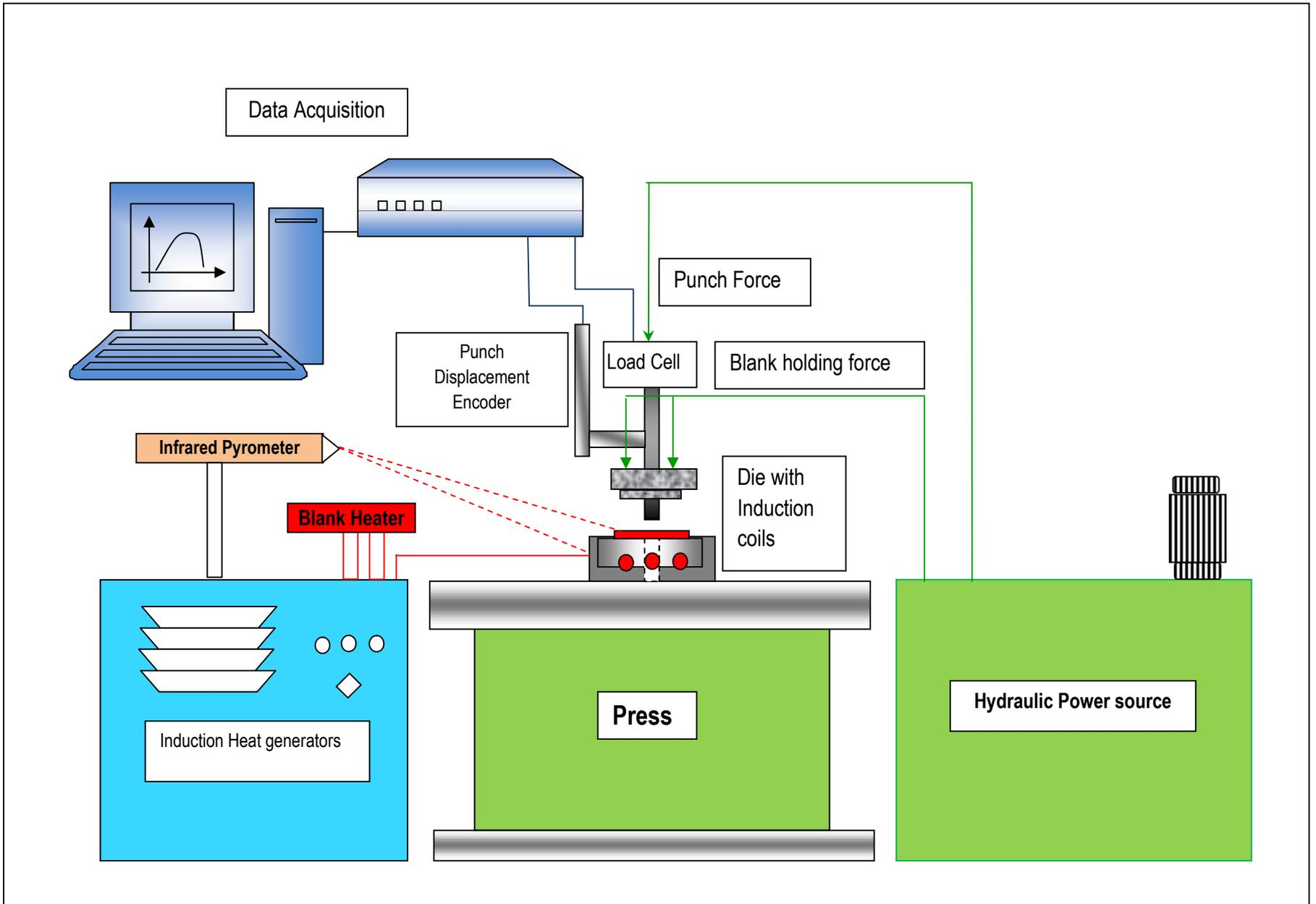
Fig 4.1 Schematic of Experimental setup for warm flow forming
