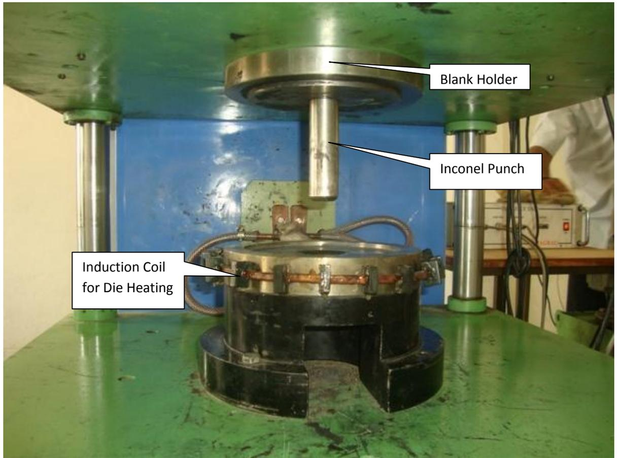
Fig 4.6 Punch Die and Blank Holder Setup
