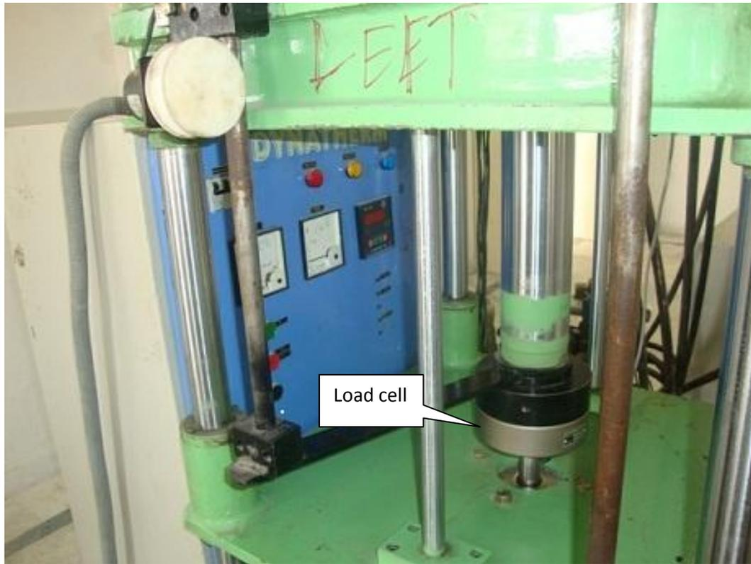
Fig 4.10 Load cell of the Data Acquisition System
