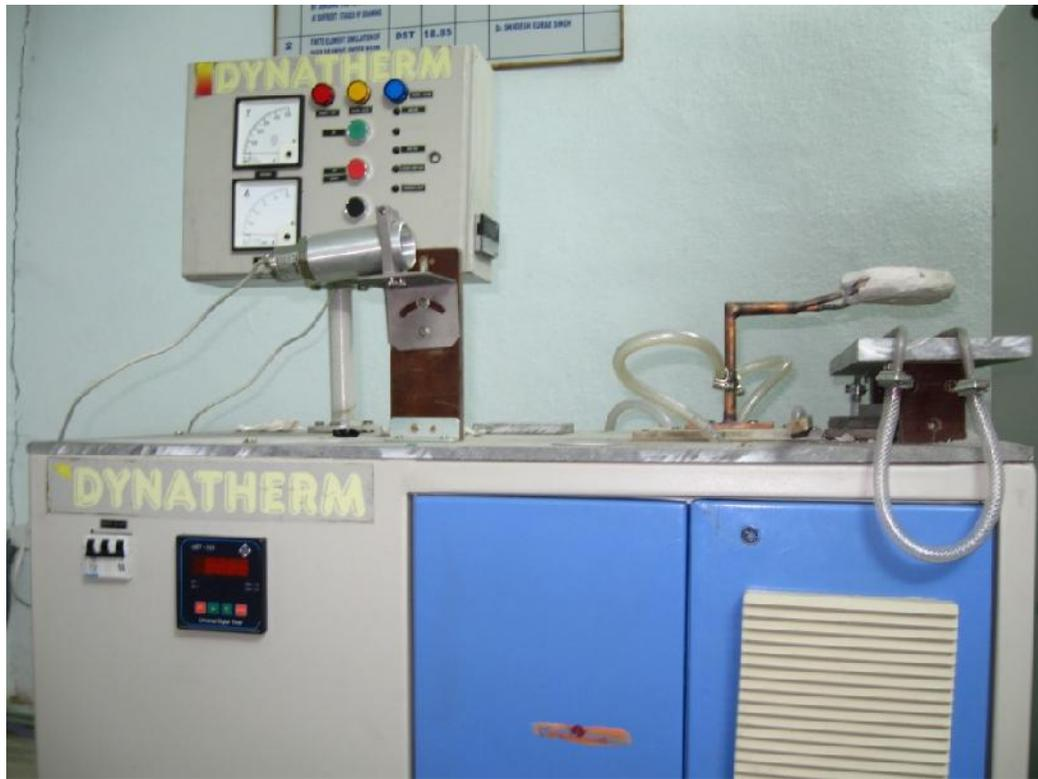
Fig. 4.7: Induction furnace used for heating the blank.
