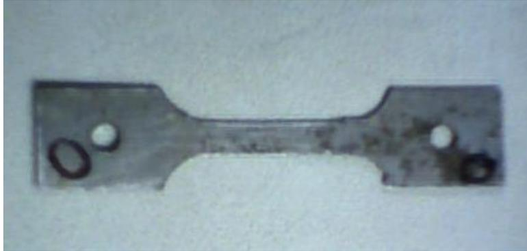
Fig 4.20 Specimen prepared according to Drawing for Tensile test
