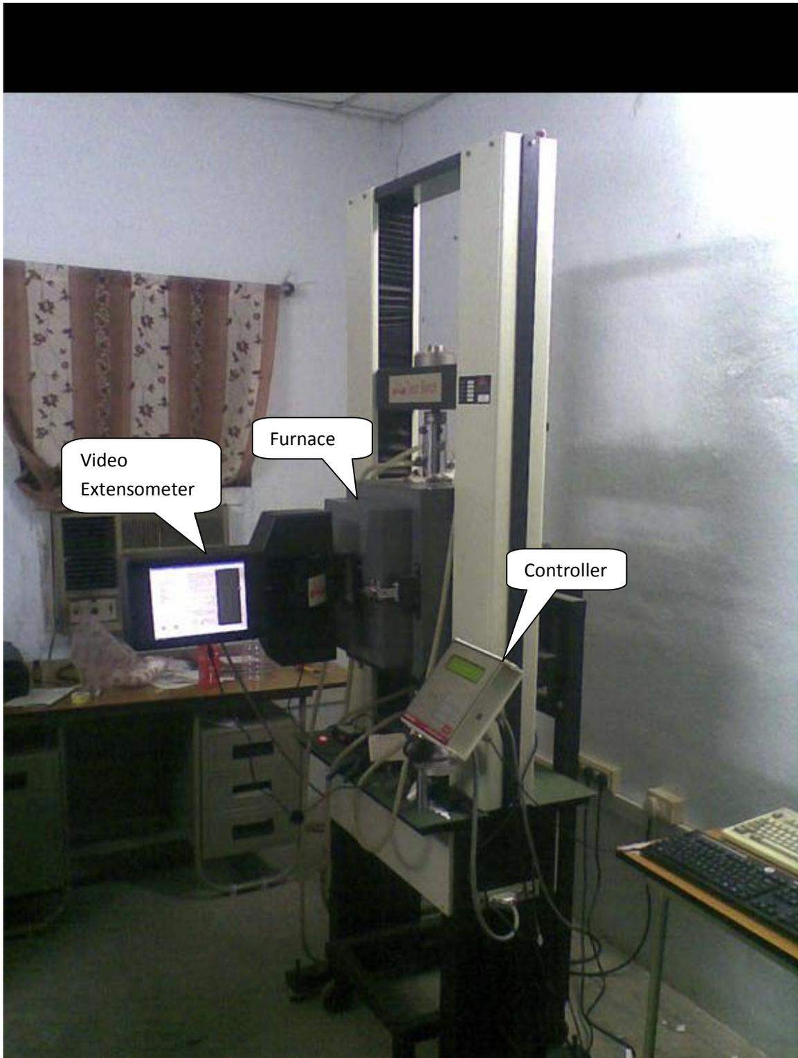
Fig 4.14 A 50 kN Electronically Controlled UTM with furnace
