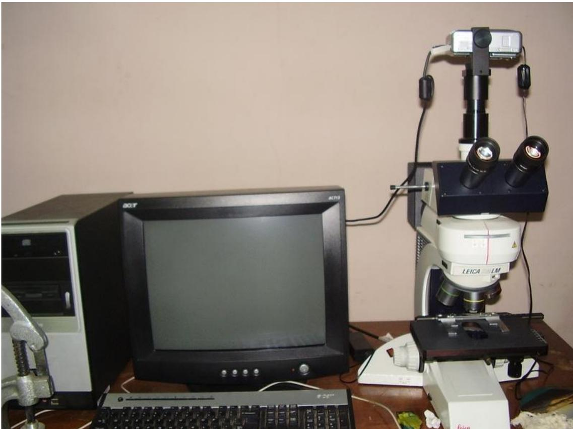
Fig 4.16 Metallurgical Microscope with image capturing device
