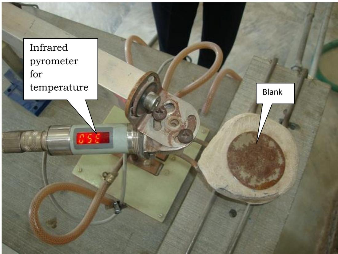
Fig 4.9. Blank Heating Arrangement with Temperature Measurement
