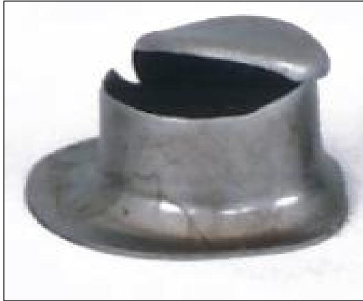
Fig. 1.8 Fracture in deep drawing [8]
