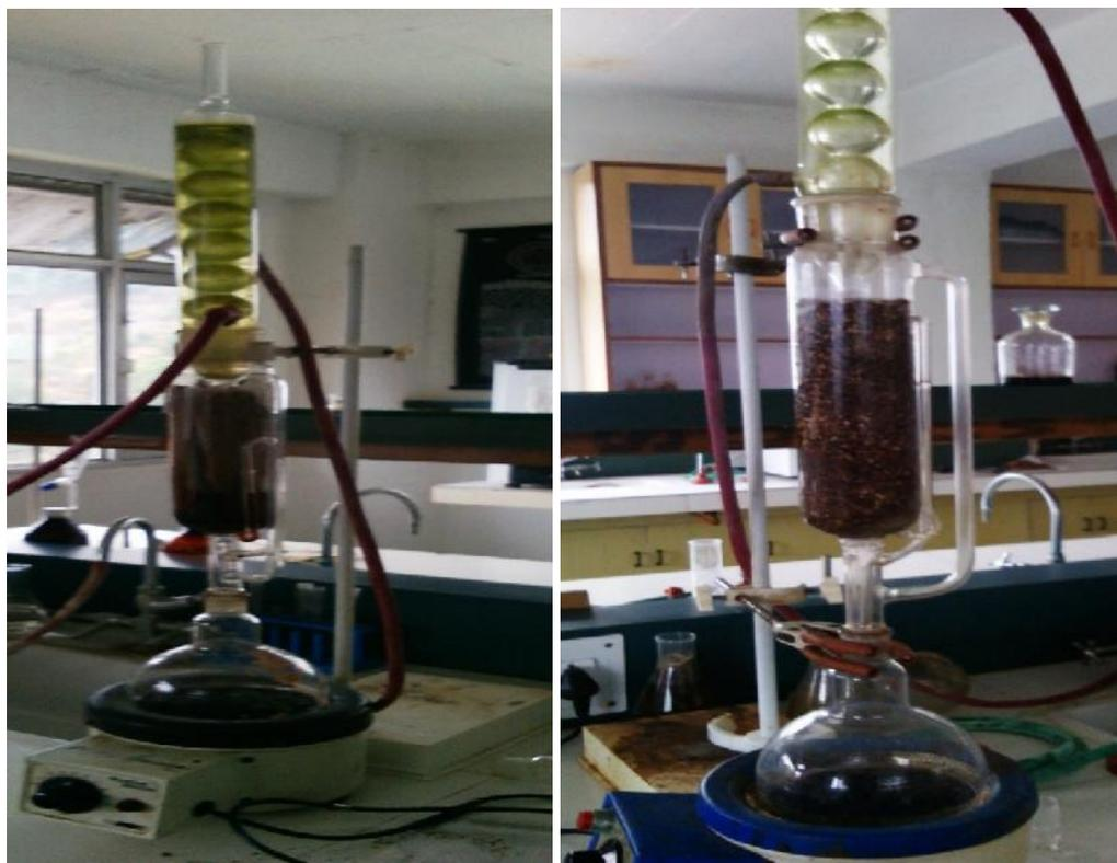
**Figure 3.2: Soxhlet apparatus**
