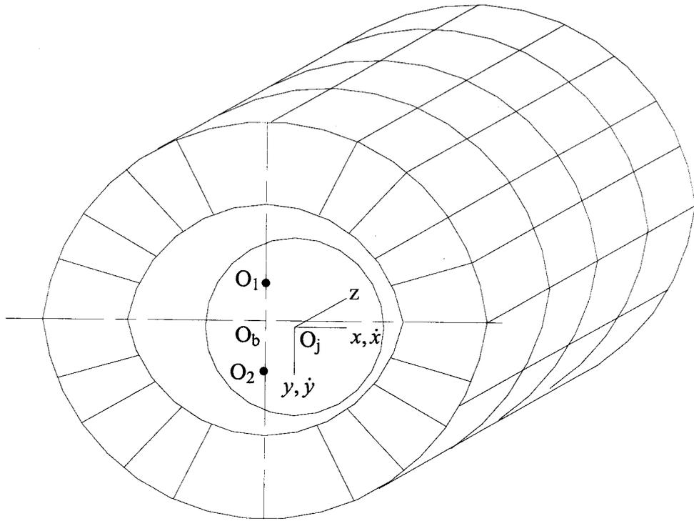
Fig. 2.7 Discretization of Two Lobe Bearing
