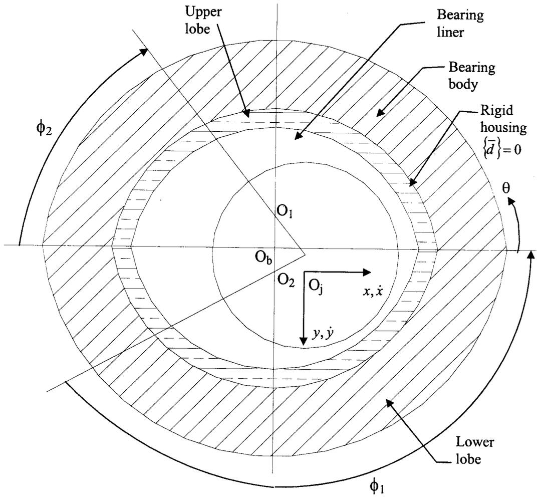
Fig. 2.2 Two Lobe Bearing Geometry
