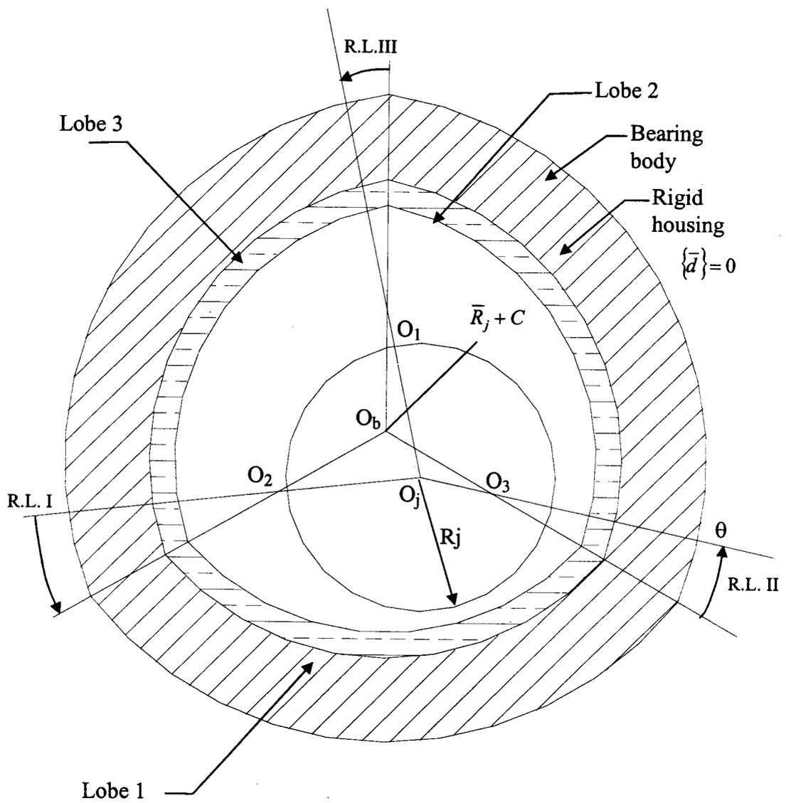
Fig. 2.3 Three Lobe Bearing Geometry
