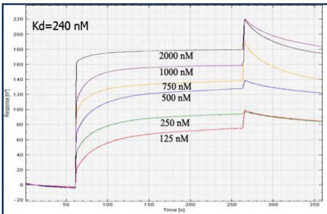
**Figure 3: SPR Sensogram:** Sensogram showing the interaction between Myosin IB-IQ motif peptide (IQKAWKGYRNRKRS) and EhCaBP5. Different concentrations of CaBP5 were injected onto the sensor chip to calculate the dissociation constant ( $K_d$ ).
