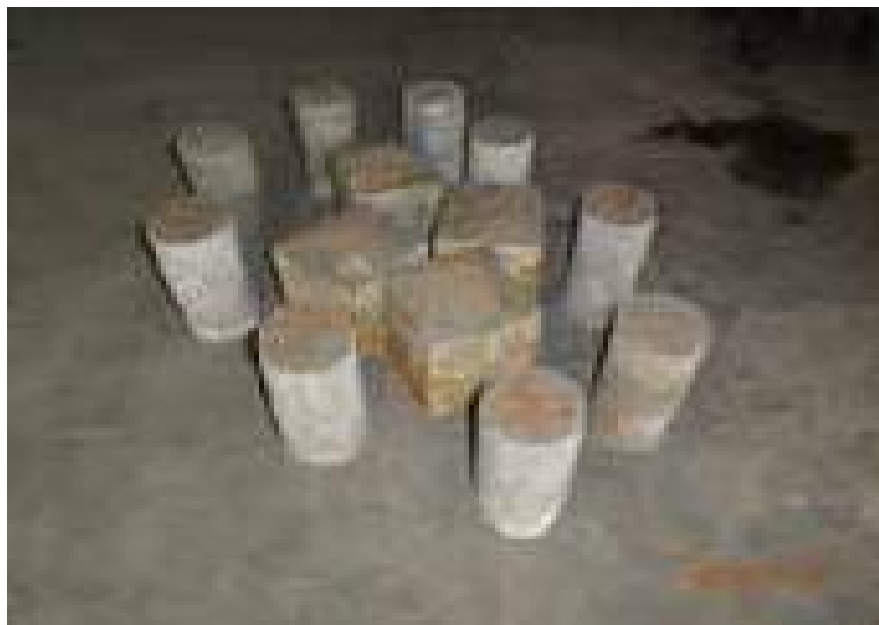
Figure 3.5 Specimen After Curing
