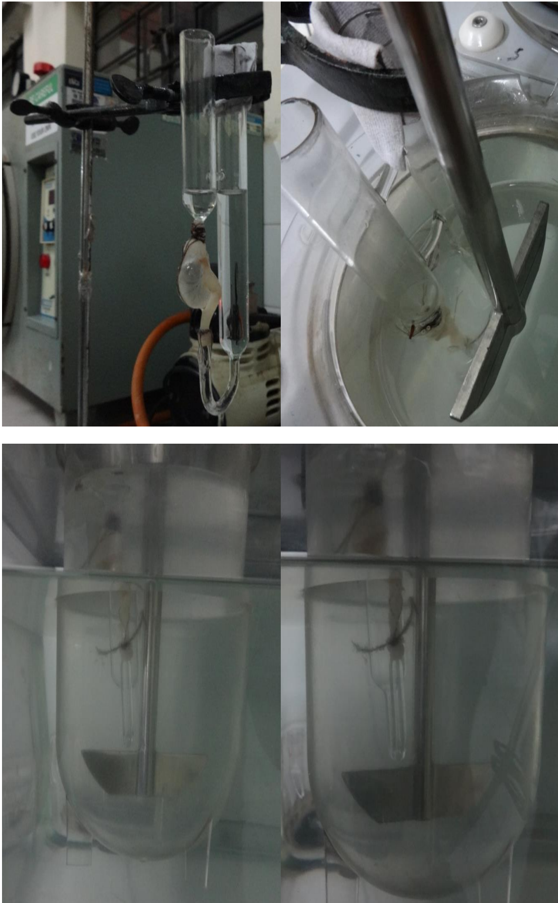
Fig. 11.2. Continuous dissolution–absorption system using everted rat stomach
