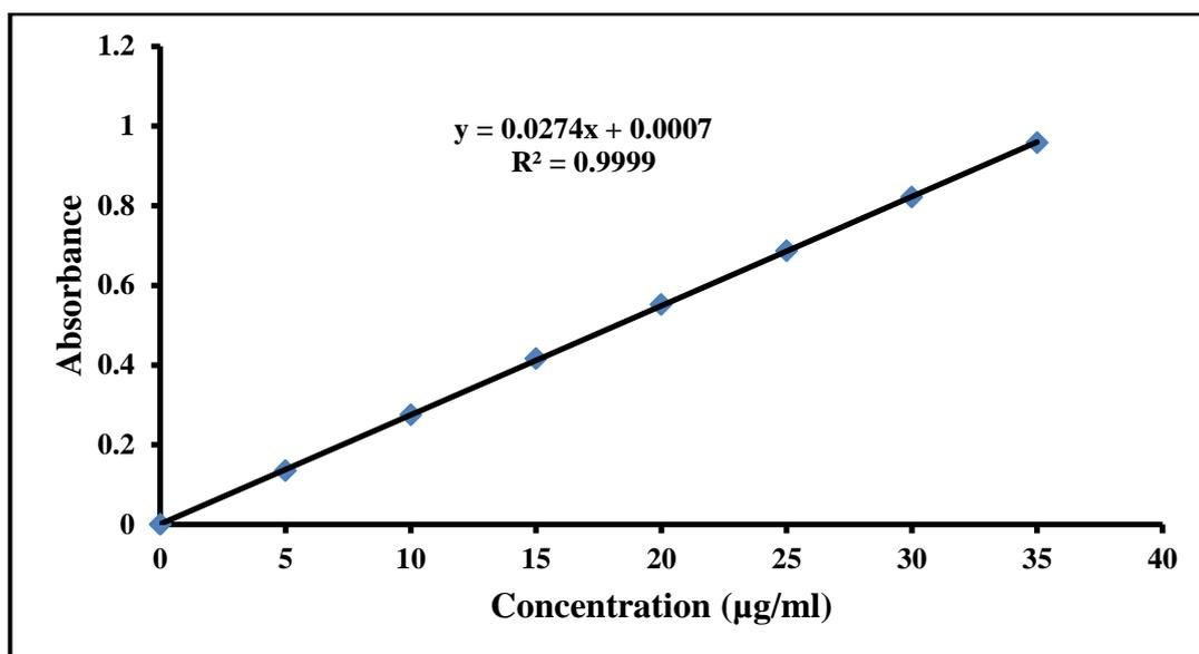
Fig. 5.5. Calibration curve of isoniazid in simulated intestinal fluid
