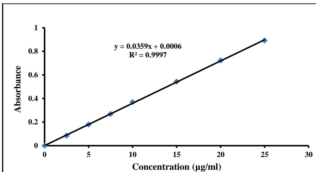
Fig. 5.6. Calibration curve of isoniazid in simulated gastric fluid
