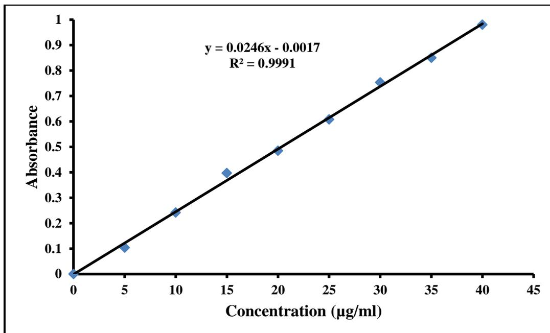
Fig. 5.3. Calibration curve of rifampicin in simulated intestinal fluid
