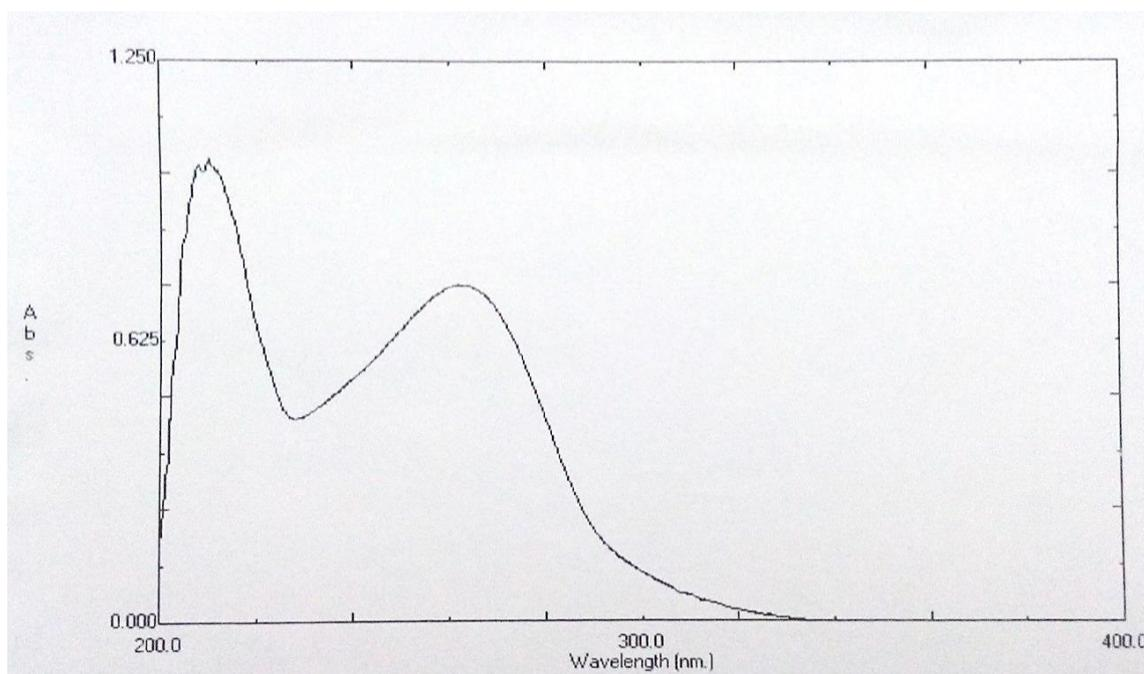
**Fig. 5.2. UV spectrum of isoniazid in simulated intestinal fluid**
