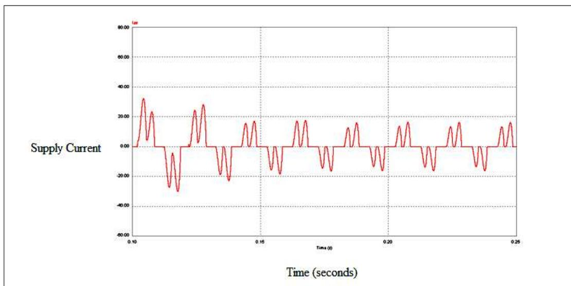
**Figure 3.12 Source current 20A/div. Time: 0.15s/div**
