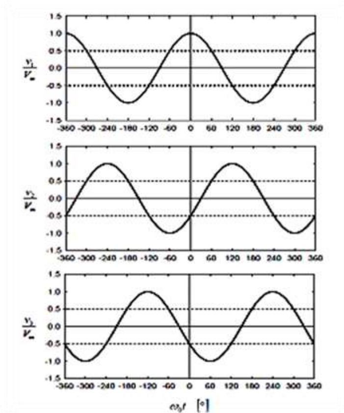
**Figure 3.3 Three phase input voltage**
