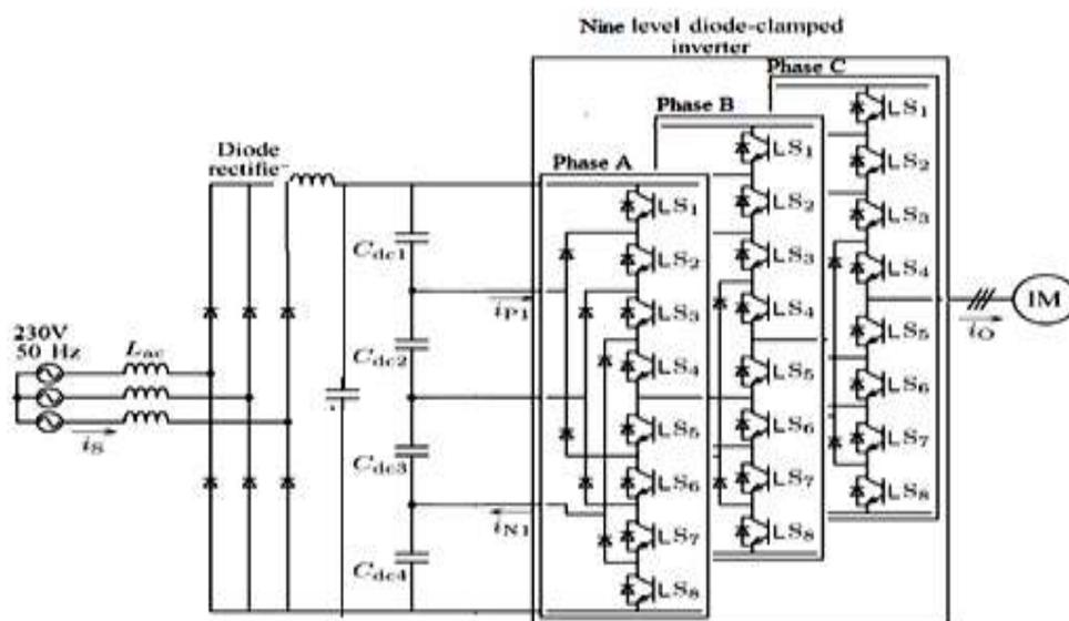
**Figure 3.1 Multilevel inverter with front end rectifier**
