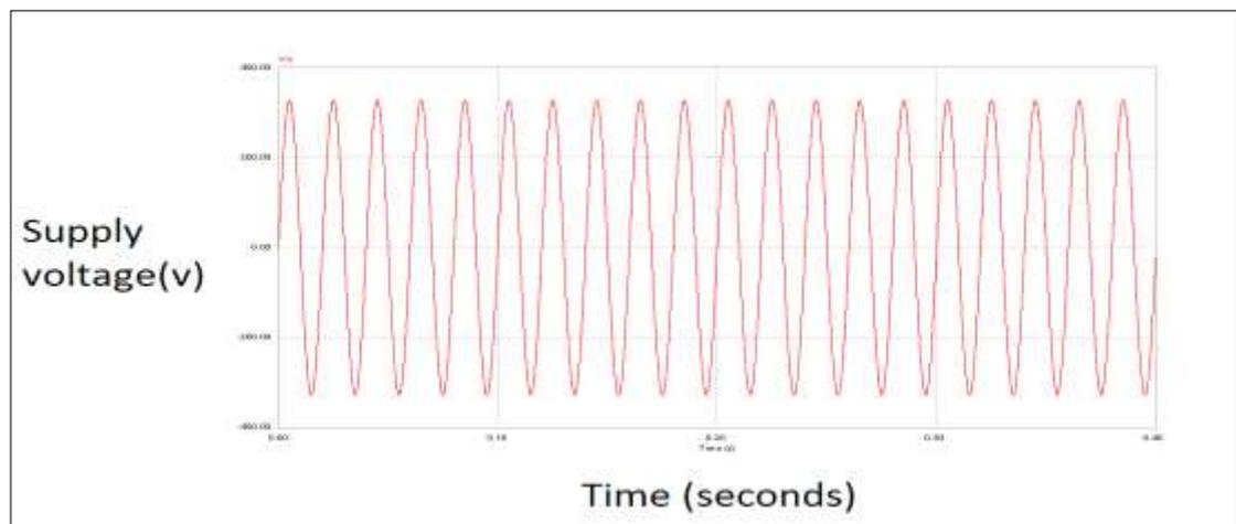
**Figure 3.11 Supply voltage 200V/div. Time: 0.10s/div**
