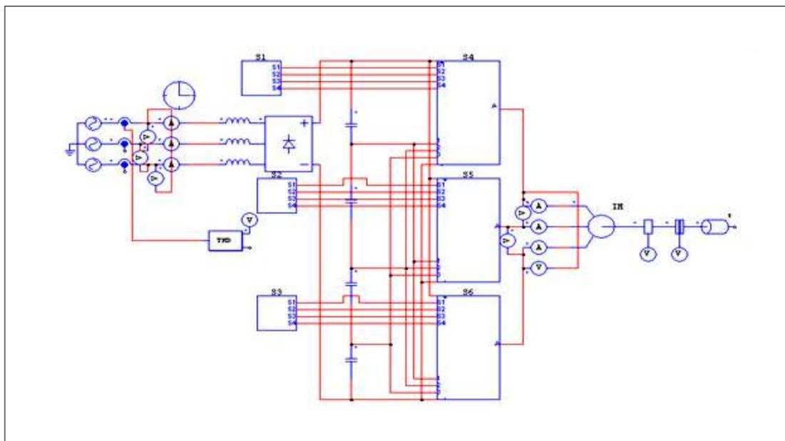
**Figure 3.9 PSIM model of nine level diode clamped multilevel inverter fed induction motor with front end rectifier**
