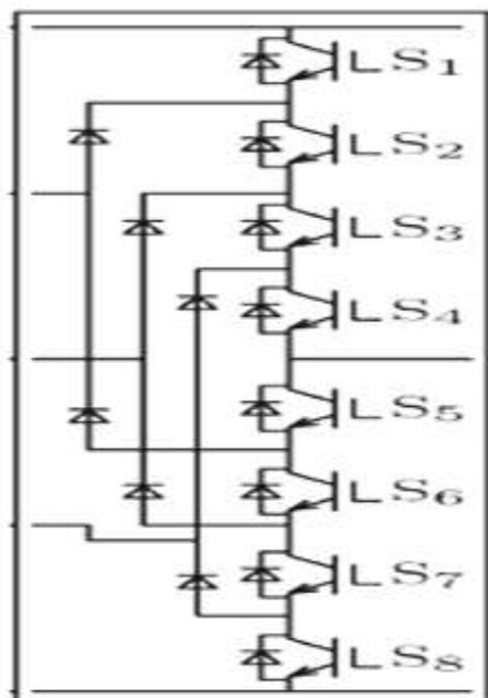
**Figure 3.8 Phase A of Nine level DCMLI**
