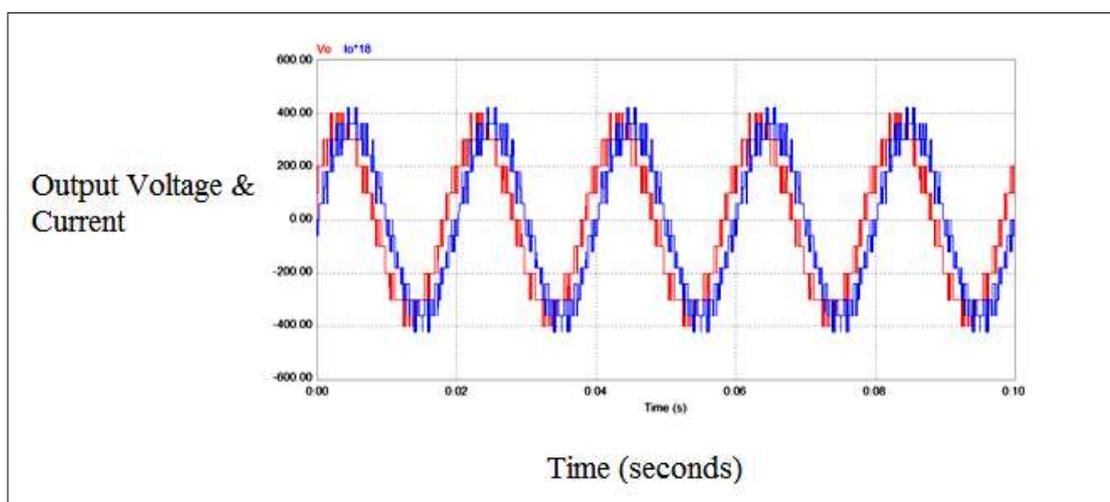
**Figure.3.13 Output voltage and current  $V_o$ : 200V/div.  $I_o$ :200A/div( $\div 18$ )
