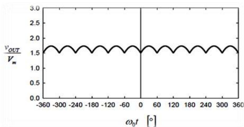
**Figure 3.5. Output voltage of the rectifier**
