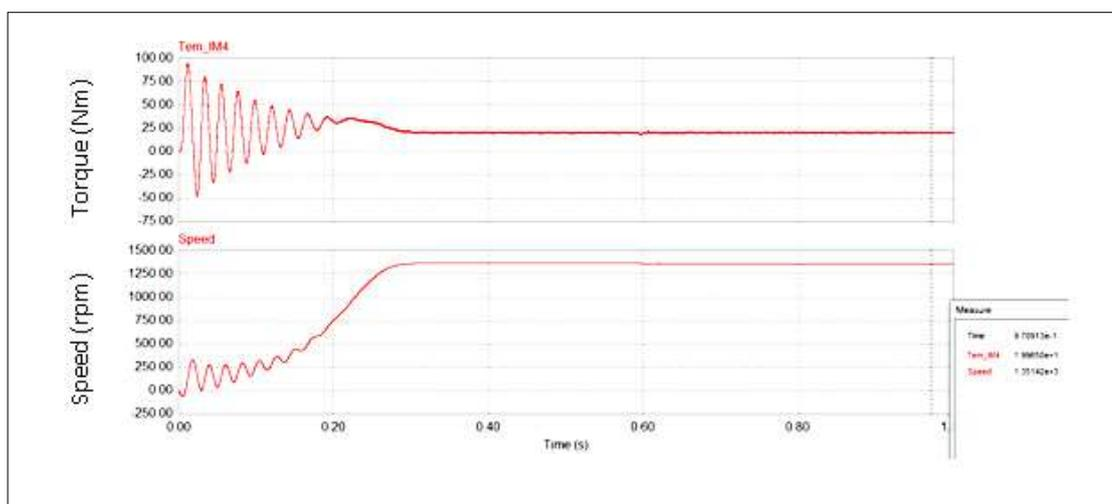
**Figure 3.16 Torque and Speed at full load (Simulation)**
