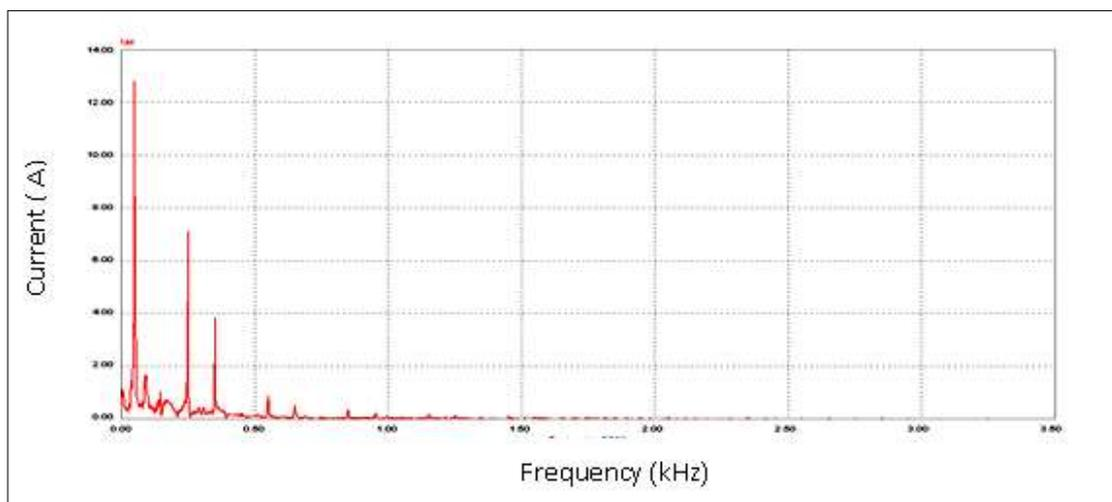
**Figure 3.15 FFT spectrum 2.0A/div. Frequency: 0.5kHz/div**
