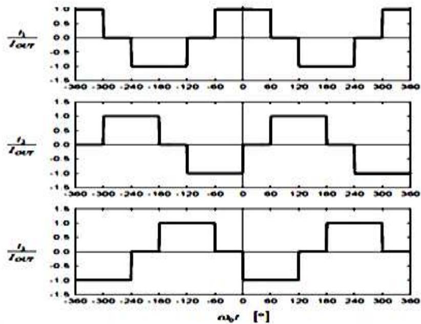
Figure 3.7 Input current waveforms
