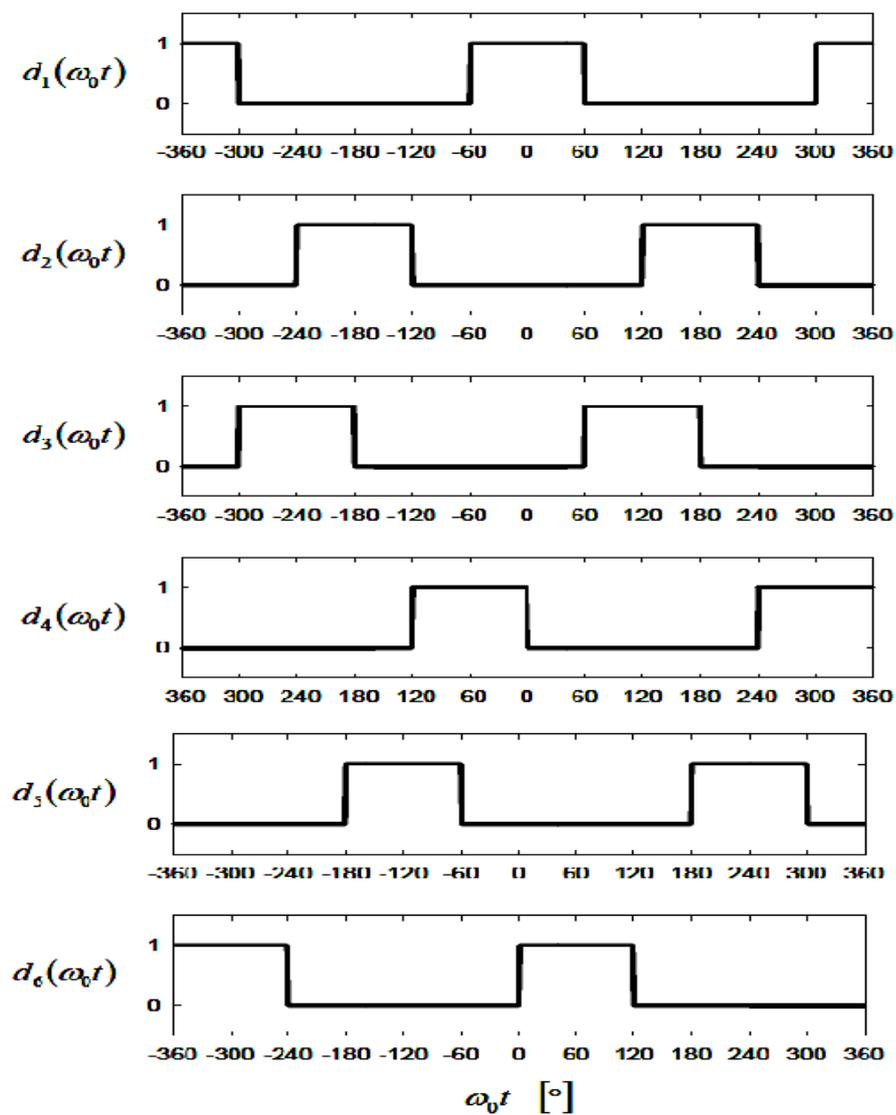
Figure 3.6 Diode conduction state function
