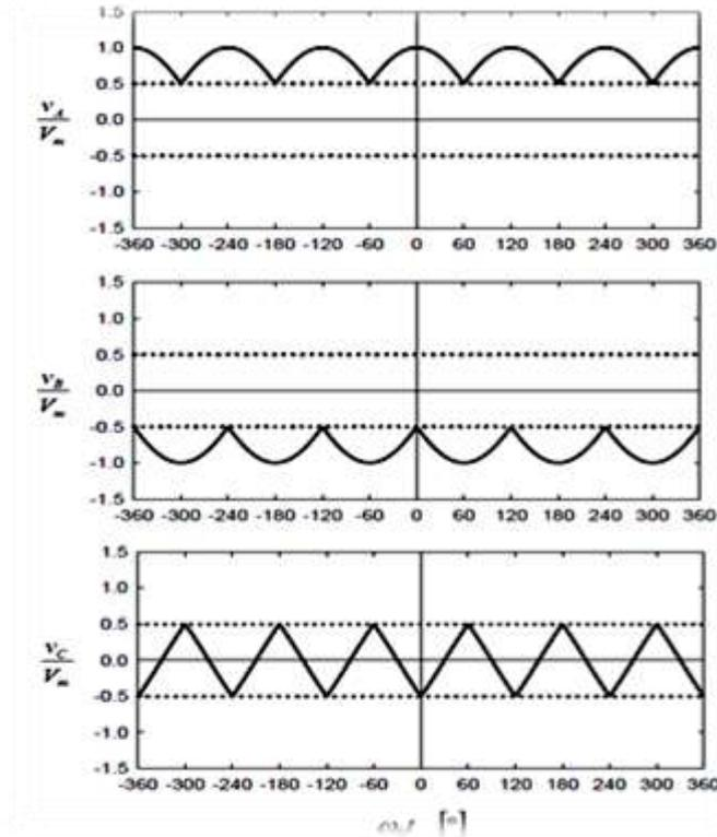
**Figure 3.4** Output voltages at terminal  $V_A$ ,  $V_B$ , and  $V_C$
