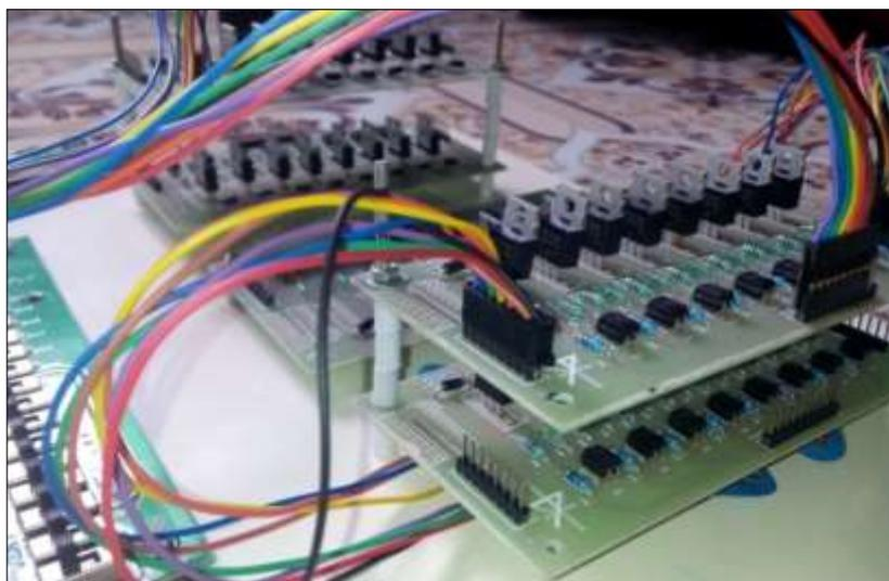
**Figure 5.20. Reconfigurable MOSFET switches**
