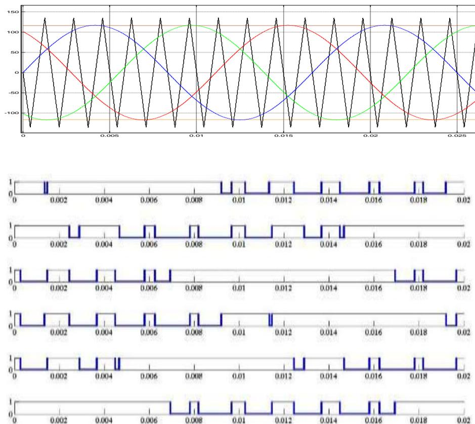
**Figure 5.5 PWM generation using maximum boost technique carrier signal, reference voltage and current signal ( $V_{carrier}, V_{ref}, i_{abc}$ )**
