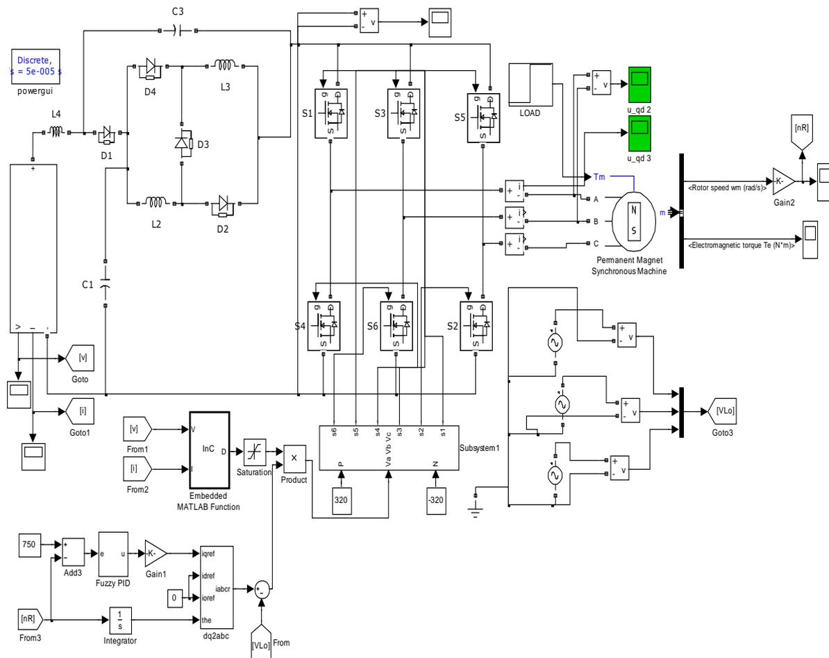
**Figure 5.9 Overall Simulation Implementation of Proposed Circuit and Control System**
