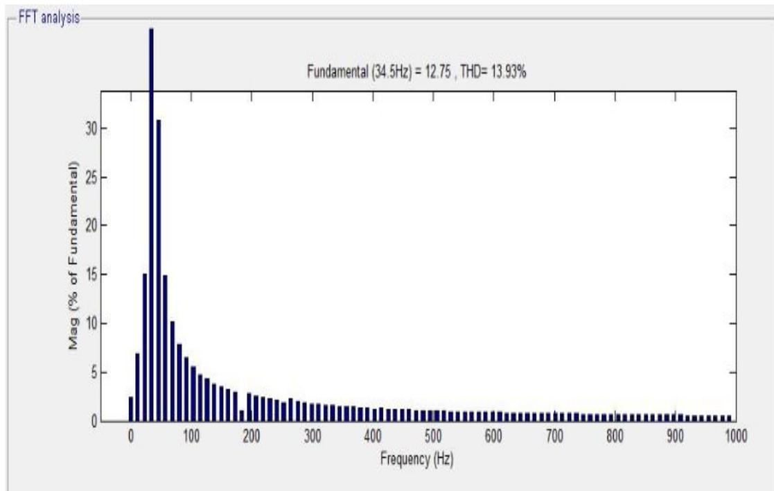
**Figure 5.12 FFT Analysis on Stator Current using Simple Maximum Boost PWM**
