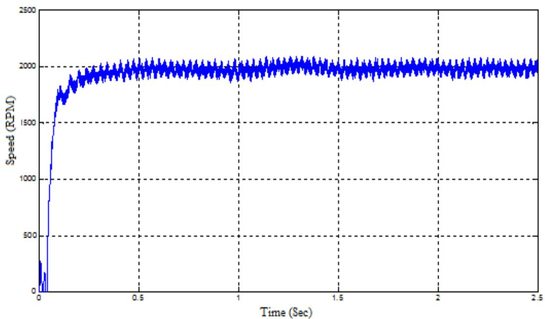
**Figure 5.13 Response of BLDC motor Speed**
