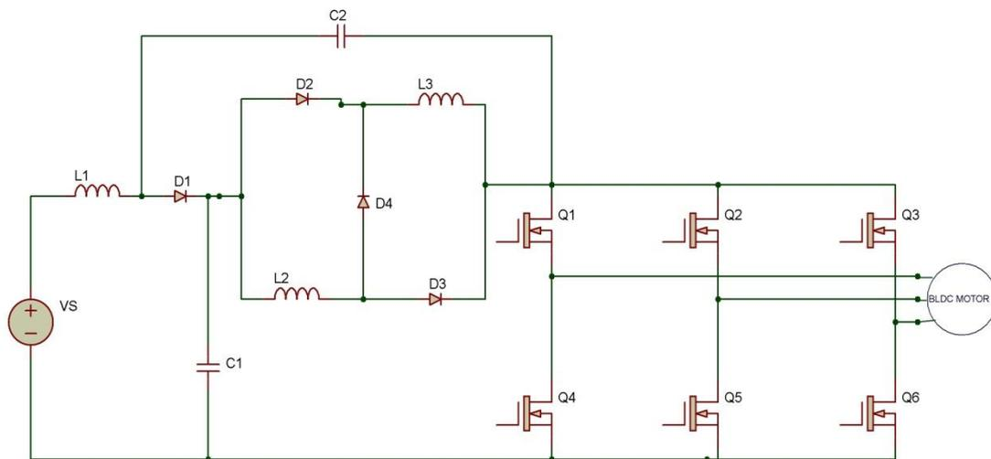
**Figure 5.1 Circuit Diagram of Switched Inductor Z –Source Inverter**
