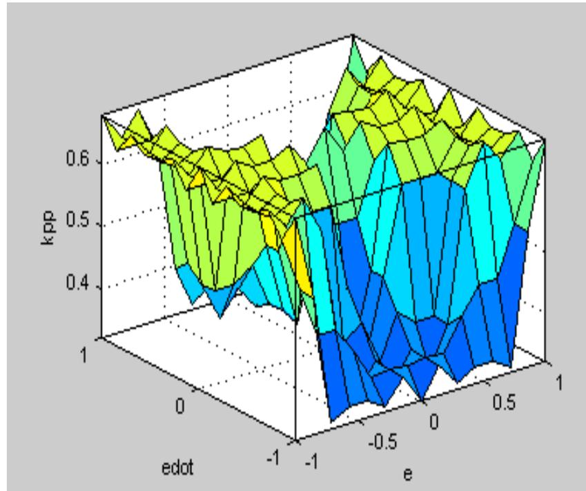
**Figure 5.8 Surface Diagram of Fuzzy**
