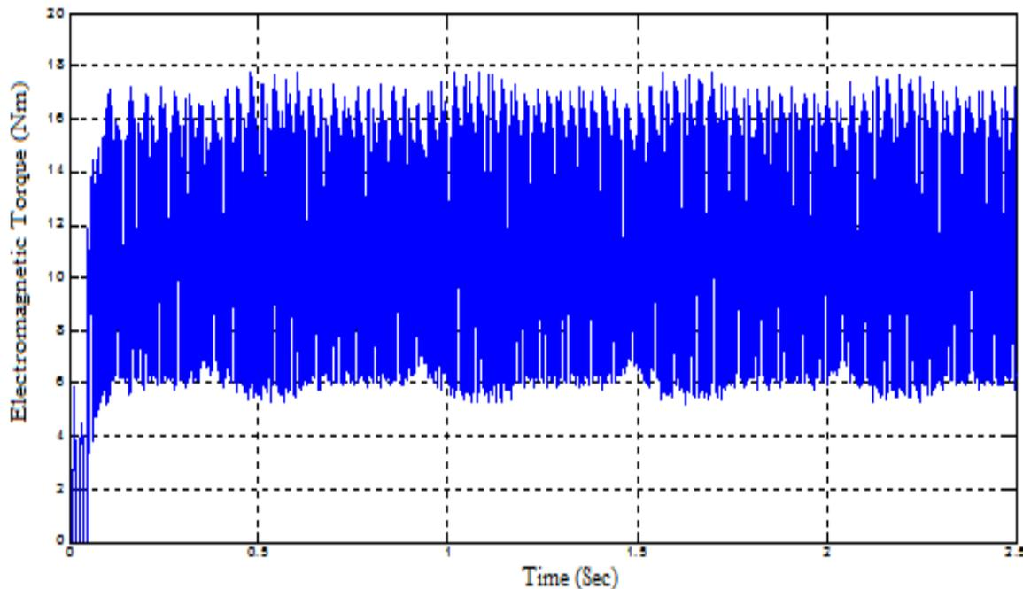
**Figure 5.14 Response of BLDC motors Electromagnetic Torque**
