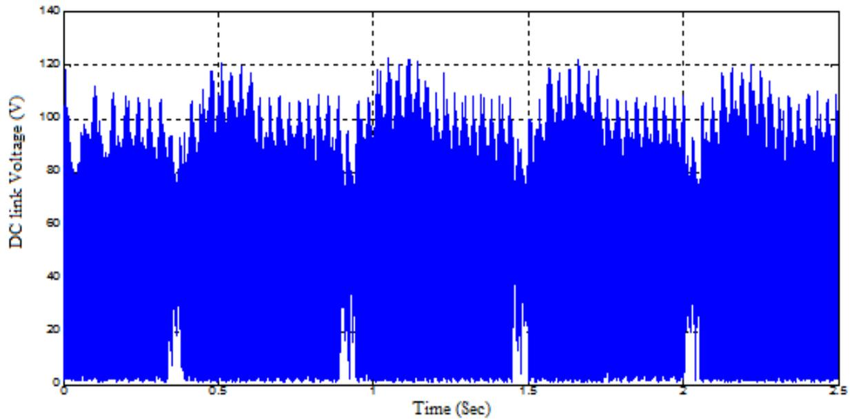
**Figure 5.10 DC-link voltage response of SLQZS Inverter**
