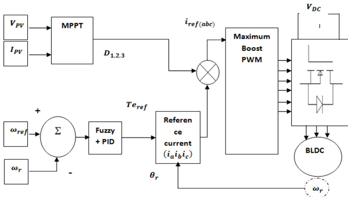
**Figure 5.4 Control Circuit for Sensor less Vector Control of BLDC Motor using Maximum boost PWM technique**
