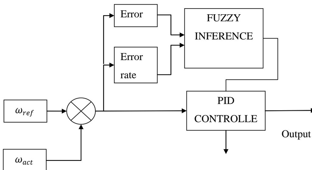
**Figure 5.6 Block Diagram of self-tuning fuzzy PID controller**
