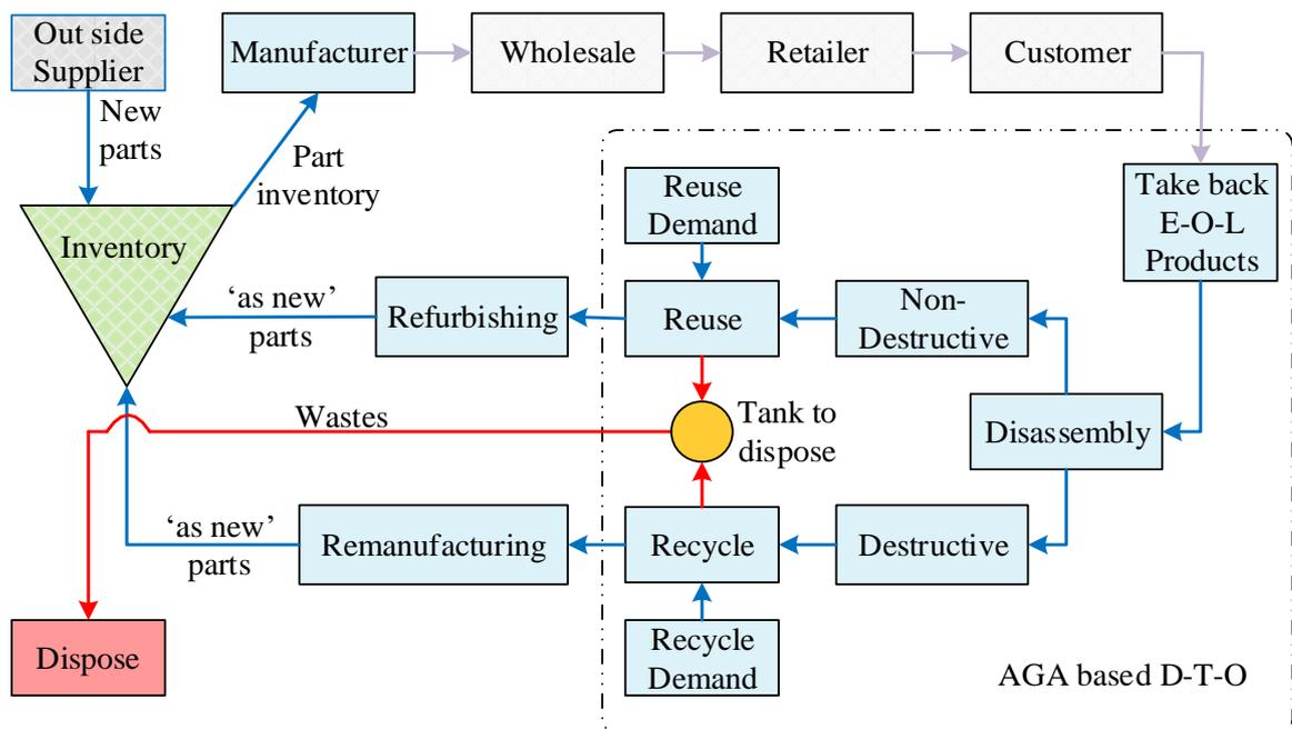
Figure 4.2. AGA based E-O-L Reverse Logistic Architecture
