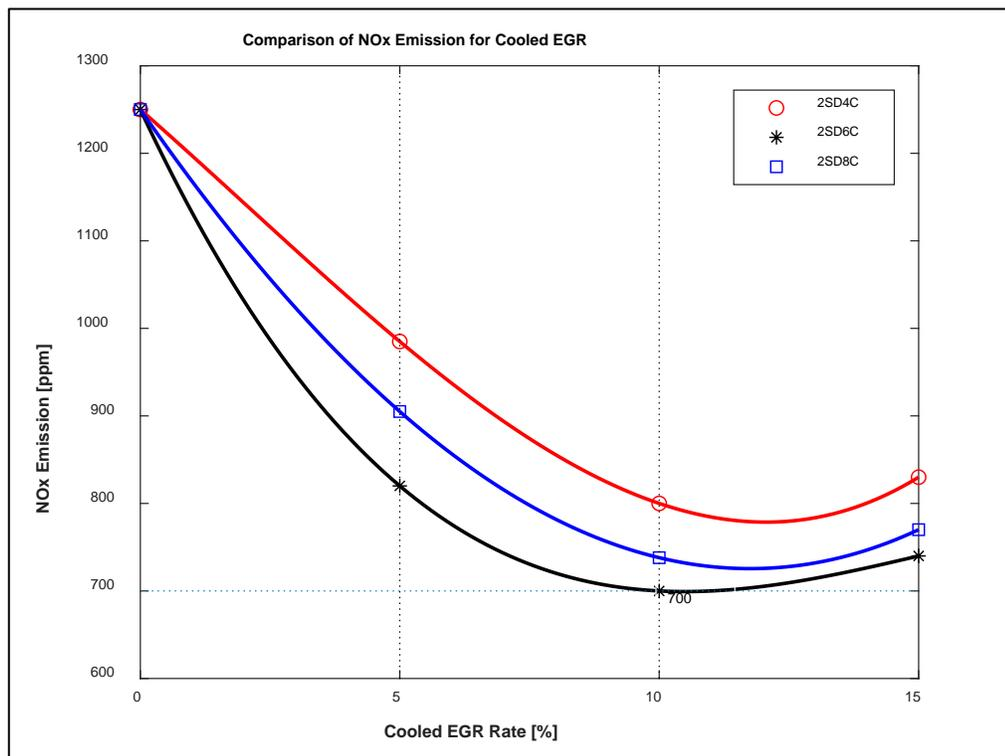
**Figure 4.26 EGR Rate vs. NOx Emission cooled EGR**
