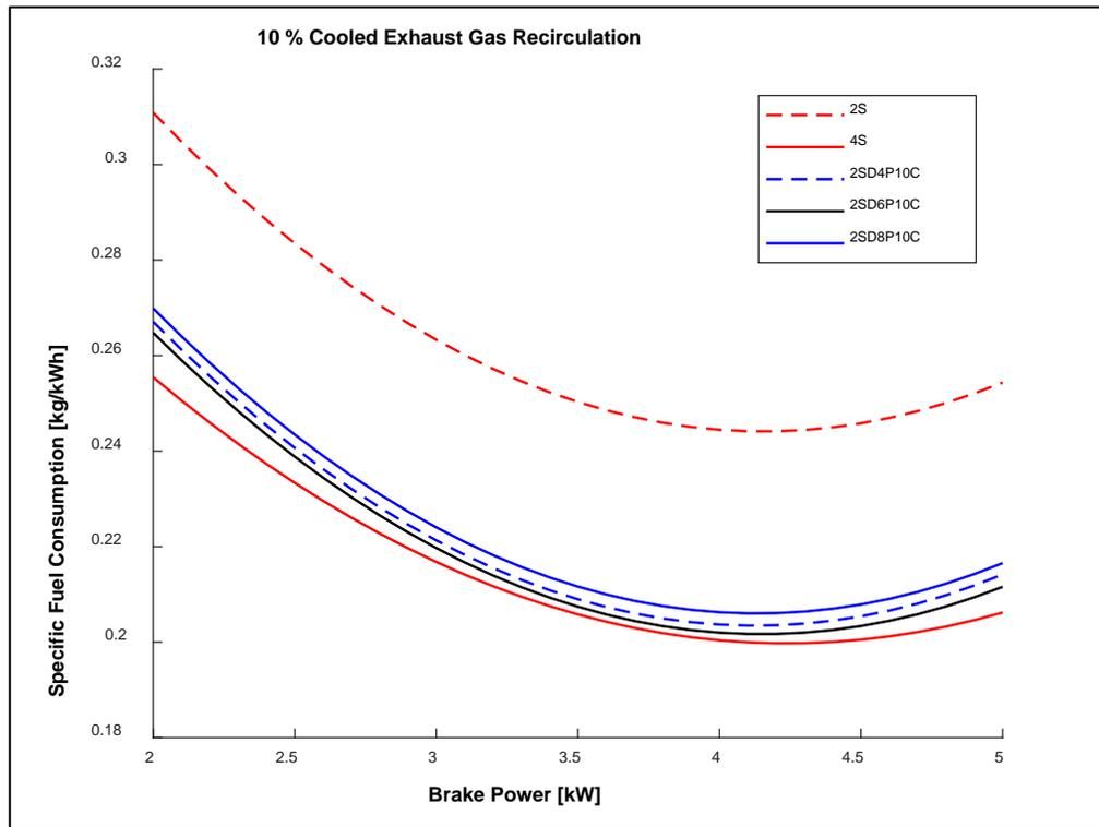
**Figure 4.11 Brake Power vs. Specific Fuel Consumption
