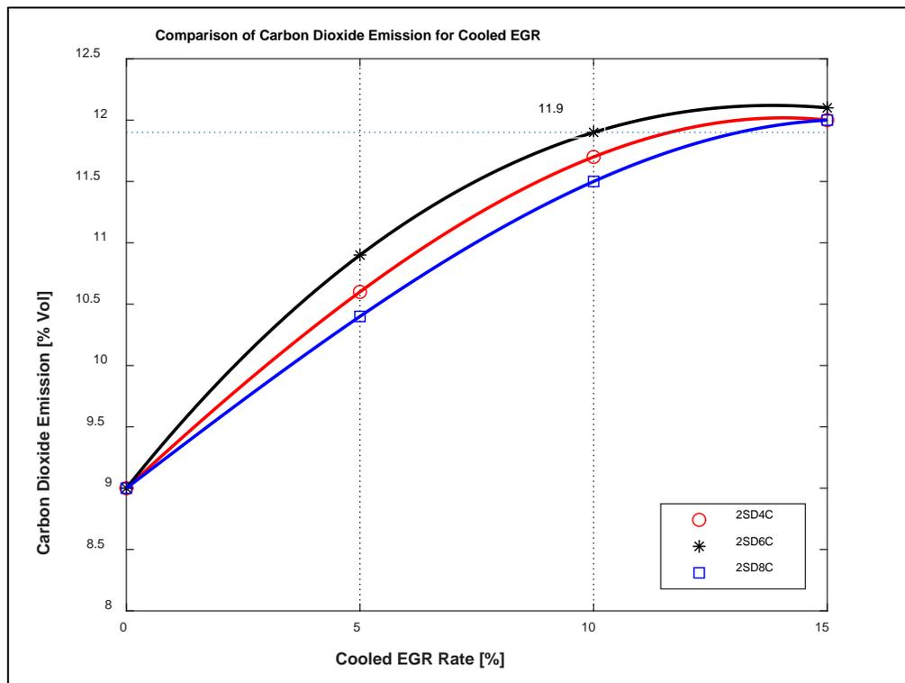
**Figure 4.22 EGR Rate vs. CO<sub>2</sub> Emission cooled EGR**
