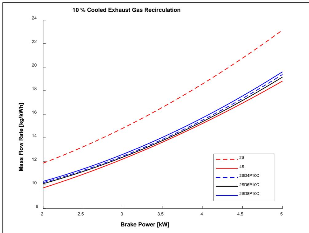
**Figure 4.15 Brake Power vs. Mass Flow Rate 10 % cooled EGR**
