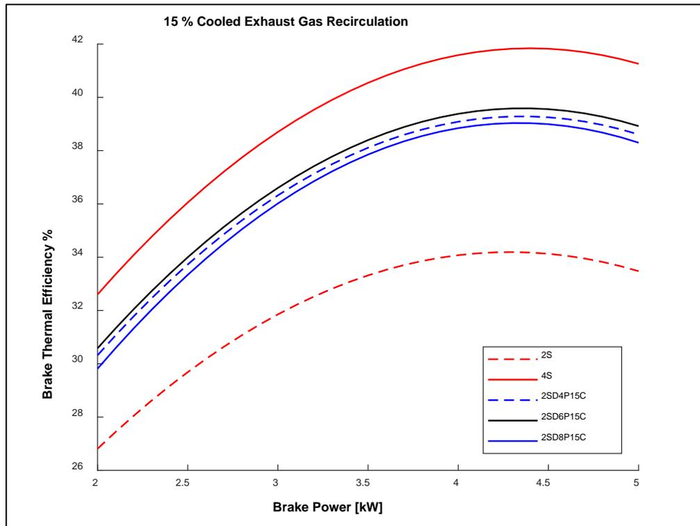
**Figure 4.6 Brake Power vs. Brake Thermal Efficiency
