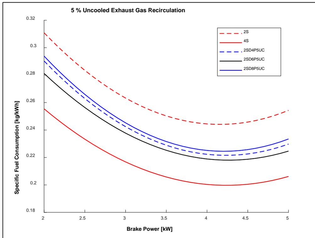
**Figure 4.8 Brake Power vs. Specific Fuel Consumption
