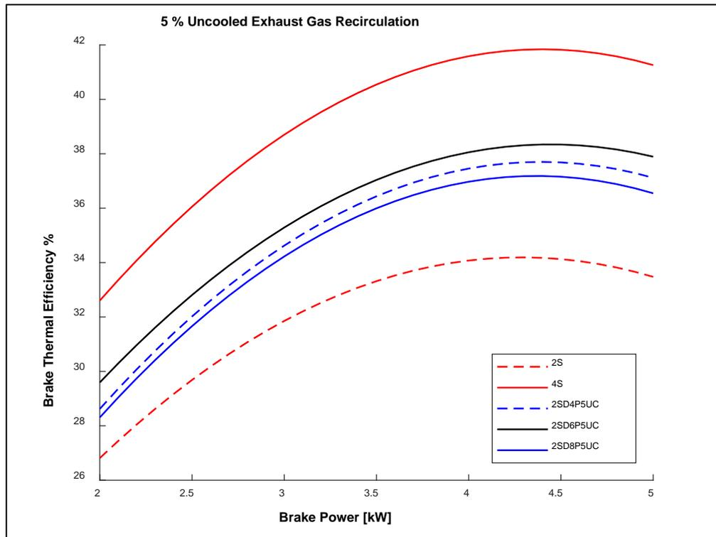
**Figure 4.1 Brake Power vs. Brake Thermal Efficiency
