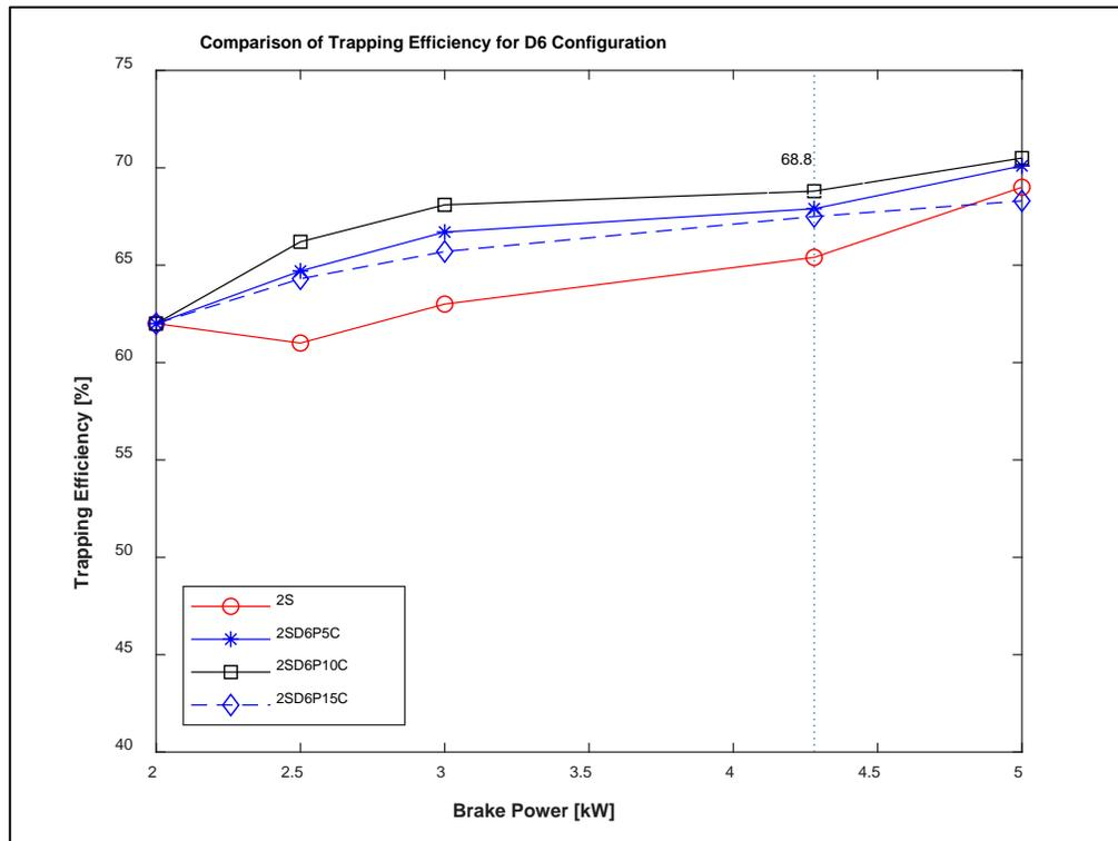
**Figure 4.18 Brake Power vs. Trapping Efficiency 6 mm orifice**
