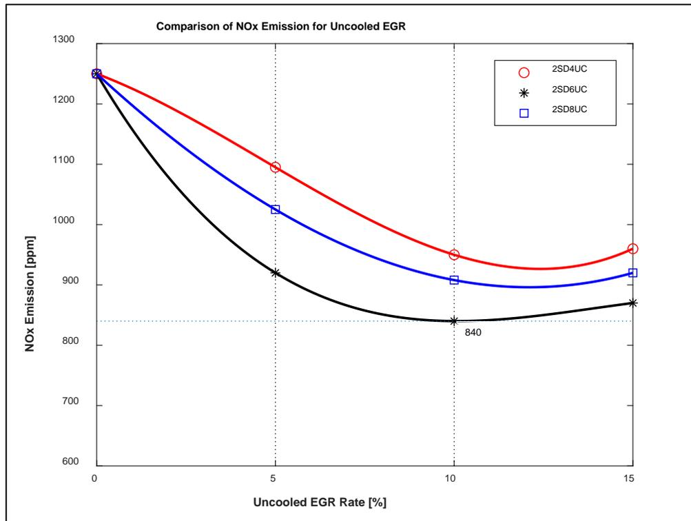
**Figure 4.25 EGR Rate vs. NOx Emission uncooled EGR**
