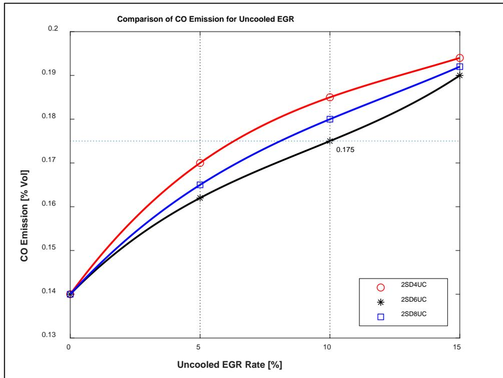
**Figure 4.19 EGR Rate vs. CO Emission for uncooled EGR**
