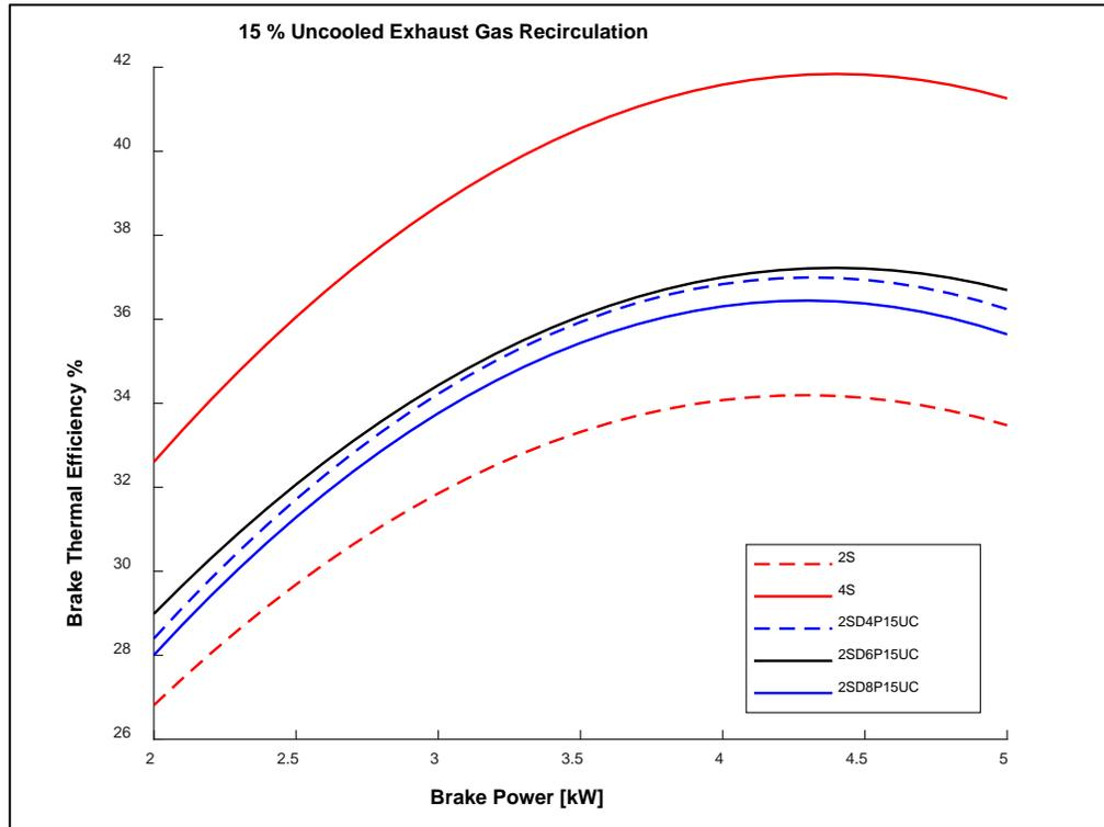
**Figure 4.5 Brake Power vs. Brake Thermal Efficiency
