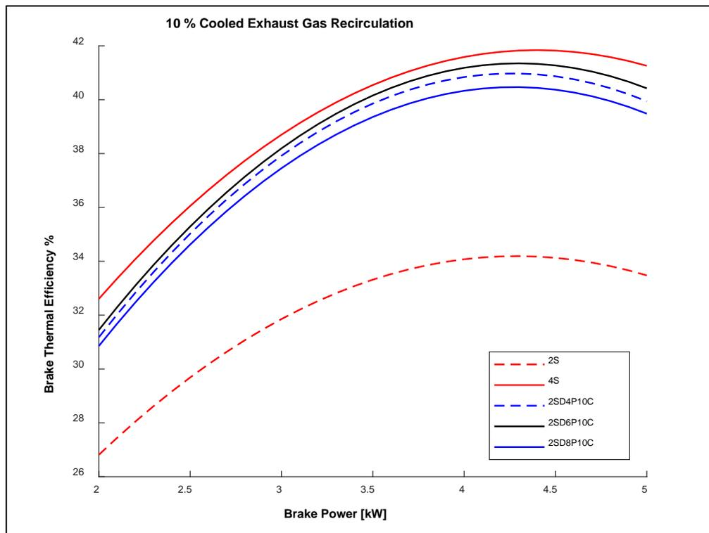
**Figure 4.4 Brake Power vs. Brake Thermal Efficiency
