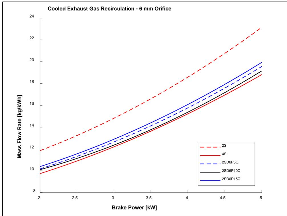
**Figure 4.16 Brake Power vs. Mass Flow Rate 6 mm orifice**
