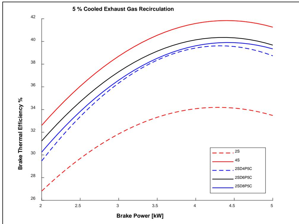
**Figure 4.2 Brake Power vs. Brake Thermal Efficiency
