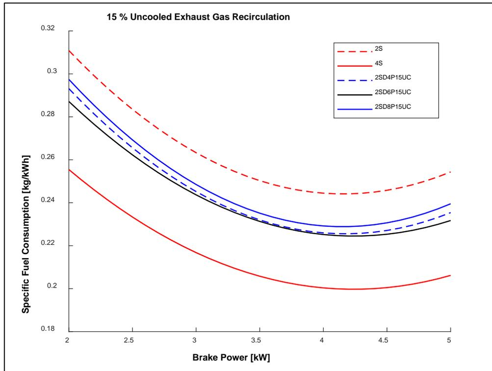
**Figure 4.12 Brake Power vs. Specific Fuel Consumption
