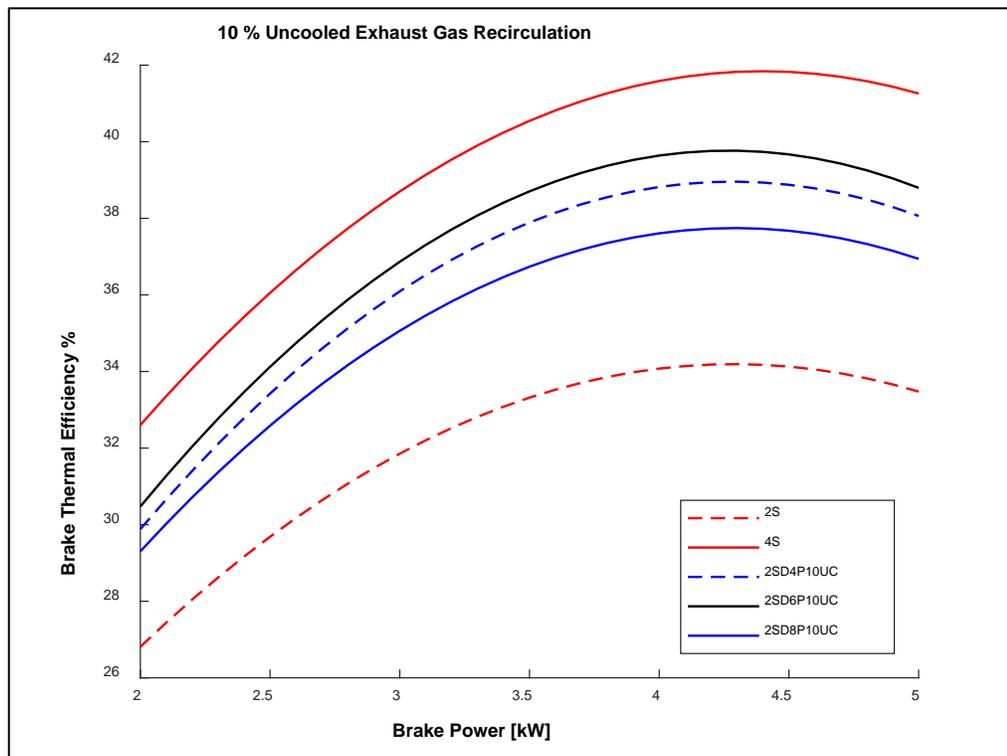
**Figure 4.3 Brake Power vs. Brake Thermal Efficiency
