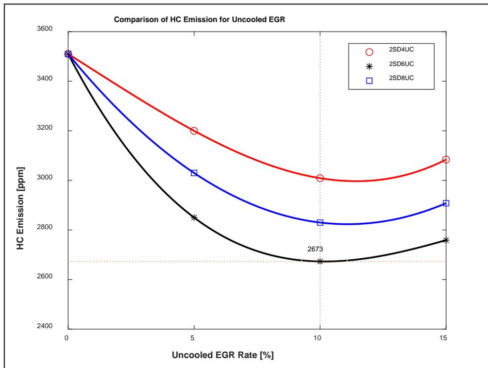
**Figure 4.23 EGR Rate vs. HC Emission uncooled EGR**
