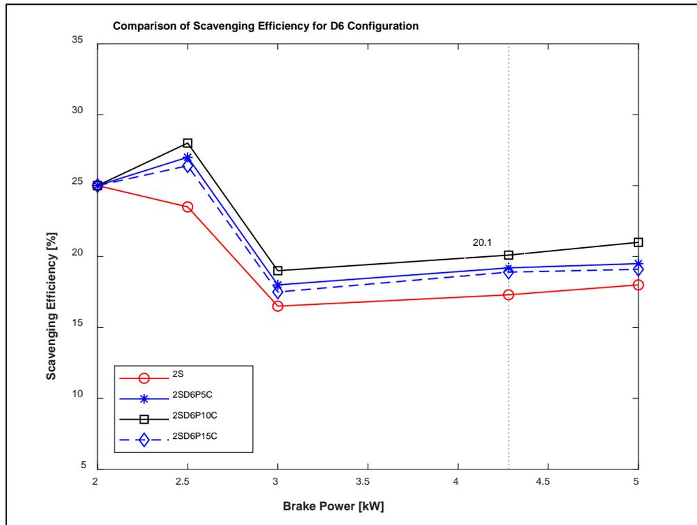
**Figure 4.17 Brake Power vs. Scavenging Efficiency 6 mm orifice**
