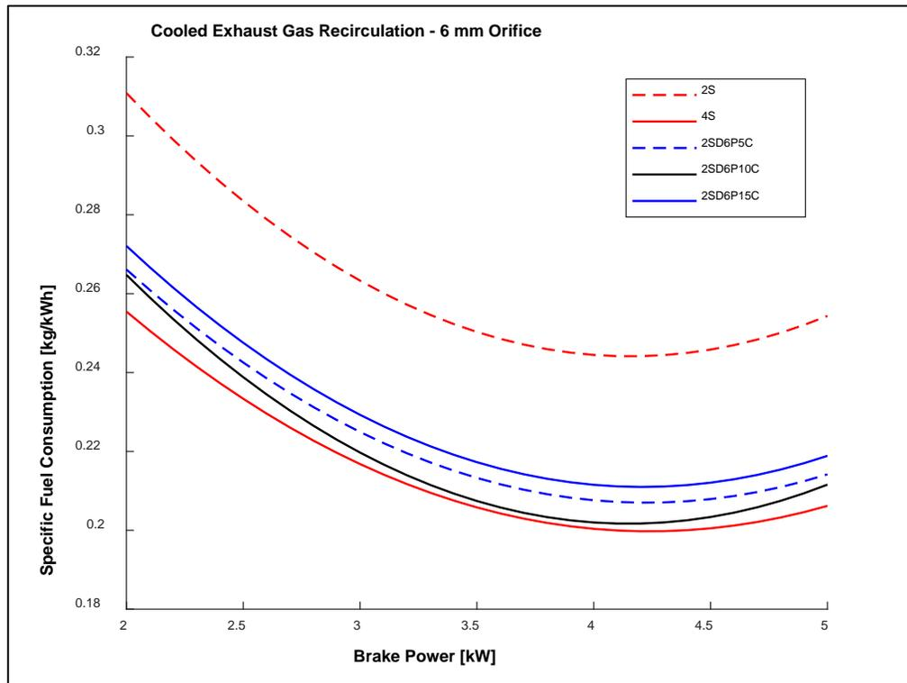
**Figure 4.14 Brake Power vs. Specific Fuel Consumption
