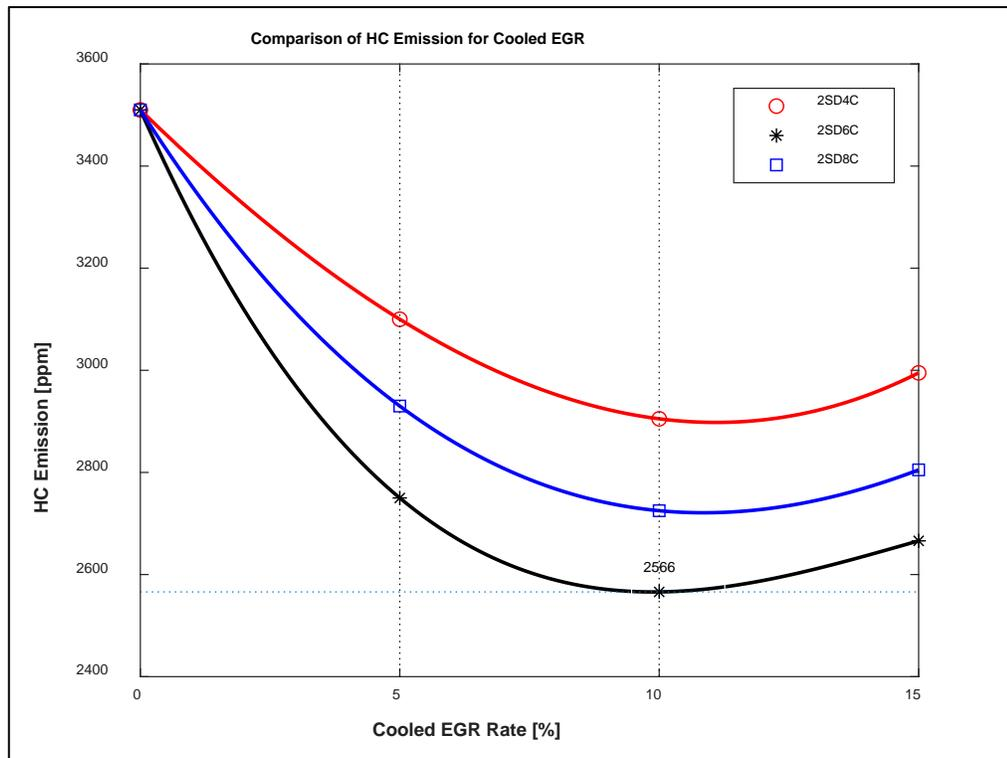
**Figure 4.24 EGR Rate vs. HC Emission cooled EGR**
