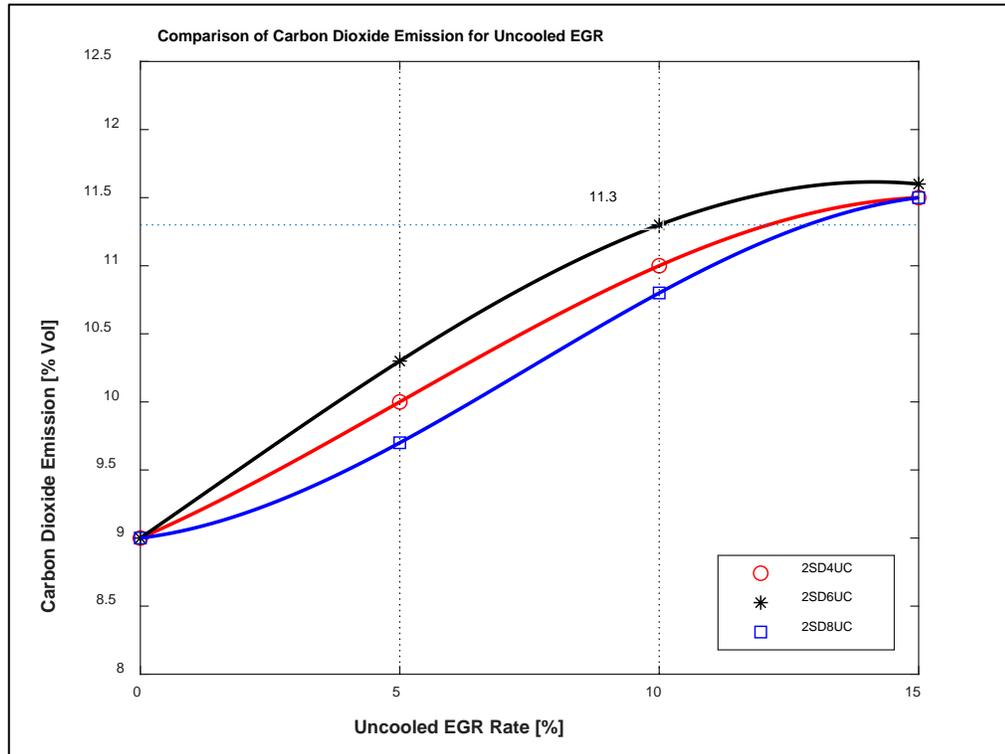
**Figure 4.21 EGR Rate vs. CO<sub>2</sub> Emission uncooled EGR**
