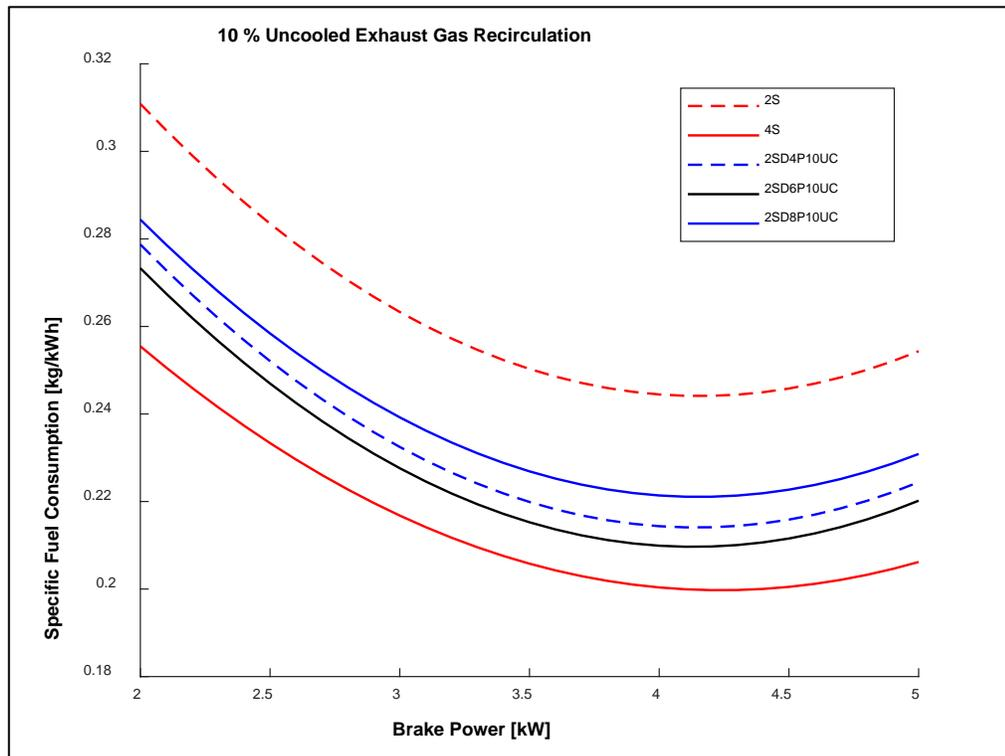
**Figure 4.10 Brake Power vs. Specific Fuel Consumption
