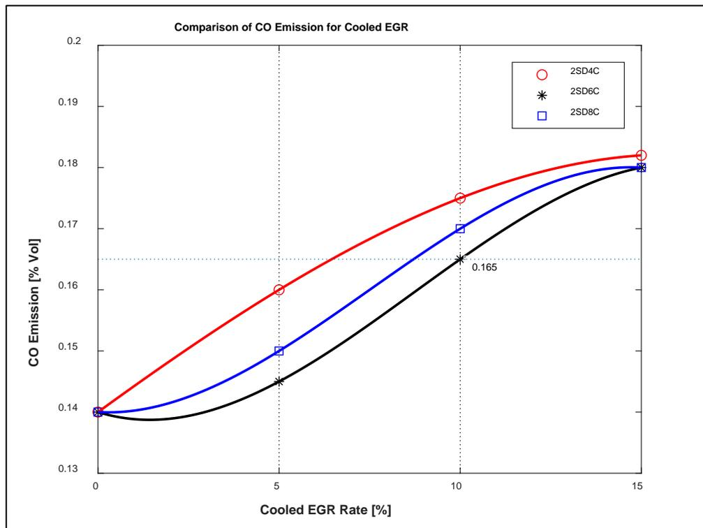
**Figure 4.20 EGR Rate vs. CO Emission cooled EGR**
