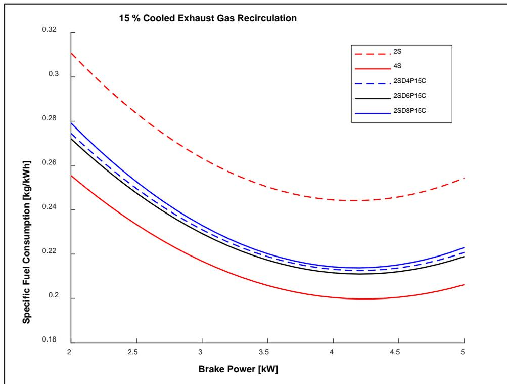
**Figure 4.13 Brake Power vs. Specific Fuel Consumption
