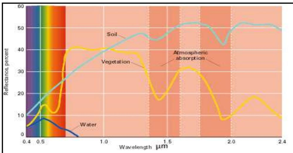
Figure 2.4: Spectral signatures of various cover types
