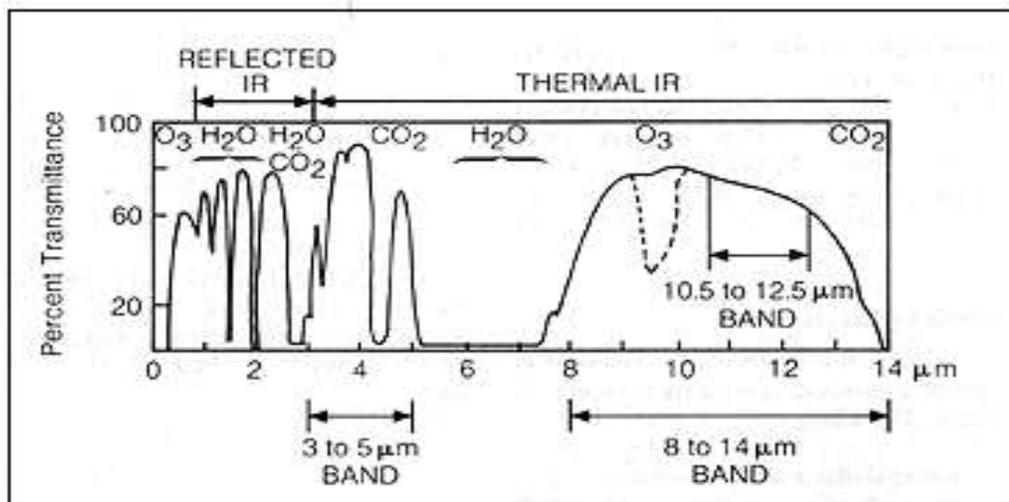
Figure 2.5: Thermal transmittance curve
