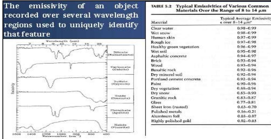
Figure 2.8: Emissivities of minerals and of various common materials
