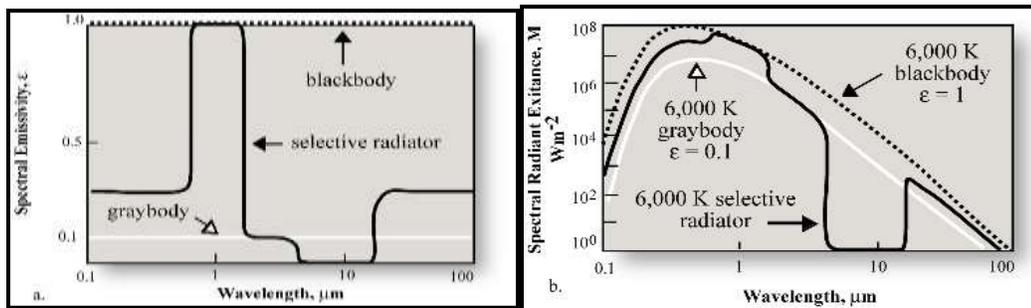
Figure 2.7: Spectral emissivity of a blackbody, a gray body, and a hypothetical selective radiator
