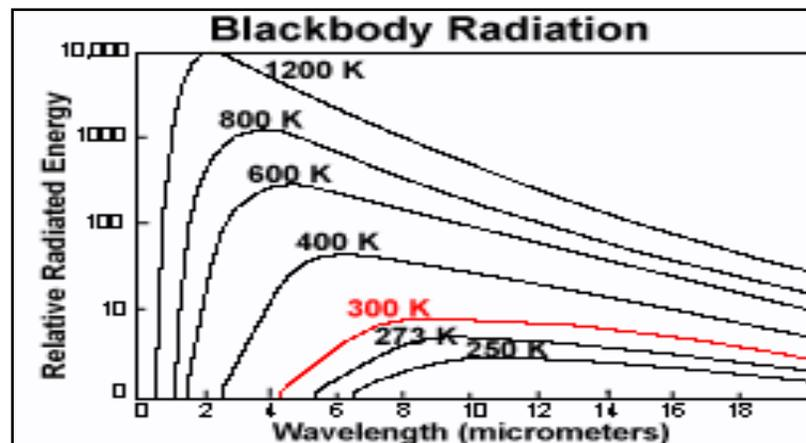
Figure 2.6: Wien Displacement law and emissivity effects
