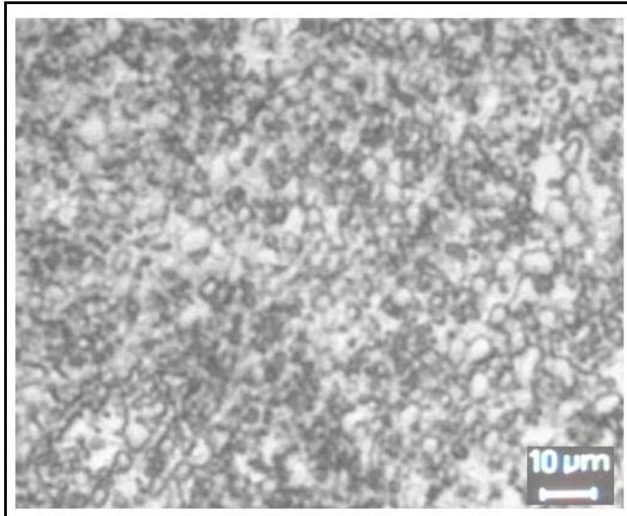
**Figure 5.3** Microstructure of untreated annealed AISI 52100 steel sample.
