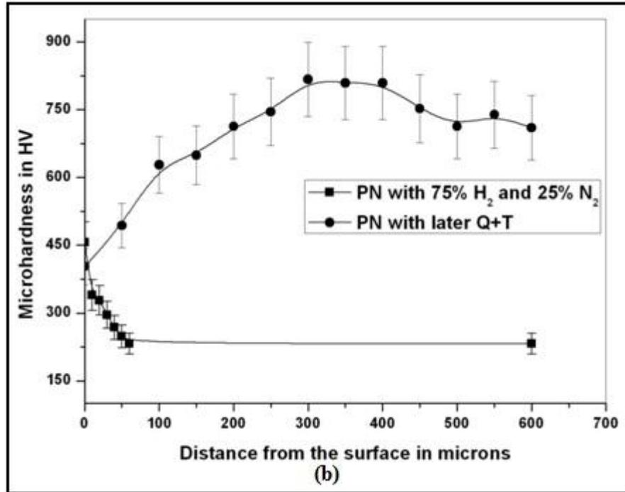
**Figure 5.7:** Micro-hardness profiles with diffusion depth in plasma nitrided samples after heat treatments (a) Plasma nitrided with 75% Ar – 25% N<sub>2</sub>, (b) Plasma nitrided with 75% H<sub>2</sub> – 25% N<sub>2</sub>.
