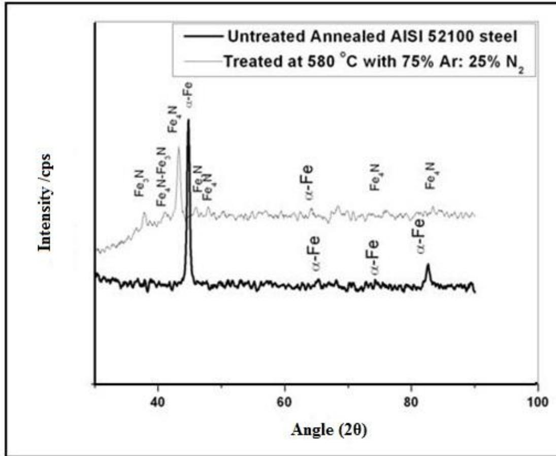
**Figure 5.6:** X-ray diffraction patterns of untreated sample and 25% Nitrogen and 75% Argon gas plasma nitrided sample.
