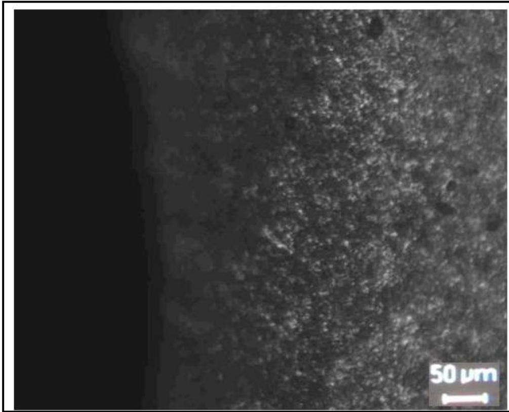
**Figure 5.8:** Microstructure of 25% Nitrogen and 75% Argon gas plasma nitrided annealed sample after quenching and tempering (Q+T).
