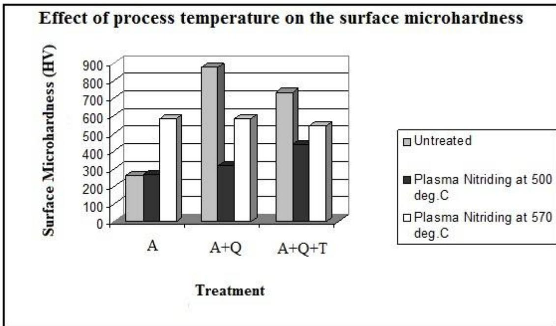
**Figure 5.1:** Effect of the process temperature on surface microhardness.
