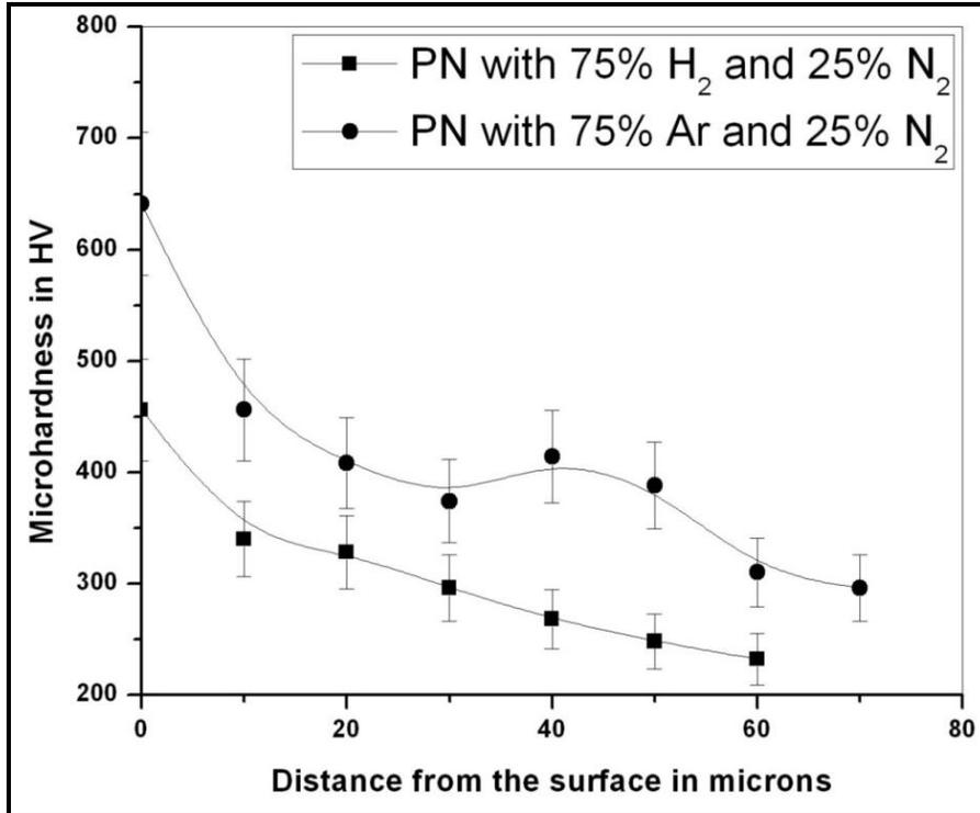
**Figure 5.5:** Micro-hardness profile with diffusion depth in plasma nitrided samples.
