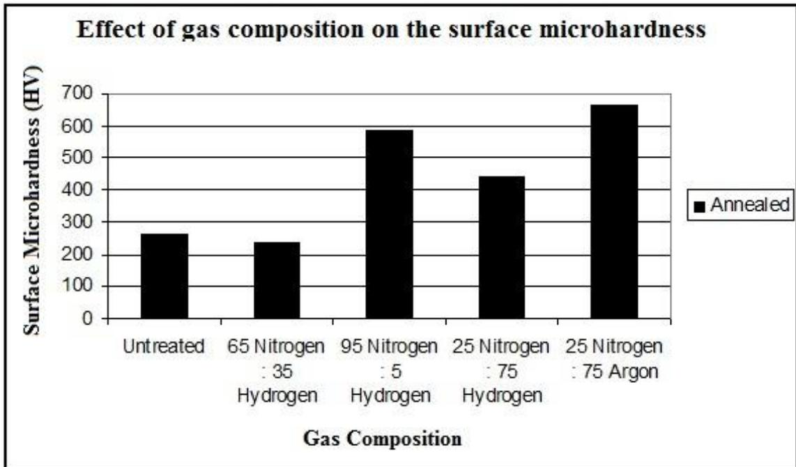
**Figure 5.2:** Effect of gas compositions on the surface microhardness.
