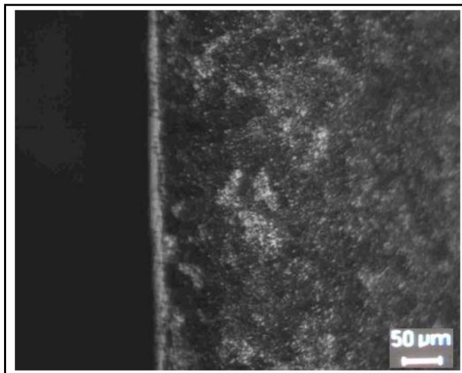
**Figure 5.4:** Microstructure of 25% Nitrogen and 75% Argon gas plasma nitrided sample.
