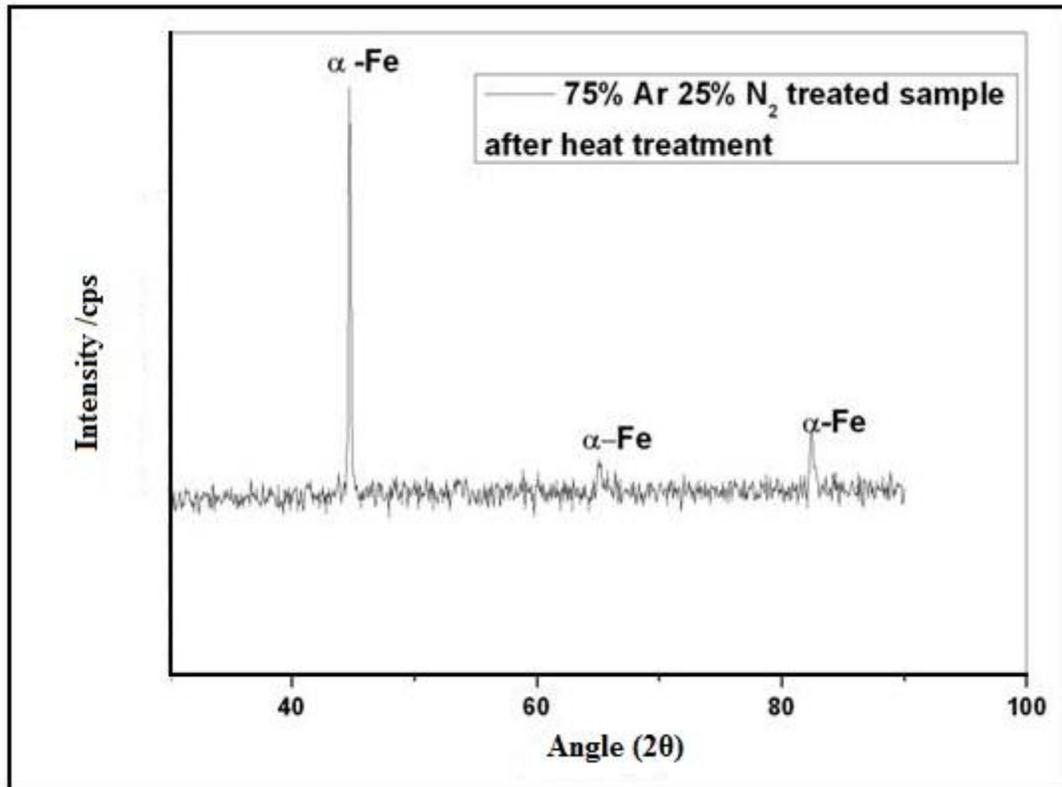
**Figure 5.9:** X-ray diffraction pattern of 25% Nitrogen and 75% Argon gas plasma nitrided sample after quenching and tempering (Q+T).
