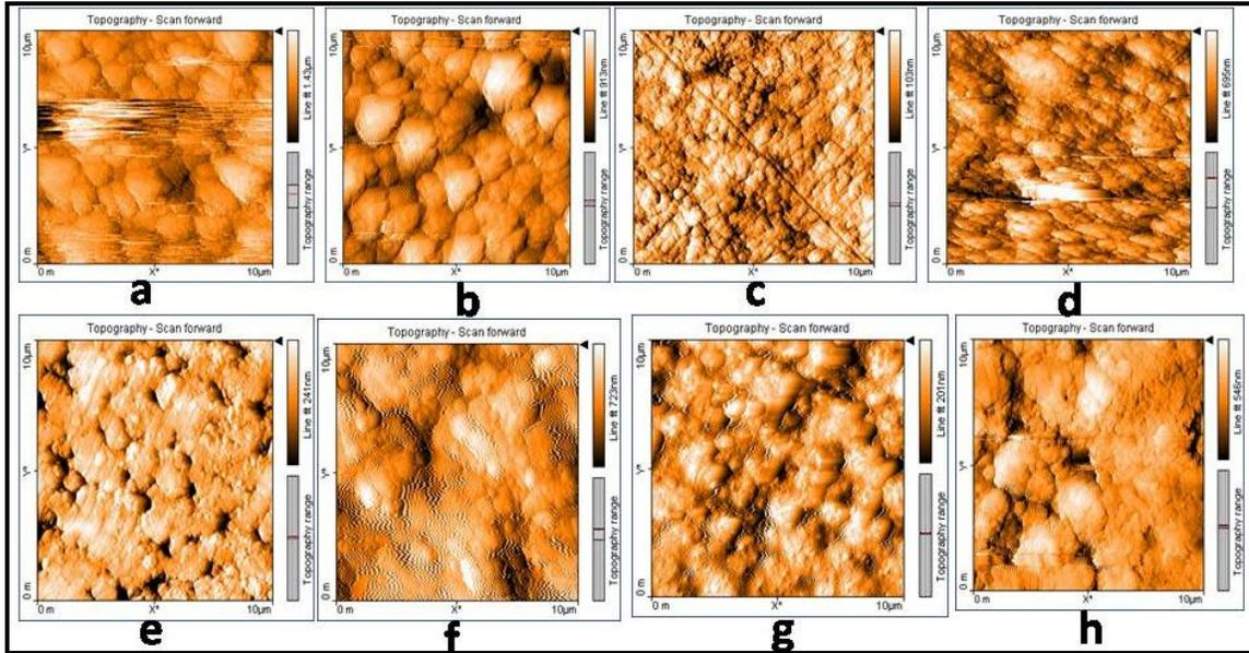
**Figure 4.7:** Morphological Images of plasma nitrided samples (a) En8, 10hours, (b) En8, 50hours, (c) En24, 10hours, (d) En24, 50hours, (e) En26, 10hours, (f) En26, 50hours, (g) En41b, 10hours, (h) En41b, 50hours.
