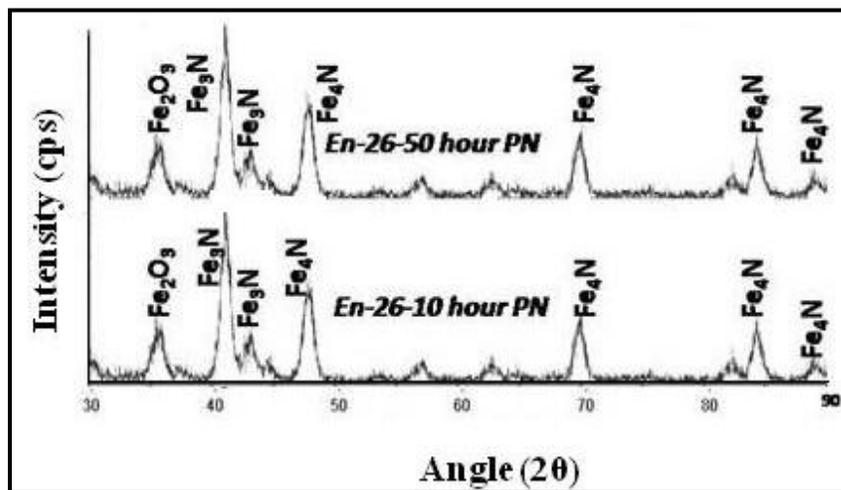
Figure 4.5: X-ray diffraction patterns of En26 steel samples for 10hours and 50hours.
