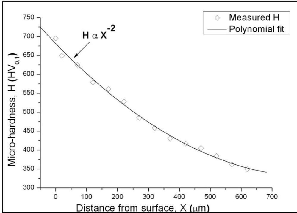
Figure 4.10: Polynomial fit of the micro-hardness profiles with diffusion depth.
