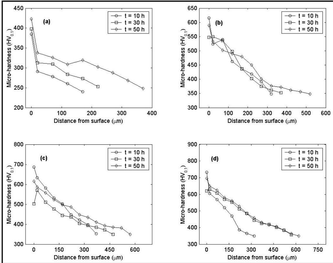
**Figure 4.9:** Variation of measured micro-hardness with diffusion depth (a) En8, (b) En24, (c) En26, (d) En41b.
