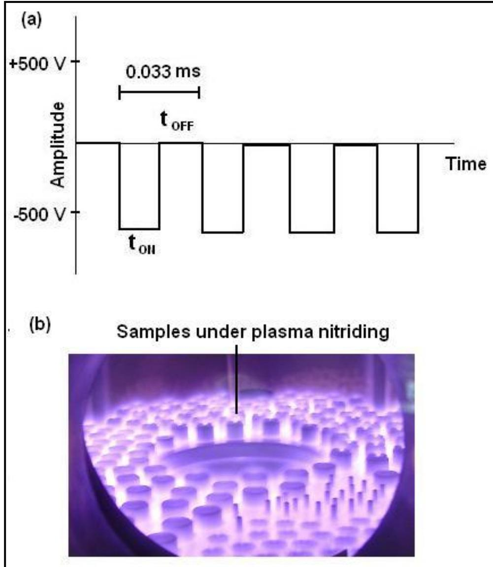
**Figure 4.1:** (a) Schematic representation of applied waveform, (b) Low alloy steel samples under plasma nitriding process.
