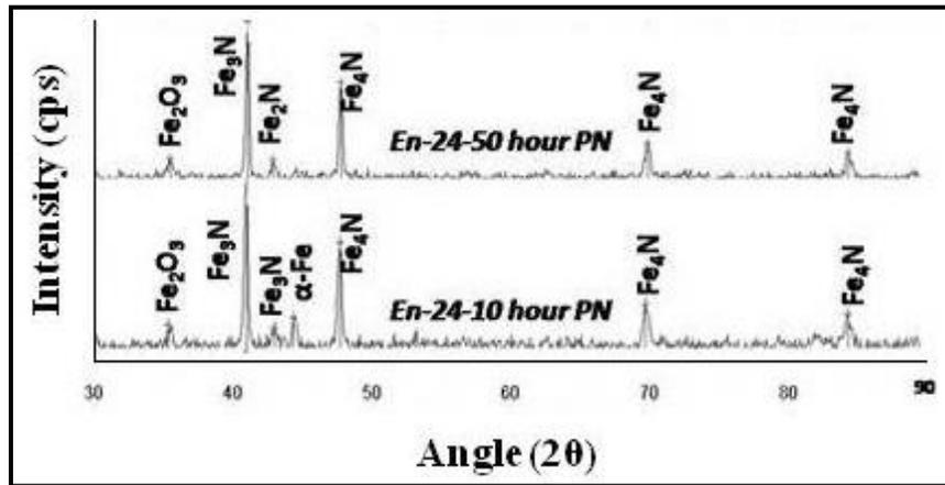
Figure 4.4: X-ray diffraction patterns of En24 steel samples for 10hours and 50hours.
