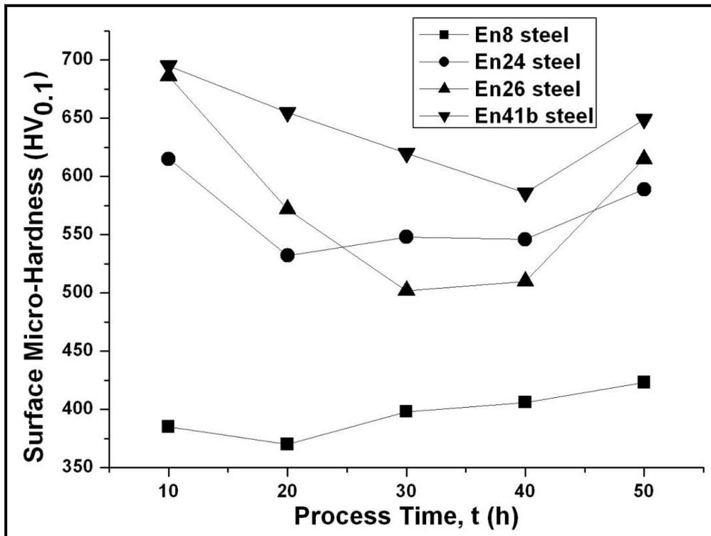
Figure 4.11: Surface micro-hardness profiles of plasma nitrided samples with variation of process time.
