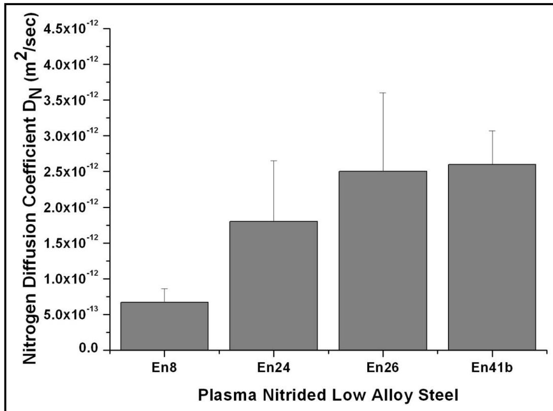
**Figure 4.12:** Values of nitrogen diffusion coefficient ( $D_N$ ) for each low alloy steel.
