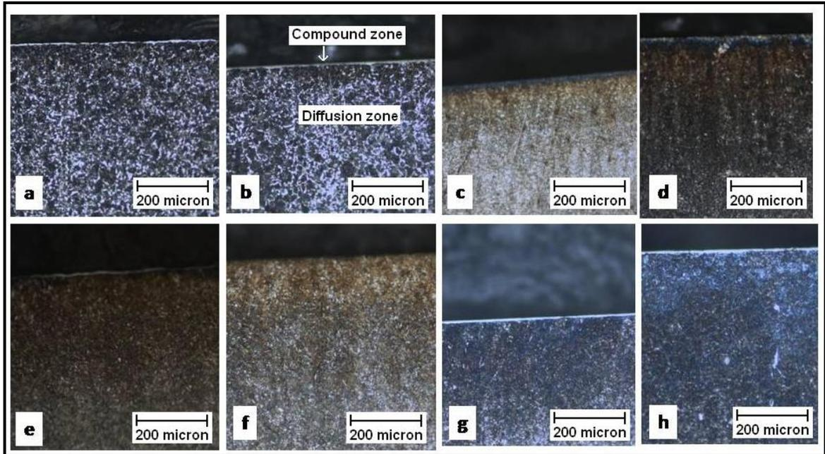
**Figure 4.2:** Microstructures of plasma nitrided samples (a) En8, 10hours, (b) En8, 50hours, (c) En24, 10hours, (d) En24, 50hours, (e) En26, 10hours, (f) En26, 50hours, (g) En41b, 10hours, (h) En41b, 50hours.
