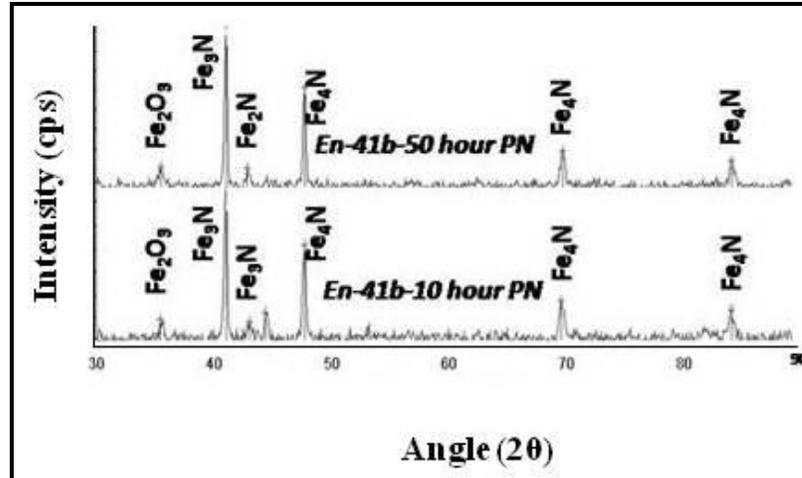
**Figure 4.6:** X-ray diffraction patterns of En41b steel samples for 10hours and 50hours.
