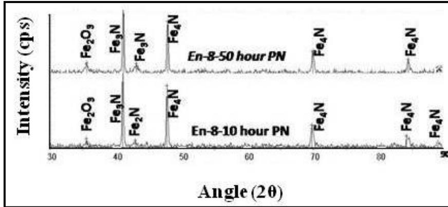
Figure 4.3: X-ray diffraction patterns of En8 steel samples for 10hours and 50hours.
