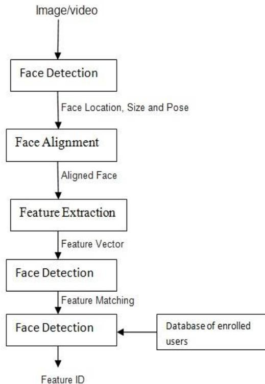
Fig 3.1: Face recognition processing flow
