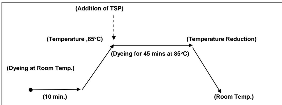
**Fig: 9. Dyeing of Cotton with Reactive dye**
