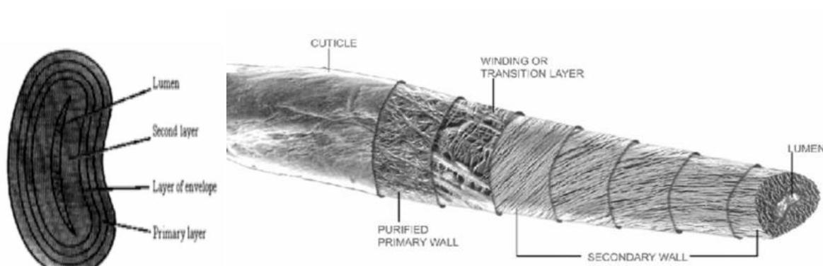
**Fig: 1. Structure of Cotton Fibre**
