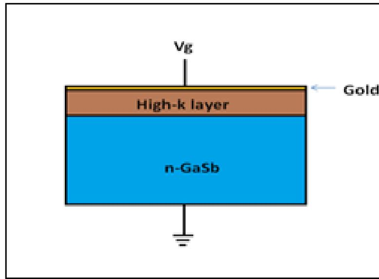
**Figure 6.1. Proposed structure of a MOSCAP without substrate passivation**
