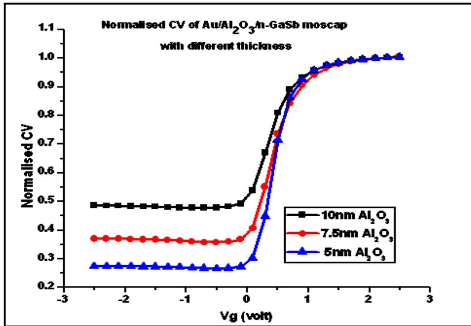
**Figure 6.3. Normalised CV Characteristics of Au/Al<sub>2</sub>O<sub>3</sub>/n-GaSb MOSCAP Structure for Different Thicknesses of Al<sub>2</sub>O<sub>3</sub>**
