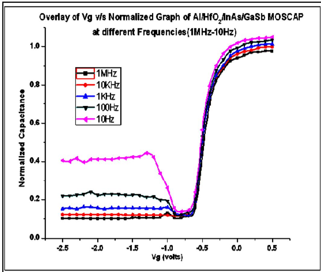
**Figure 6.8 Multi-frequency Capacitance-Voltage Characteristics of Au/HfO<sub>2</sub>/InAs/n-GaSb MOSCAP**
