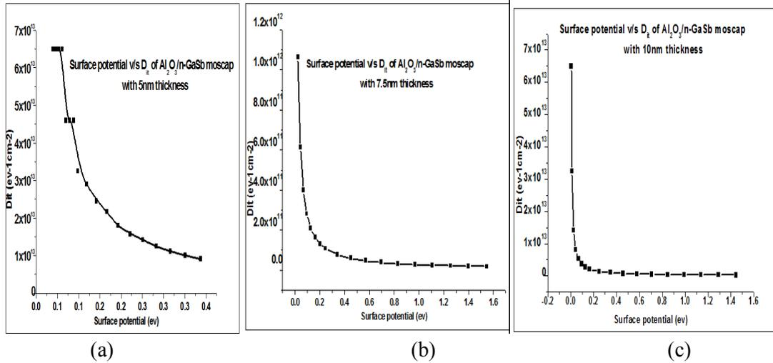
Figure 6.5. Surface Potential v/s  $D_{it}$  of Au/ $Al_2O_3$ /n-GaSb MOSCAP Structures for Different Thicknesses of  $Al_2O_3$  (a) 5nm (b) 7.5nm (c) 10nm
