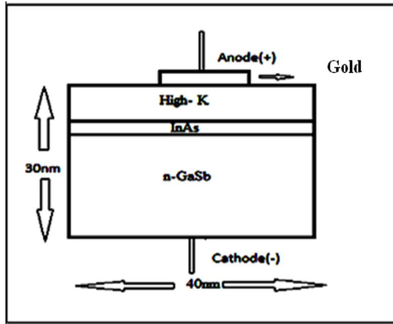
**Figure 6.2 Schematic Diagram and Sign Convention of the Proposed MOSCAP Structures with Surface Passivation Layer**
