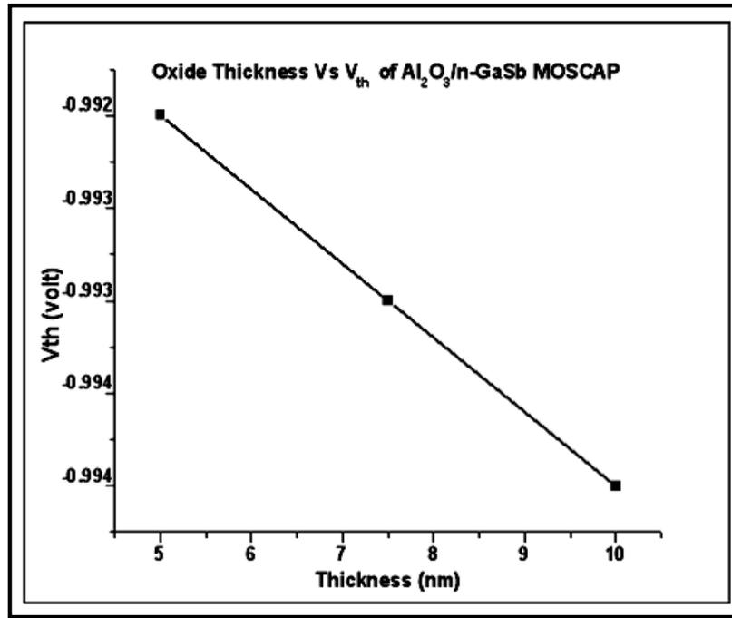
Figure 6.6(a).Oxide Thickness v/s  $V_{th}$  for Au/ $Al_2O_3$ /n-GaSb MOSCAP
