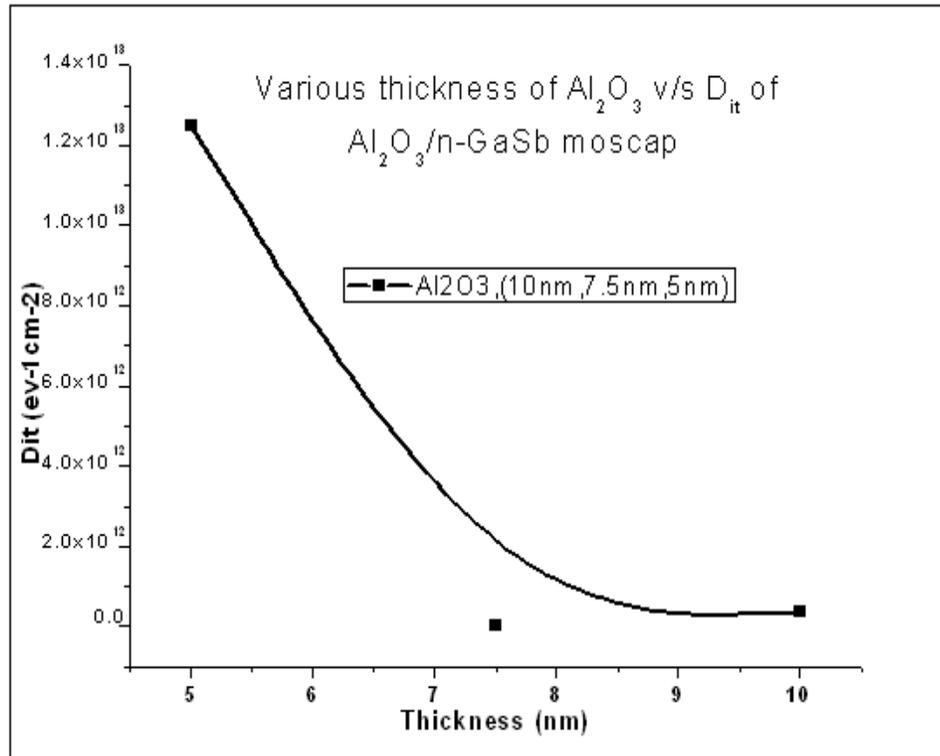
**Figure 6.4. Oxide Thickness v/s  $D_{it}$  of Au/ $\text{Al}_2\text{O}_3$ /n-GaSb MOSCAP Structure for Different Thicknesses of  $\text{Al}_2\text{O}_3$**
