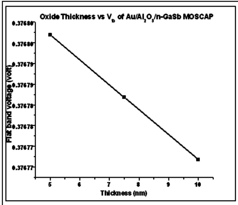
Figure 6.6(b) Oxide Thickness vs  $V_{fb}$  for Au/Al<sub>2</sub>O<sub>3</sub>/n-GaSb MOSCAP
