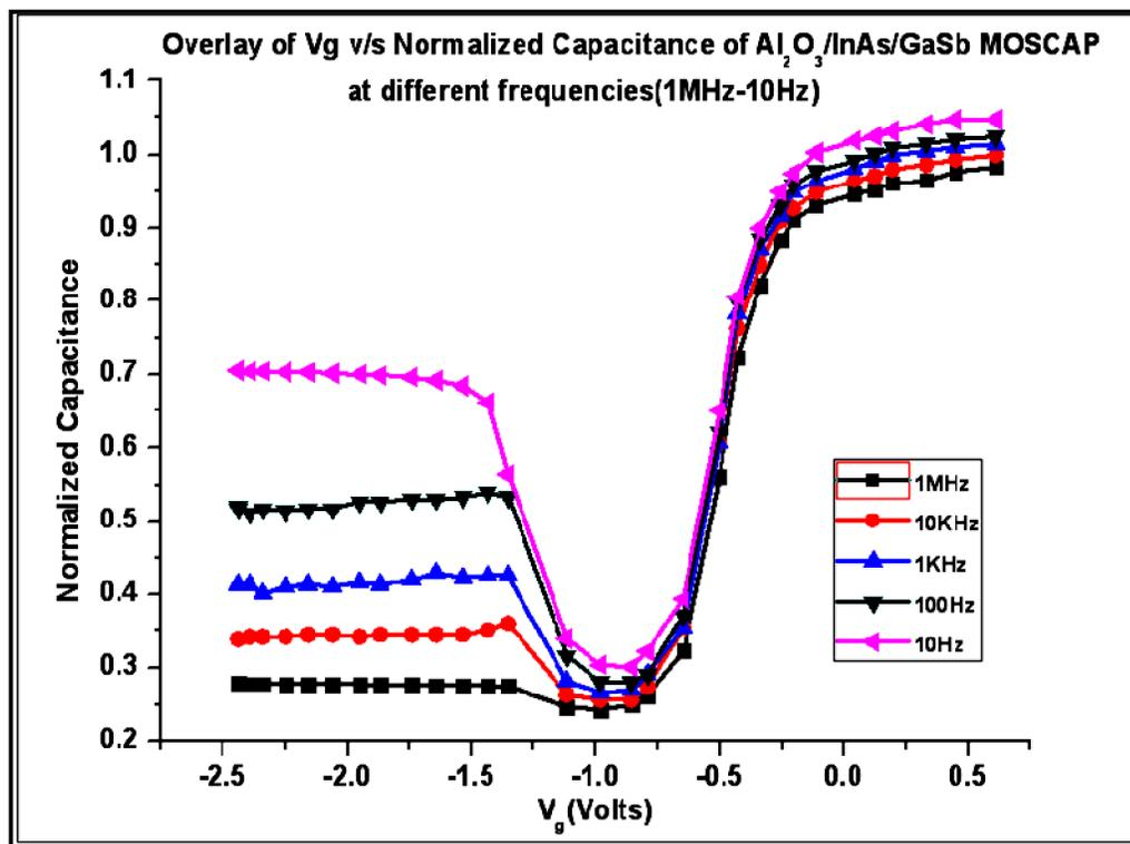
**Figure 6.7 Multi-frequency Capacitance-Voltage Characteristics of Au/ $Al_2O_3$ /InAs/n-GaSb MOSCAPs**
