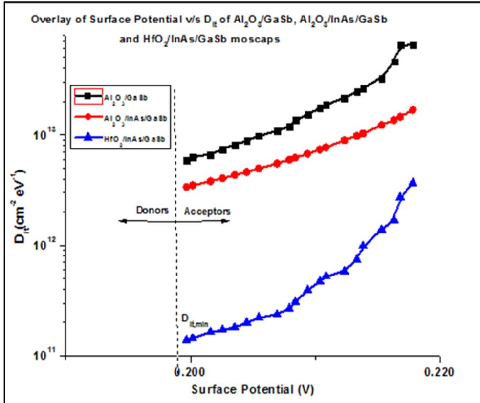
**Figure 6.9 Interface Trap Distribution for  $\text{Al}_2\text{O}_3/\text{n-GaSb}$  ,  $\text{Al}_2\text{O}_3/\text{InAs}/\text{n-GaSb}$  and  $\text{HfO}_2/\text{InAs}/\text{n-GaSb}$  MOSCAP Structures**
