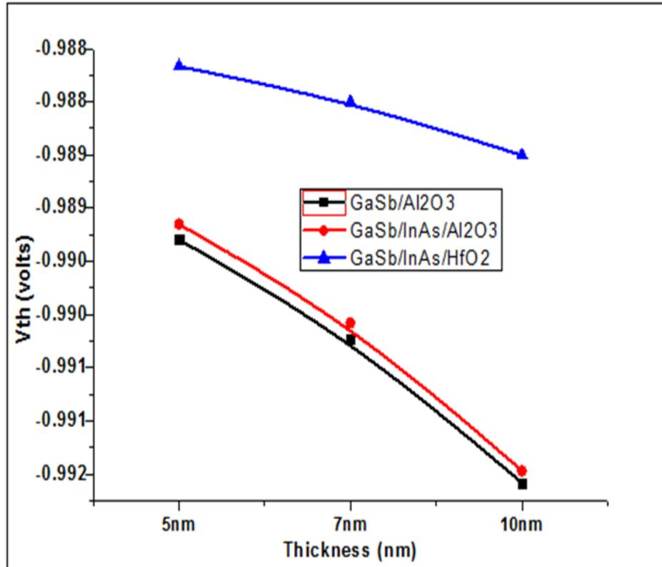
**Figure 6.10 Oxide Thickness v/s Threshold Voltage of  $\text{Al}_2\text{O}_3/\text{GaSb}$ ,  $\text{Al}_2\text{O}_3/\text{InAs}/\text{GaSb}$  and  $\text{HfO}_2/\text{InAs}/\text{GaSb}$  MOSCAPS**
