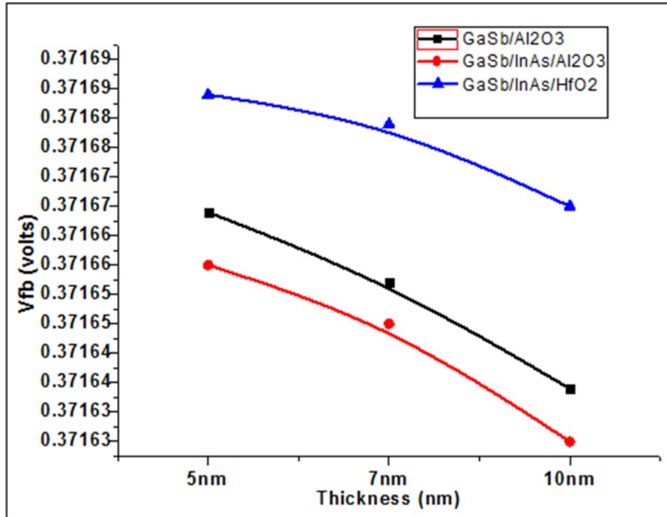
**Figure 6.11 Oxide Thickness v/s FlatBand Voltage of Al<sub>2</sub>O<sub>3</sub>/GaSb, Al<sub>2</sub>O<sub>3</sub>/InAs/ GaSb and HfO<sub>2</sub>/InAs/ GaSb MOSCAPs**
