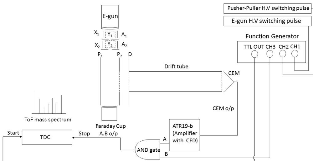
**Figure 6.1:** DEToF experimental schematic (first acceleration region: region between  $P_1$  and  $P_2$ , second acceleration region: region between  $P_2$  and  $D$ )
