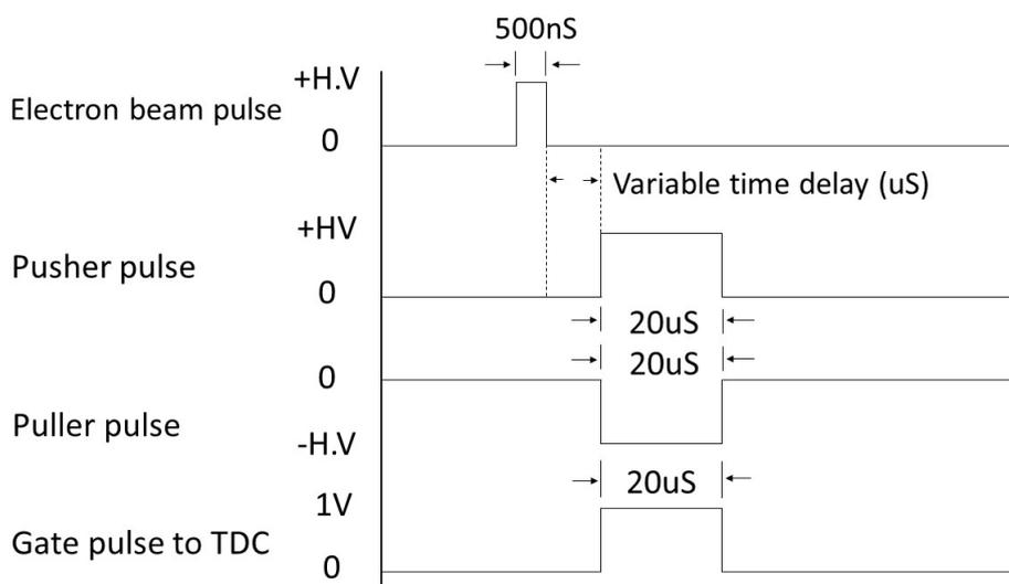
**Figure 6.2:** Pulsing sequence for DEToF
