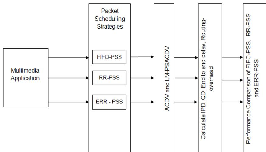
**Figure 5.1: Flow Diagram for performance comparison of Packet Scheduling Strategies over Multimedia Applications**
