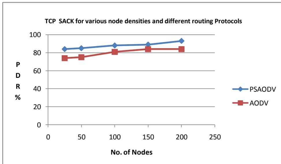
**Figure 3.3: PSAODV - Effect of Packet Delivery Ratio on varying node density using TCP-SACK**
