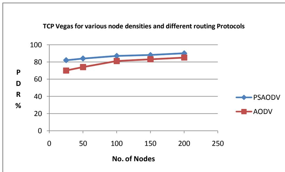
**Figure 3.1: PSAODV - Effect of Packet Delivery Ratio on varying node density using TCP-Vegas**
