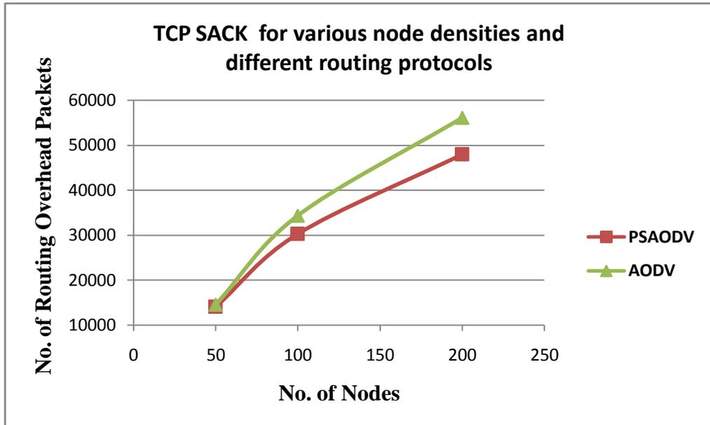
**Figure 3.4: PSAODV - Effect of Routing overhead on varying node density using TCP-SACK**
