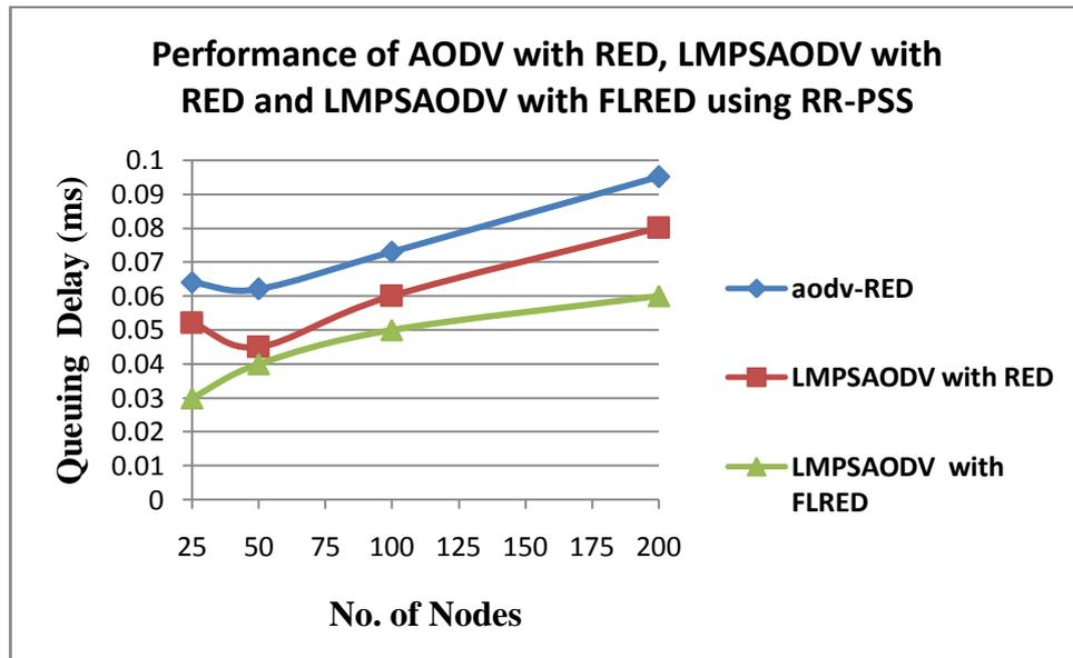
**Figure 6.2: FL-RED Effect of Queuing Delay on varying node density using different Routing Protocols and Queue Management Techniques**
