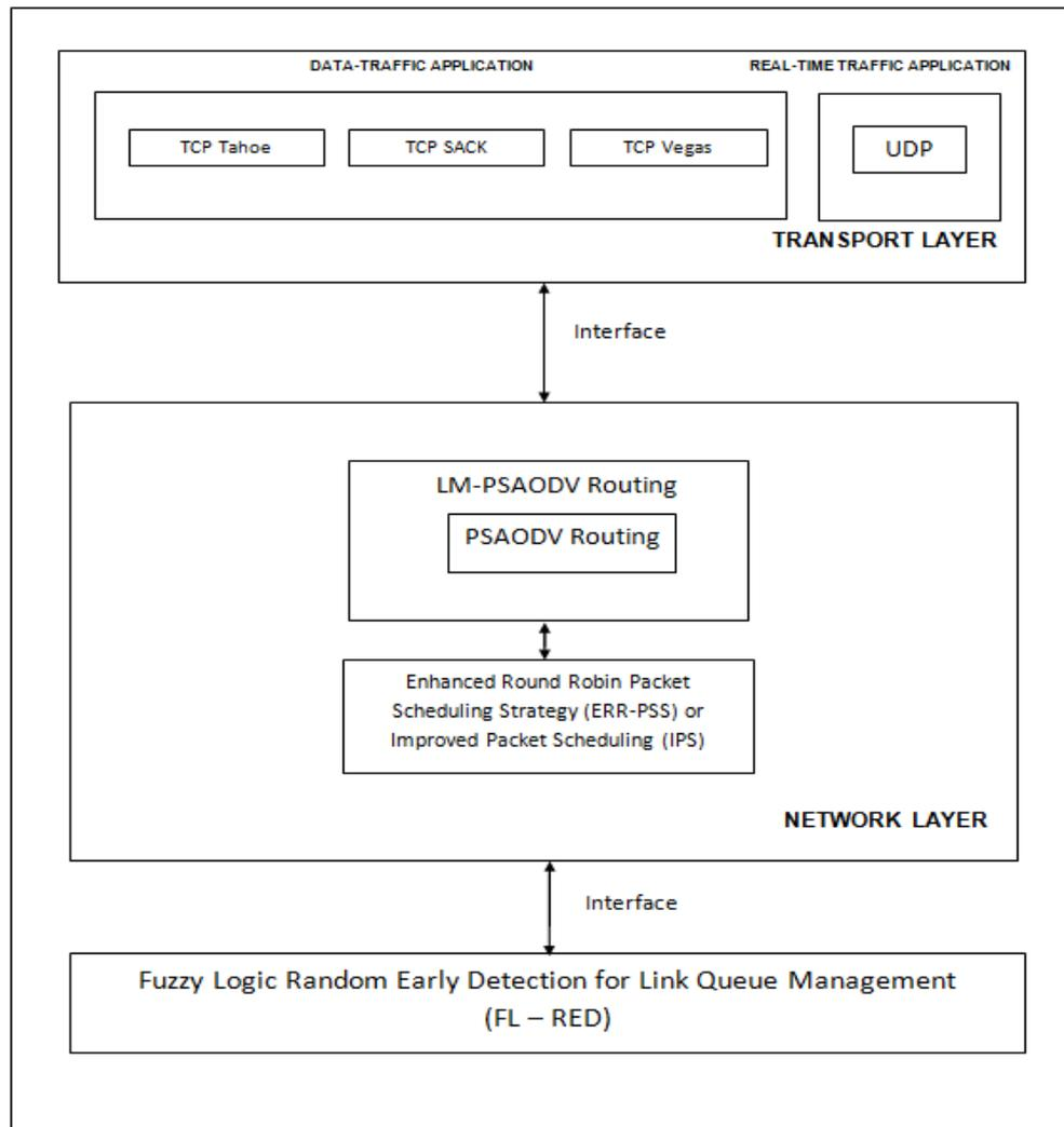
**Figure 6.3: Integrated Routing and Queue Management framework**
