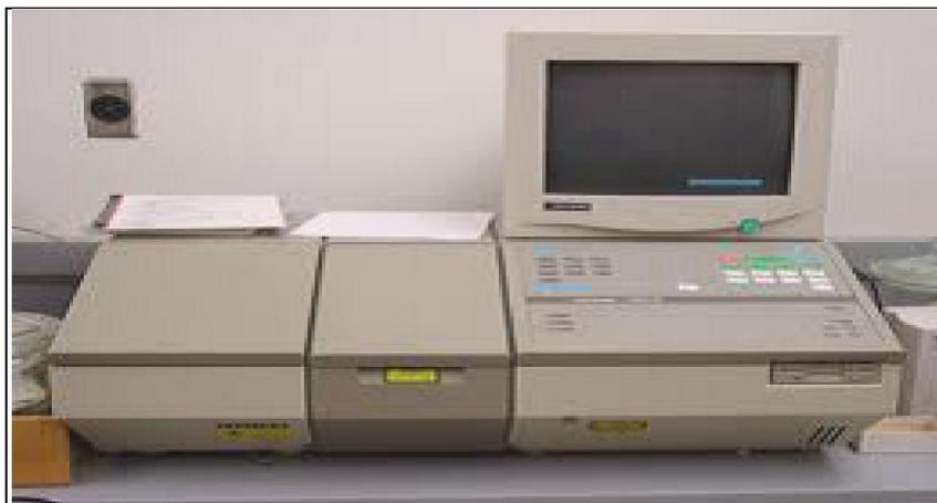
**Fig 1.13: Schematic diagram of IR spectrophotometer**
