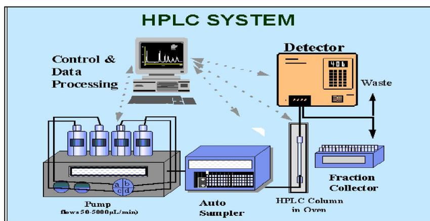
**Fig 1.10: Schematic diagram of an HPLC instrument**
