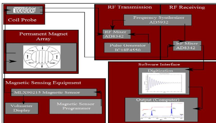
**Fig 1.14: Schematic diagram of NMR spectrophotometer**
