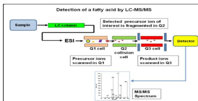
**Fig 1.11: Schematic representation of LC-MS instrument**
