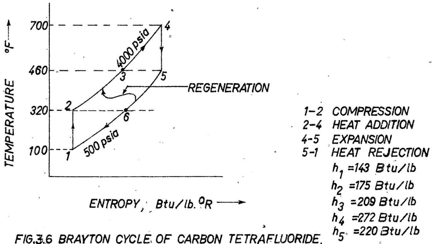
FIG.3.6 BRAYTON CYCLE OF CARBON TETRAFLUORIDE.
