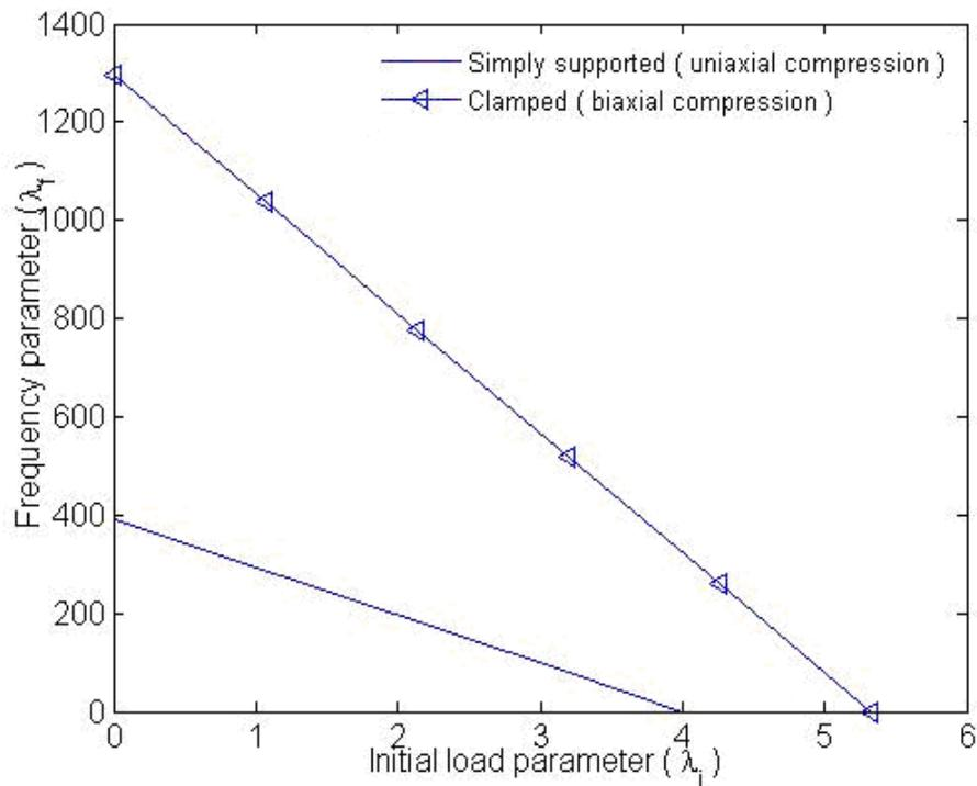
**Fig. 4.10 Thin square plate with simply supported under uniaxial compression and clamped square plate under biaxial Compression**
