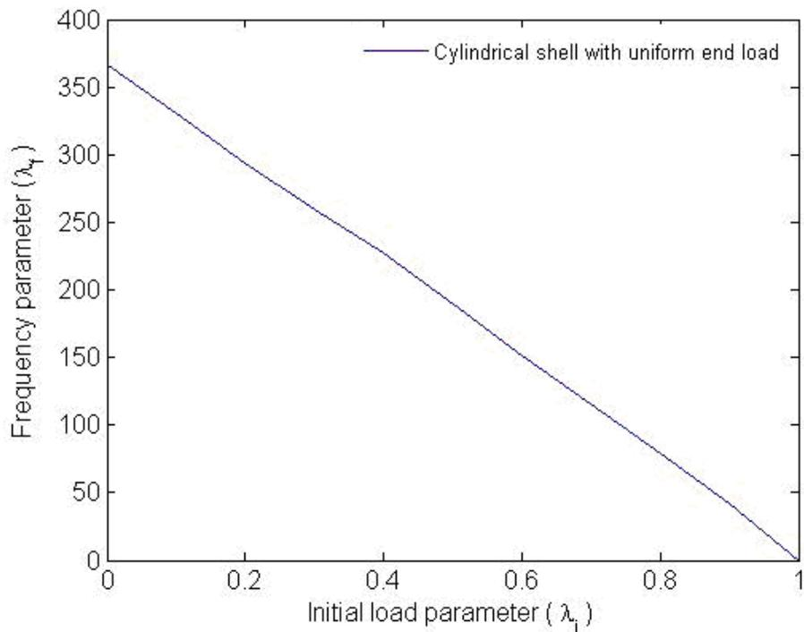
**Fig. 4.11 Layered cylindrical shell with delamination under uniform end load**
