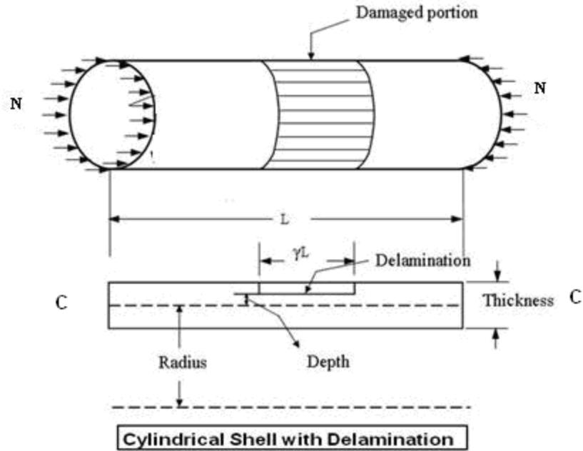
**Fig. 4.5 Layered cylindrical shell with delamination under uniform end load**
