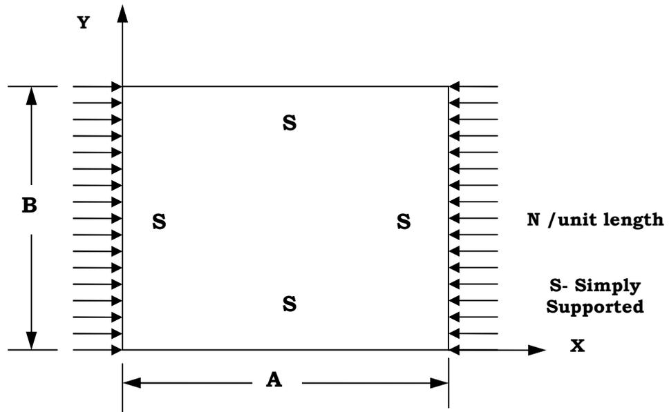
**Fig. 4.4a Thin simply supported square plate under uniaxial compression**
