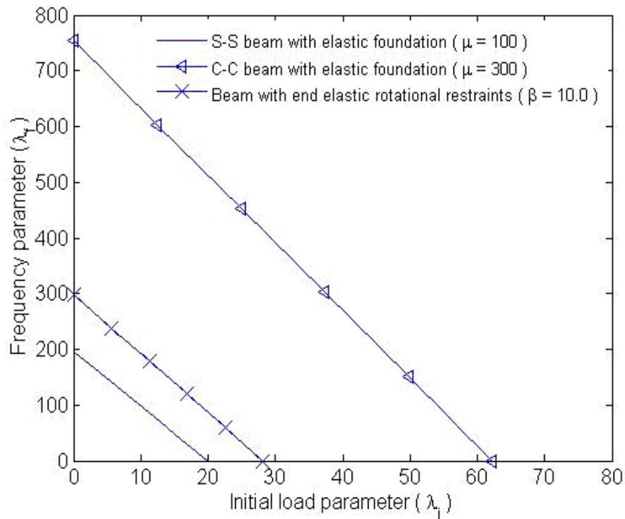
**Fig. 4.6 Slender uniform beams with elastic foundation and elastically restrained against rotation**
