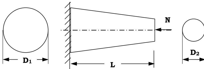
**Fig.4.2a Short tapered cantilever beam of circular cross-section**
