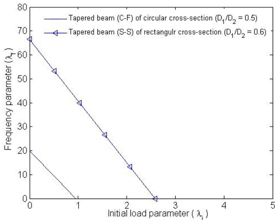
**Fig. 4.7 Short tapered beams of circular (clamped-fixed) and rectangular cross-section (simply supported)**
