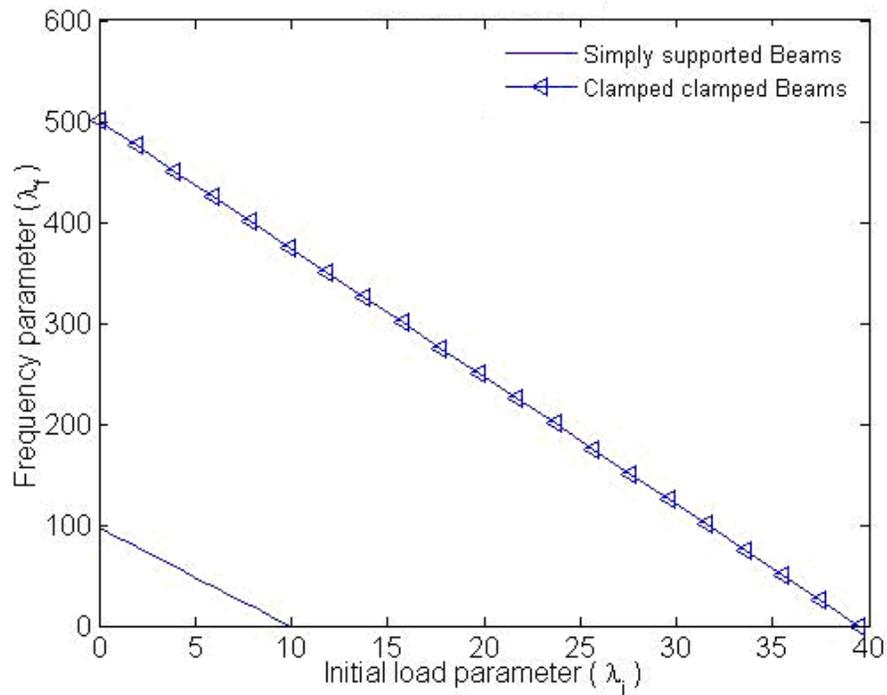
**Fig. 4.8 Composite beams with simply supported (S-S) and clamped-clamped (C-C) end conditions**
