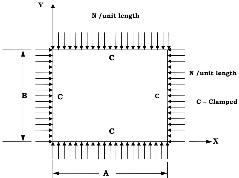
**Fig. 4.4b Thin clamped square plate under biaxial compression**
