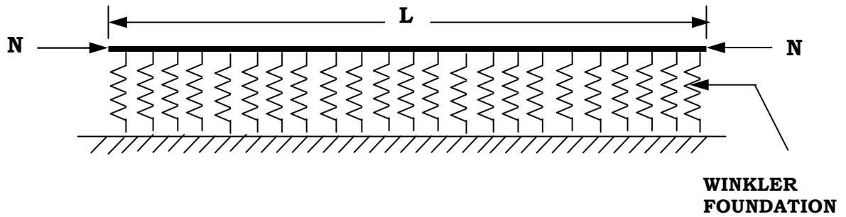
**Fig. 4.1a Uniform isotropic beam on elastic foundation**
