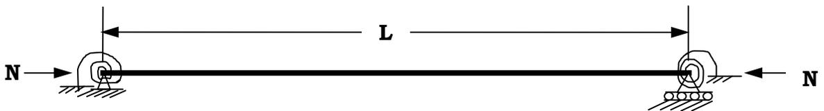
**Fig. 4.1b Uniform isotropic beam with elastically restrained ends against rotation**
