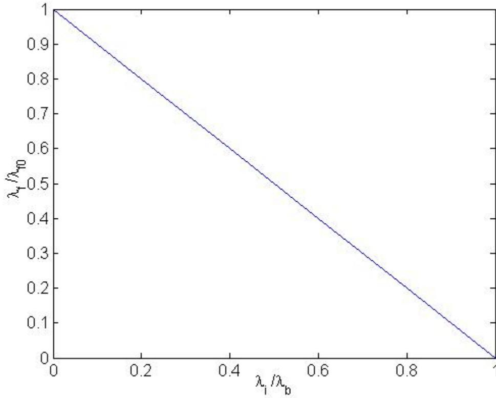
**Fig. 4.12 Universal curve for initially loaded structural member**
