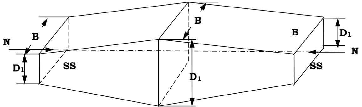
**Fig. 4.2b Short symmetrically tapered simply supported (SS) beam of rectangular Cross - Section**
