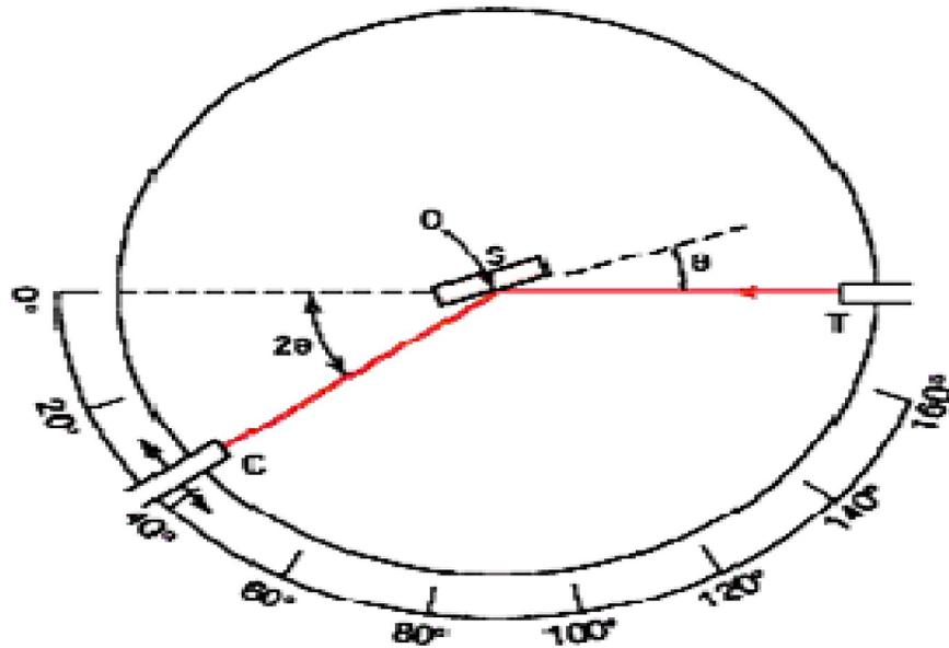
**Figure 4.3: Schematic diagram of an X-ray diffractometer; T is the X-ray source, S the specimen, C the detector and O the axis around which the specimen and detector rotate.**
