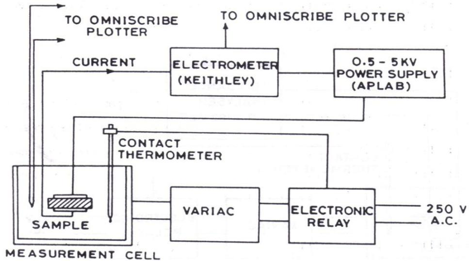
Figure 4.8: A set up to study conductivity of the samples.
