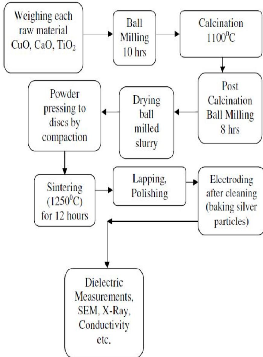
**Figure-4.1: The mixed oxide route of CCTO ceramic preparation**
