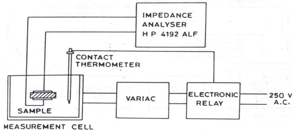
**Figure 4.7: The schematic diagram of the set up used for measuring the dielectric constant**
