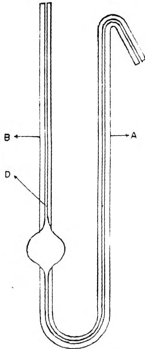
Fig. 2.3- Bicapillary pycnometer
