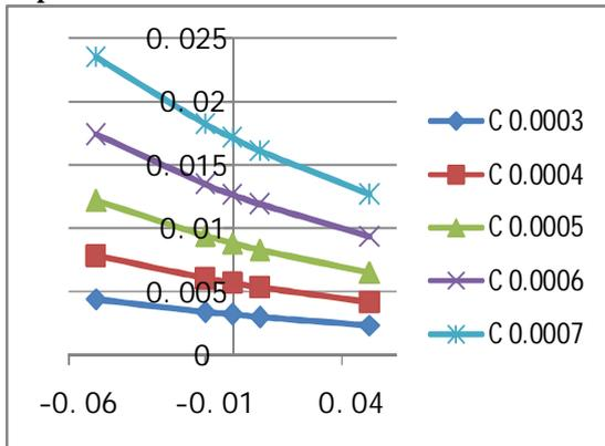
**Figure: 8** Variation of Load carrying capacity with respect to  $\alpha$  for various values of B/L.
