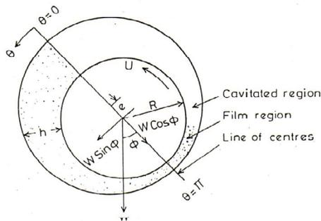
Figure :1 Configuration of bearing system.
