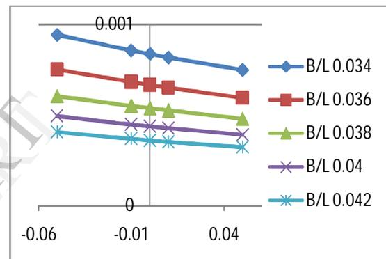
The effect of skewness presented in figures (2) to (5) indicate that the load carrying capacity decreases as positive skewness increases while negatively skewed roughness increases the load carrying capacity. The positive effect of the negatively skewed roughness is relatively more in the case of standard deviation, while there is a nominal adverse effect registered by standard deviation.
