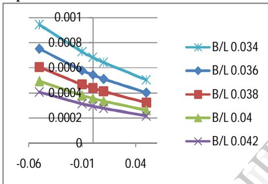
The effect of variance on LCC is given in figures (6) to (8). It is interesting to note that variance follows the path of the skewness so far as the LCC is concerned. Accordingly the positive effect of negative variance gets enhanced by negatively skewed roughness.
