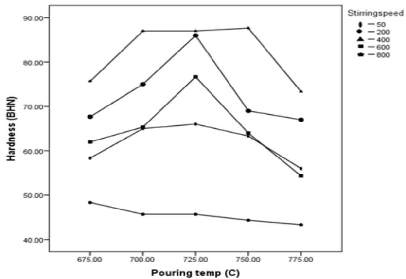
**Figure 5.8 Pouring Temperature Vs Hardness Graph**
