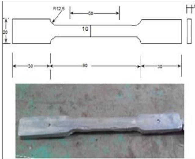
**Figure 5.3 Specimen of Tensile Test**
