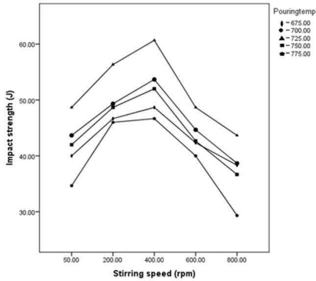
**Figure 5.9 Stirring Speed Vs Impact Strength Graph**
