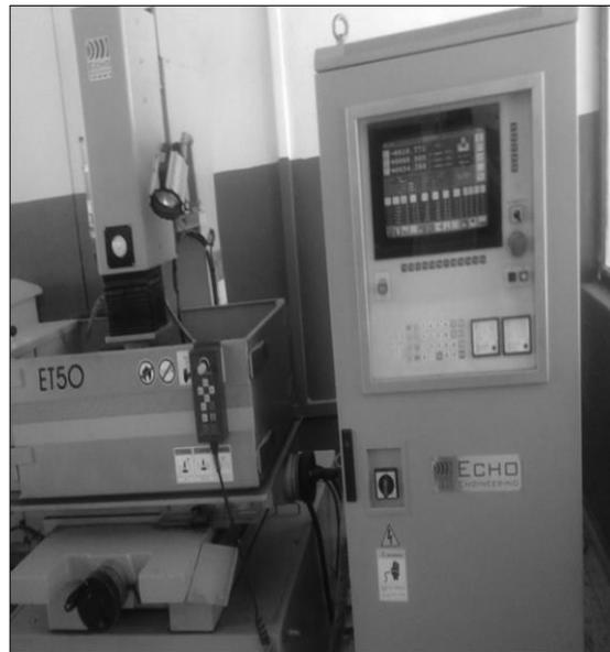
**Figure 5.4 Electro discharge Machining.**
