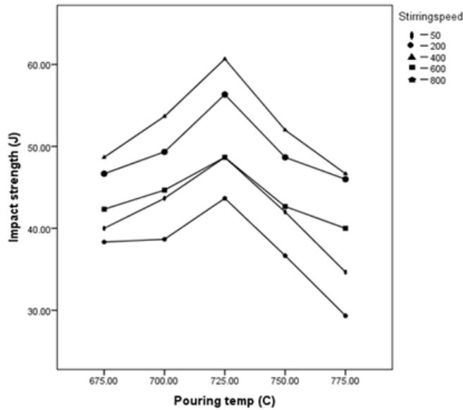
**Figure 5.10 Pouring Temperature Vs Impact Strength Graph**
