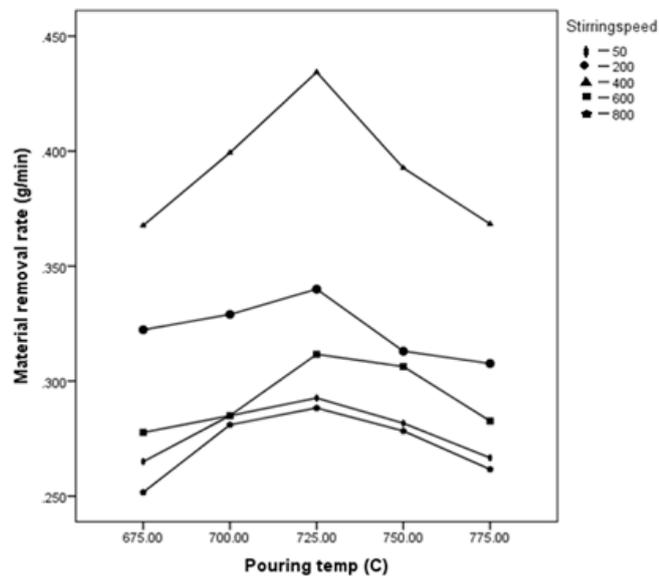
**Figure 5.12 Pouring Temperature Vs Material Removal Rate Graph**
