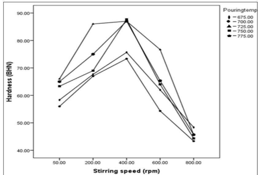
**Figure 5.7 String Speed Vs Hardness Graph**
