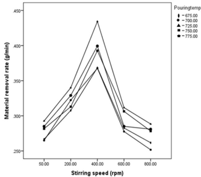
**Figure 5.11 Stirring Speed Vs Material Removal Rate Graph**
