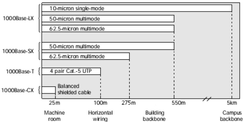
Figure 2.2.4 Gigabit Ethernet application environments and link distances [89]
