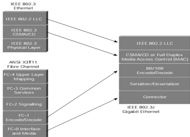
Figure 2.2.5 Gigabit Ethernet Protocol Stack [90]
