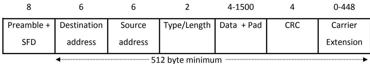
Figure 2.2.2 Gigabit Ethernet Frame Structure with Carrier Extension
