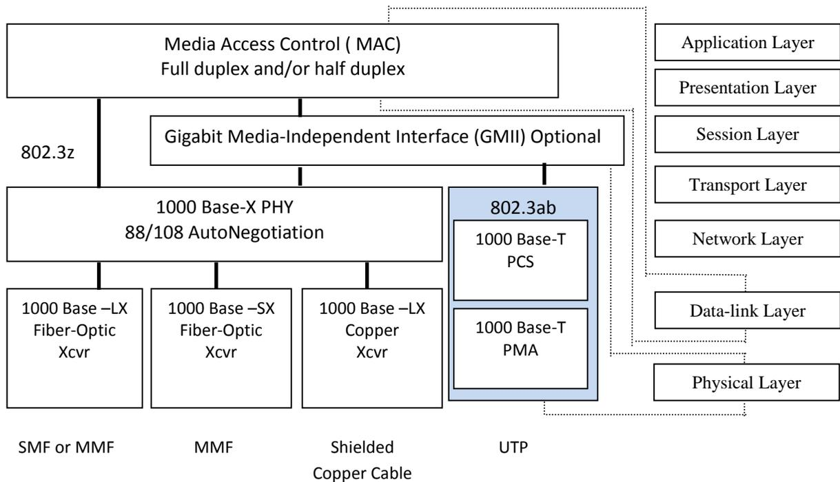
Figure 2.2.1 Gigabit Ethernet layer diagram [89]
