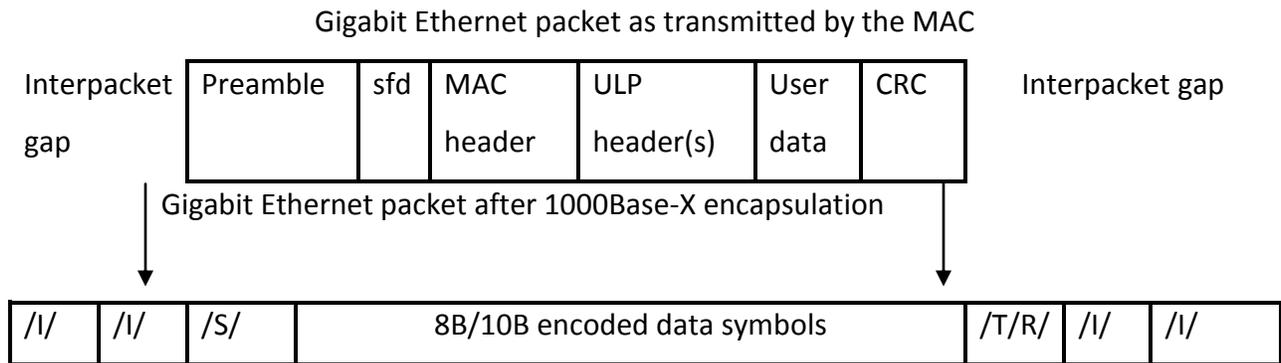
Figure 2.2.3 1000Base-X encapsulation
