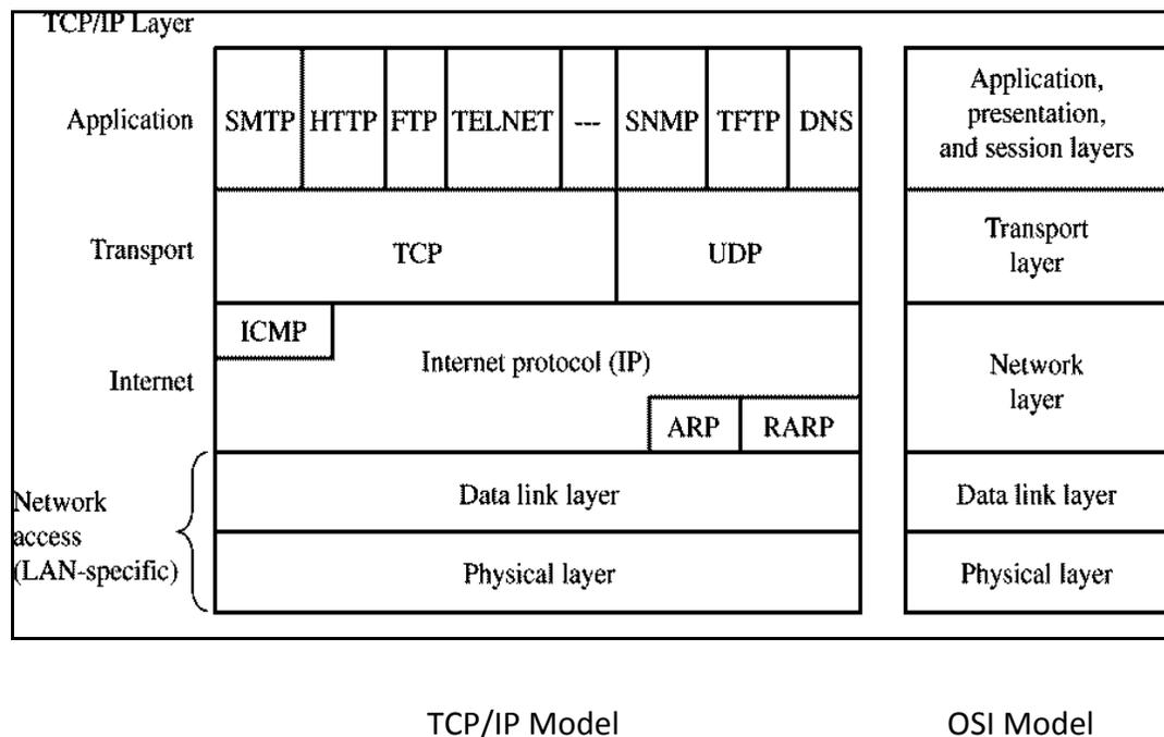
Figure 1.3.1 Comparison of TCP/IP and OSI models [3]
