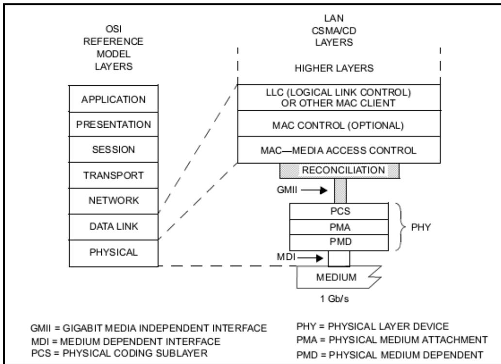
Figure 1.6.3 Gigabit Ethernet protocol architecture [12]
