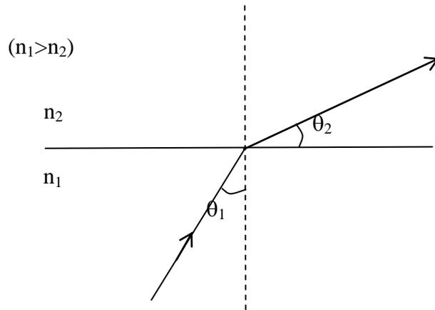
**Figure 1.12: Refraction of light at an interface of two media**
