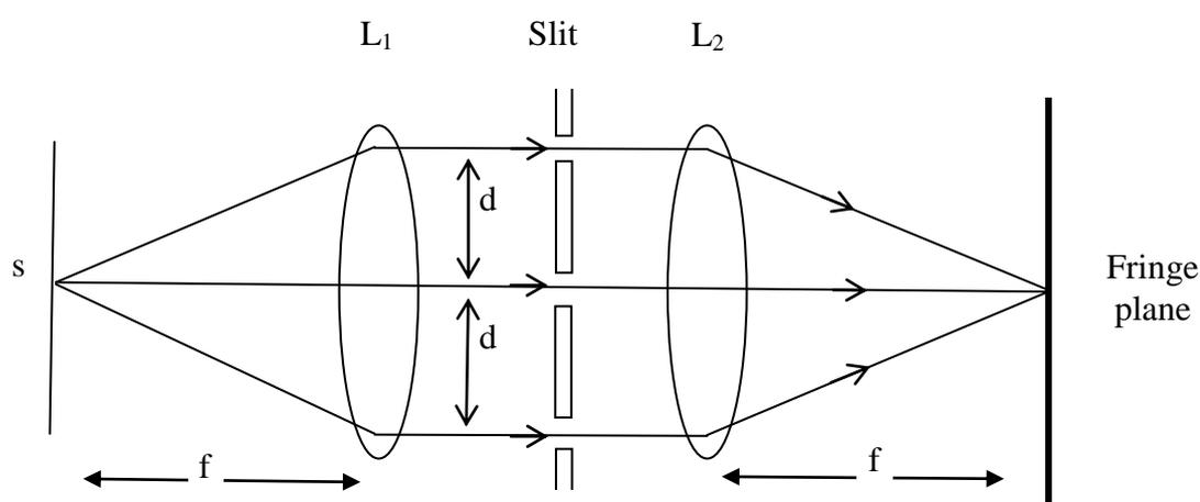
**Figure 1.10: Zernike's Three Beam Interferometer**
