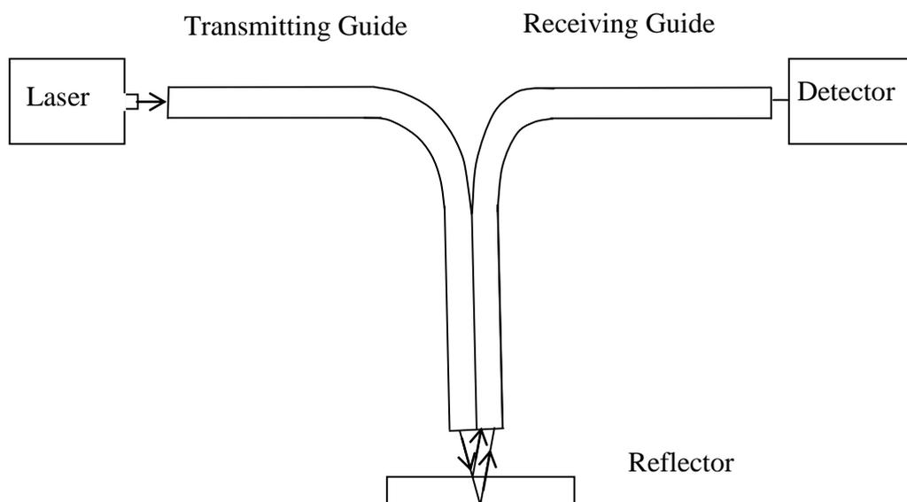
**Figure 1.15: Basic diagram of a Y-Guide**
