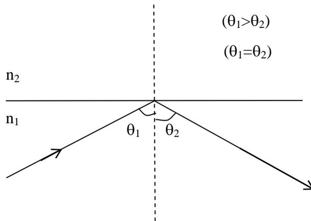
**Figure 1.13: Total internal reflection of light**
