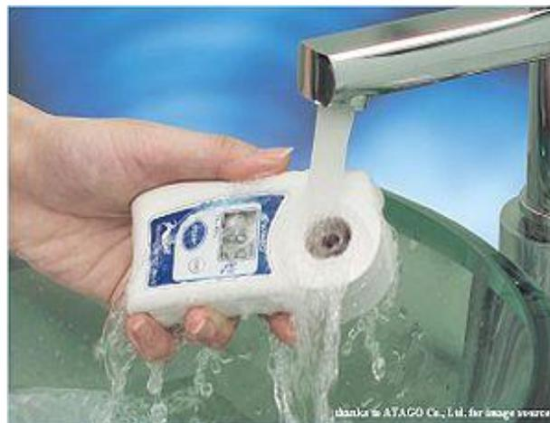
**Figure 1.3: A Modern Digital Handheld Refractometer**
