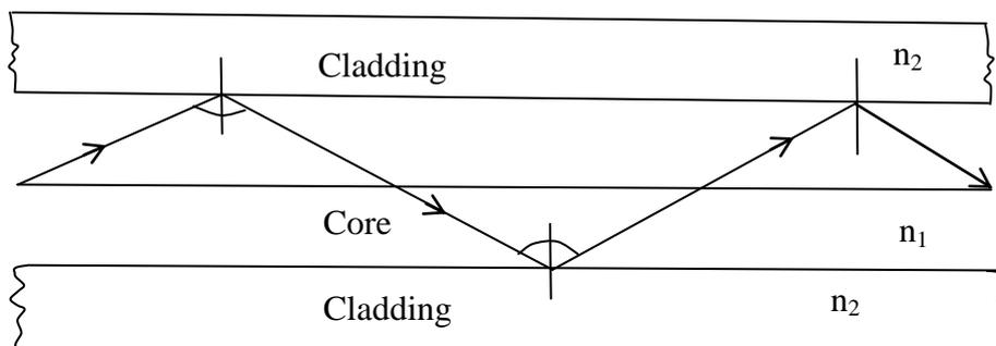
**Figure 1.14: Transmission of an optical ray through an optical fiber**
