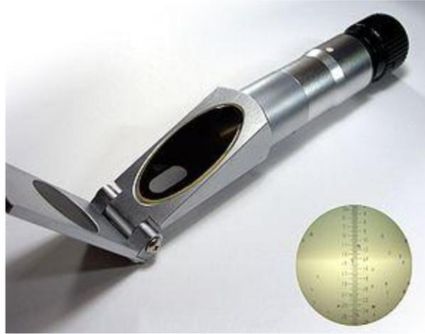
**Figure 1.2: Handheld Refractometer**
