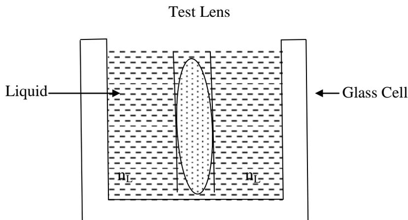
**Figure 1.5: Actual lens arrangement used for experimental investigation**
