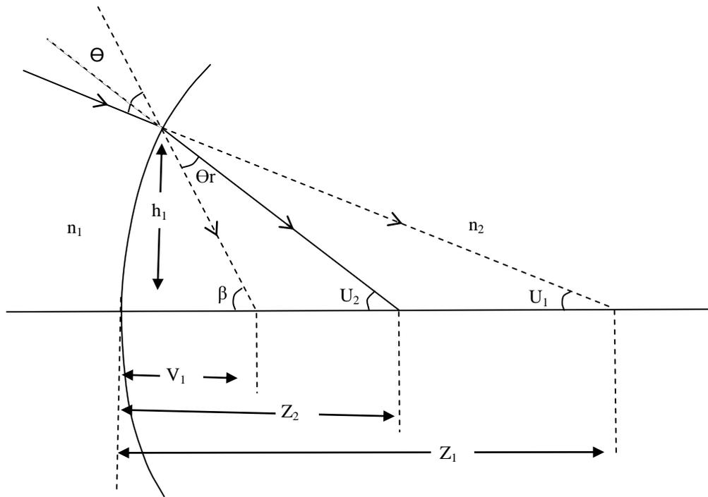
**Figure 1.6 Ray-Tracing Scheme for a single curved surface**
