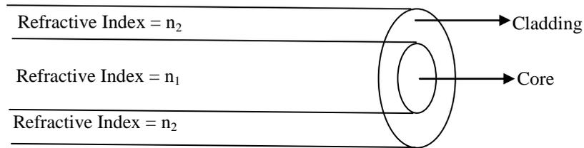
**Figure 1.11 Typical Optical Fiber Geometry**
