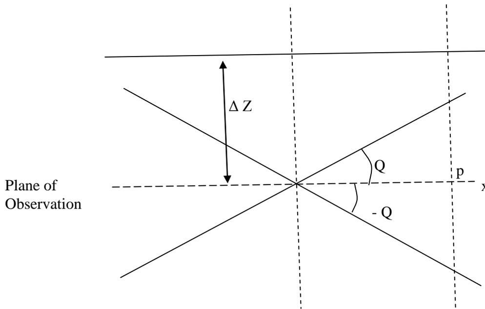
**Figure 1.8: Formation of three beam fringes**
