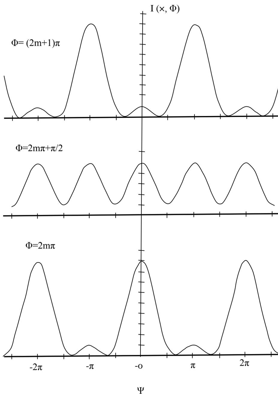
**Figure 1.9: Intensity distribution in three beam fringes for different value of  $\phi$ , the phase difference between the third beam and the other two beams.**
