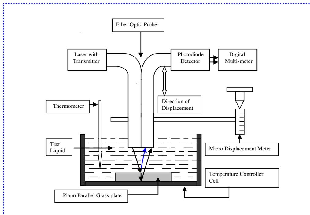
**Figure 5.2: Schematic experimental set-up of the Y-Guide refractometer**
