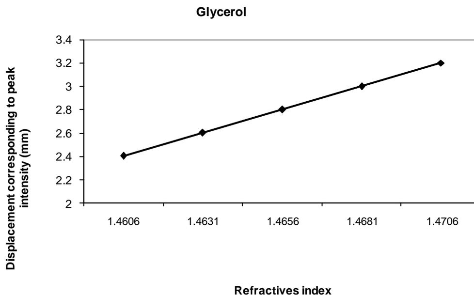
**Figure 5.13: Variation of displacement corresponding to peak intensity with refractive index of glycerol.**
