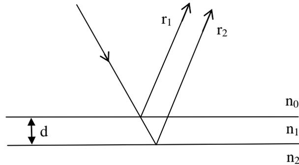
**Figure 5.1 reflection of light in Plano parallel glass plate**
